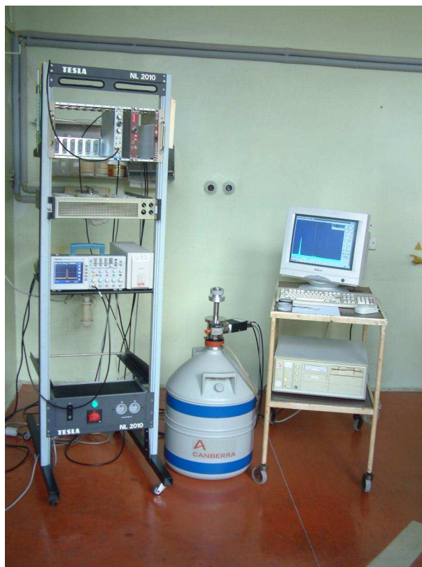
Figure 106: The \gamma -spectrometer with a Si(Li) detector.
