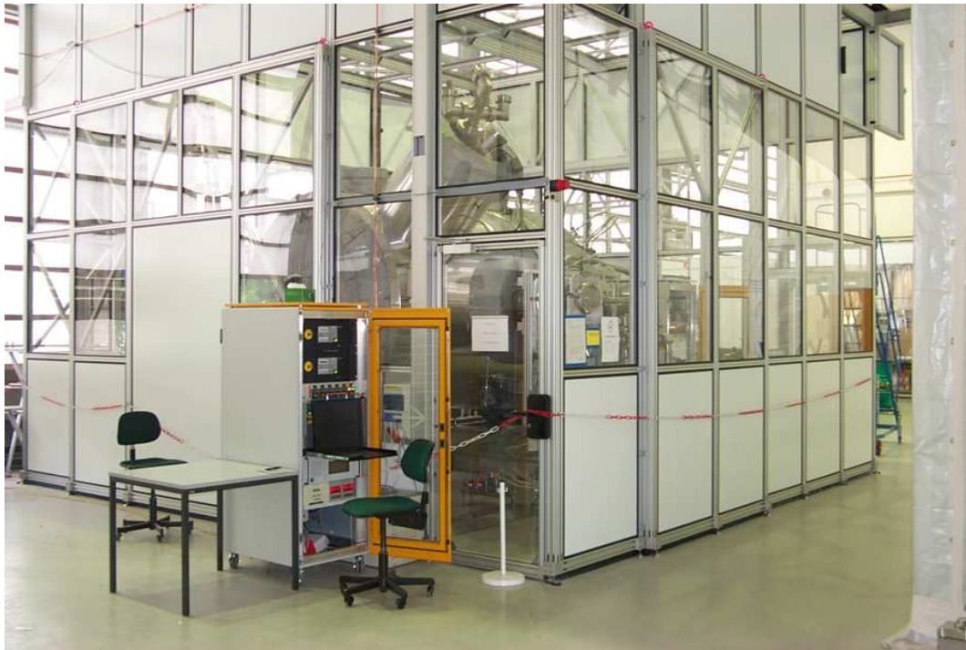
Figure 66: The dry-air compartment around the KATRIN pre-spectrometer.
