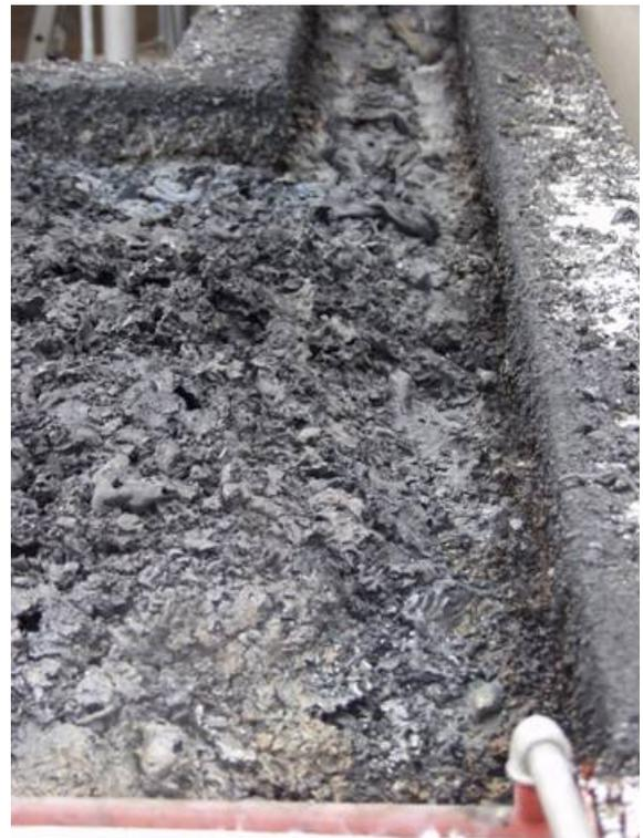
**Figure 3-14**: Anchored melt crust at the sidewalls
