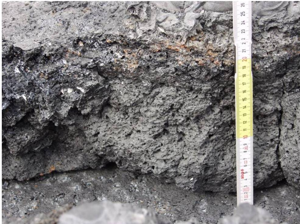
**Figure 3-26:** Left side of the solidified oxide melt in the trench, 1.4 m from the front side.
