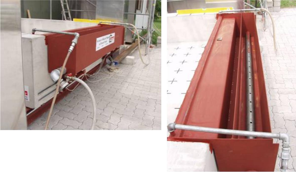
**Figure 2-7:** Water distribution tank of 200 liters mounted at the opposite wall of the cavity
