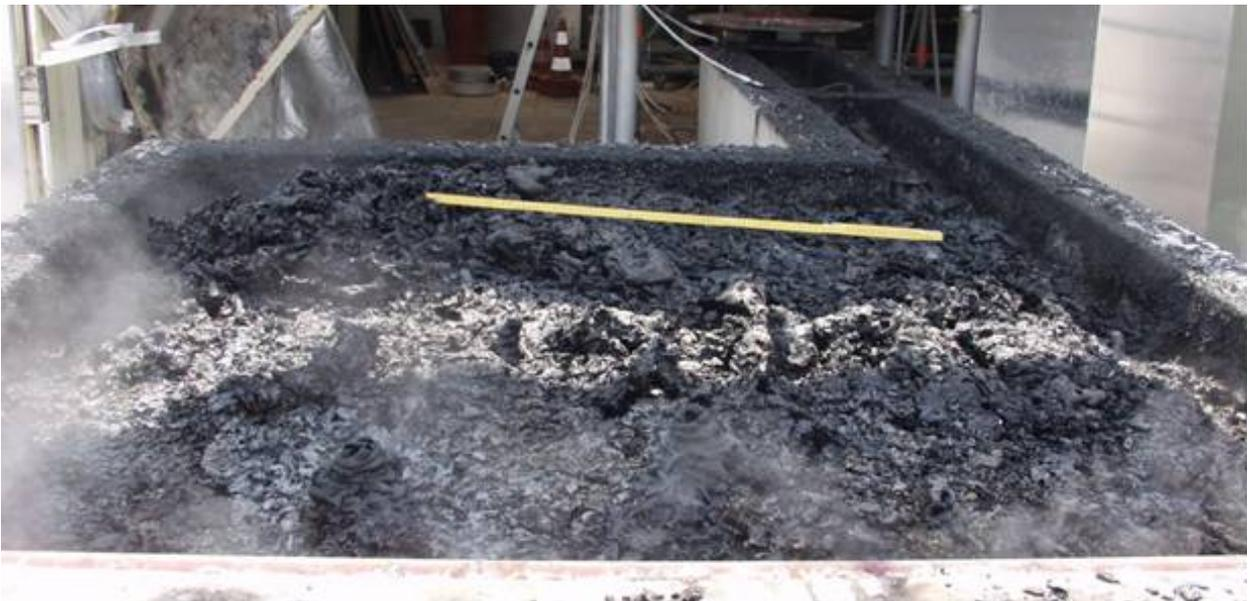
**Figure 3-11:** Surface of the solidified melt. View from the weir after 3 hours
