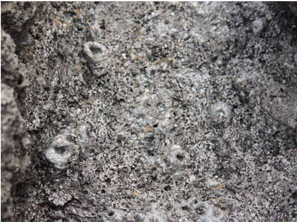
**Figure 3-28:** Structure of the metal plate at the bottom of the melt
