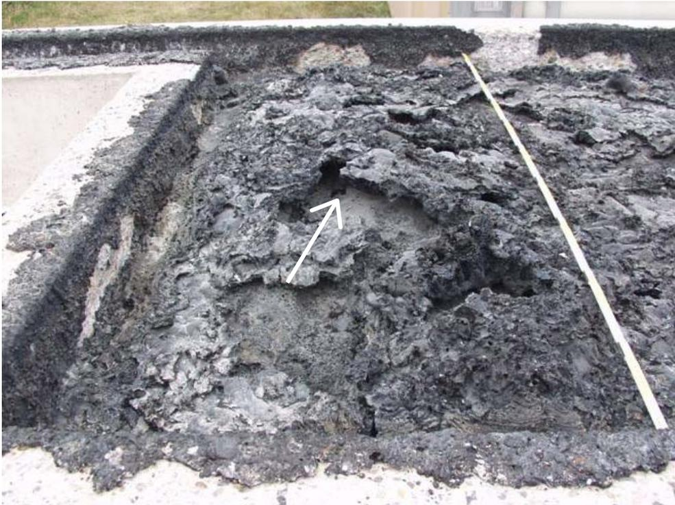
**Figure 3-20:** Melt surface at the highest elevation after removing the upper layer
