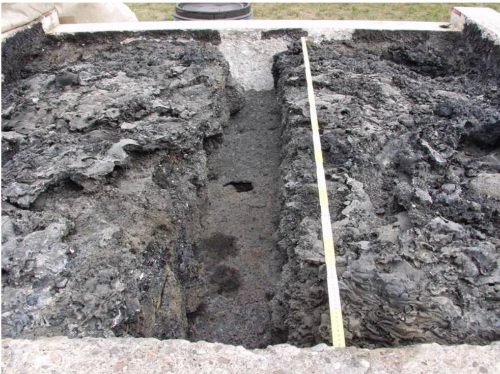
**Figure 3-23:** Trench through the melt to investigate the melt constitution, opposite wall in the background, from which the weir is removed
