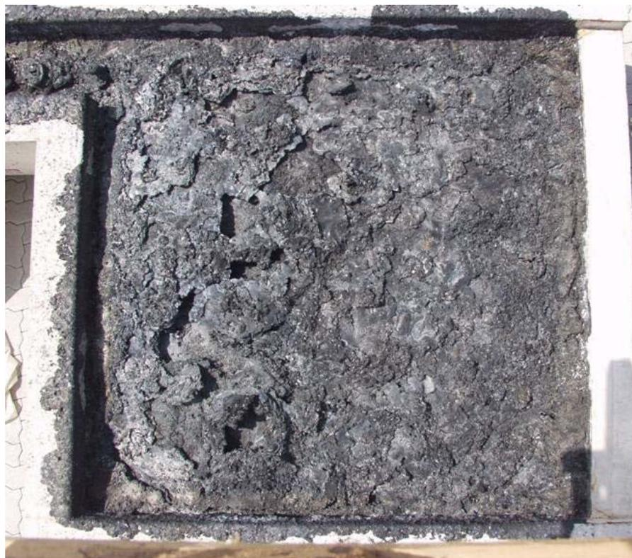
**Figure 3-19:** Melt surface after removing the upper crashed layer
