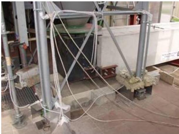
Thermite crucible with load cells,
