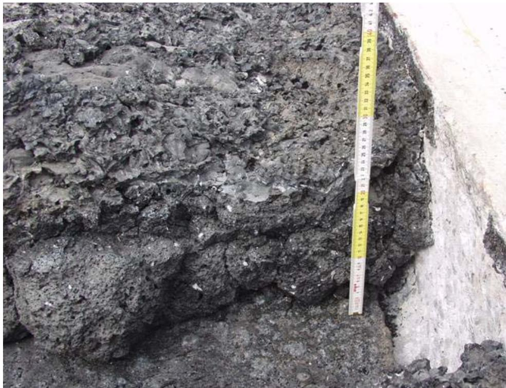
**Figure 3-27:** Left side of the solidified oxide melt in the trench at the opposite wall.
