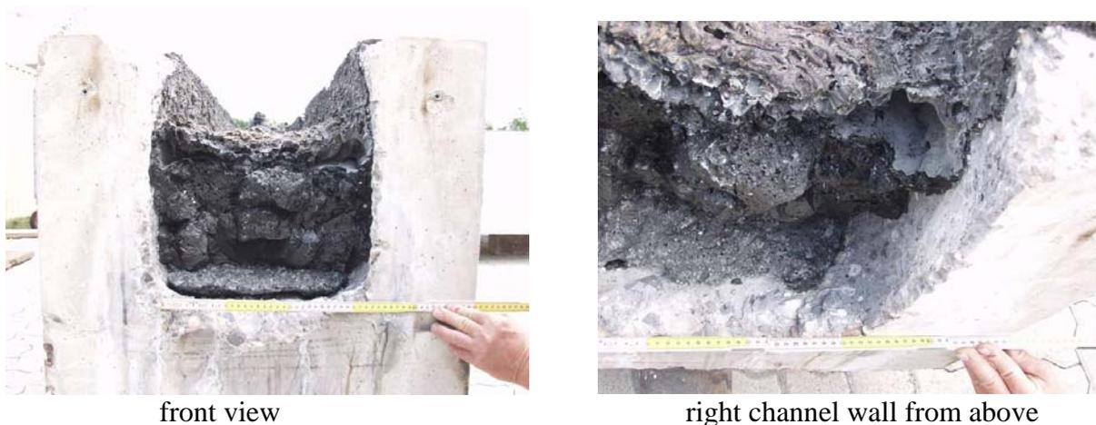
**Figure 3-9:** Erosion of concrete at the beginning of the supply channel
