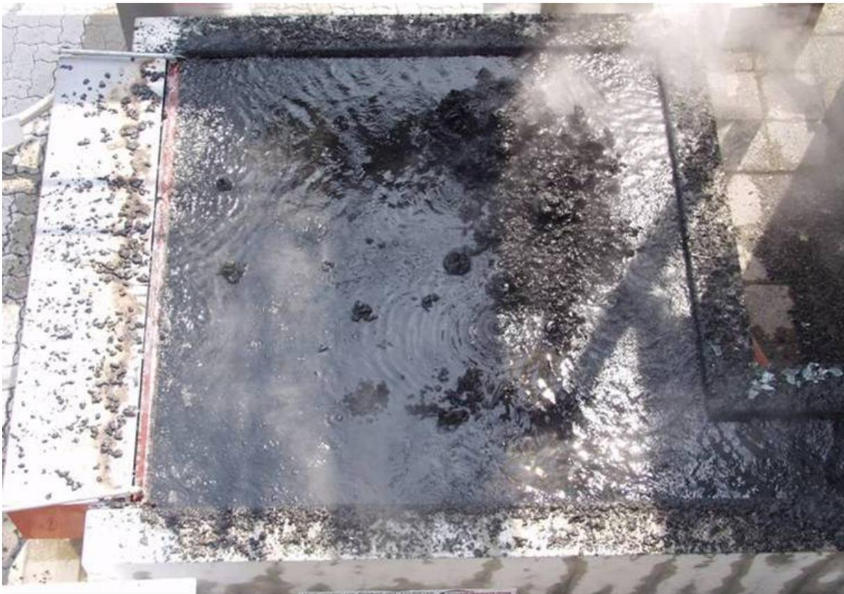
Figure 3-5: Water layer above the melt at the end of the 6<sup>th</sup> flooding period
