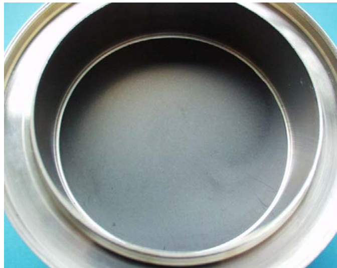
Fig. 8: Window insert consisting of CVD-diamond disk, Inconel cuff and Steel side walls of cooling chamber as removed from torus window demonstrator.
