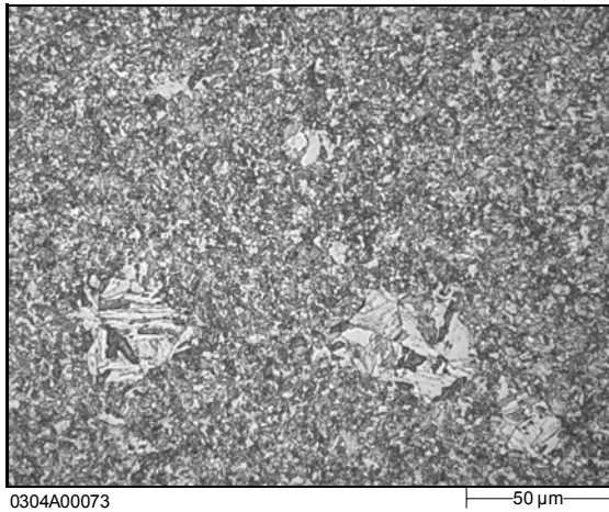
Fig. 1: Etched cross section: mainly tempered martensite (HV30 ~ 320), more ferritic (?) islands (white spots) Specimen orientation: L-S, sample taken from plate 155 x 62 x 10 mm 3 Heat treatment: 1100°C 30 min Ar/water + 750°C 2 h V/V.
