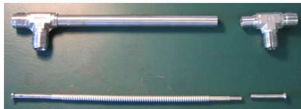
Fig. 2: Picture of two coaxial tube PERMCAT parts before final assembly.
