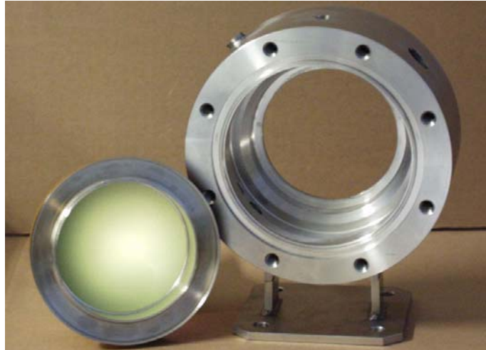
Fig. 10: Torus window demonstrator disassembled into outer housing and window insert.
