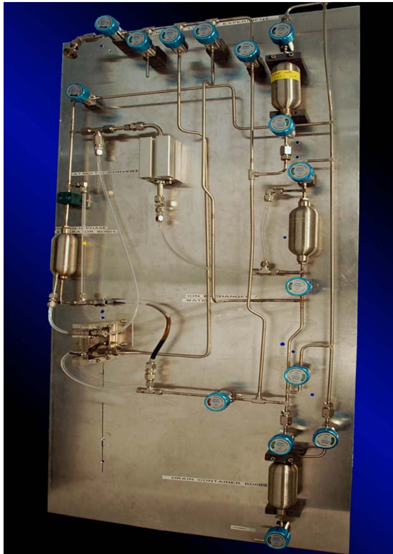
Fig. 3: The experimental rig to test the SPM lifetime.
