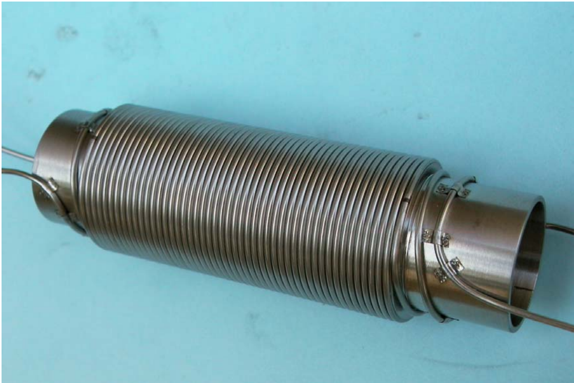
Fig. 7: Double heater helix on the inner wall for the ITHEX annular test section.
