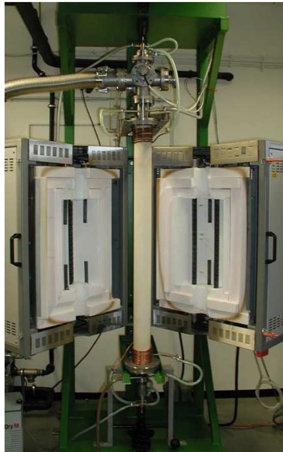
Fig. 1: High temperature creep rupture facility. A ceramic vacuum tube is used as container for the whole specimen test and measuring equipment. All flanges and seals are water cooled. For easier installation a fold-away furnace is applied to the testing device.
