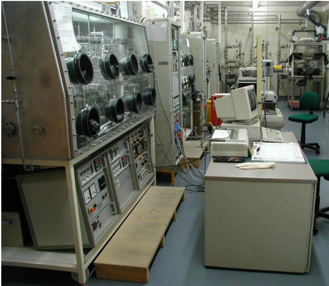
Fig. 1: Glove Box with Tritium and Helium Desorption Measurement Devices at Fusion Materials Laboratory.
