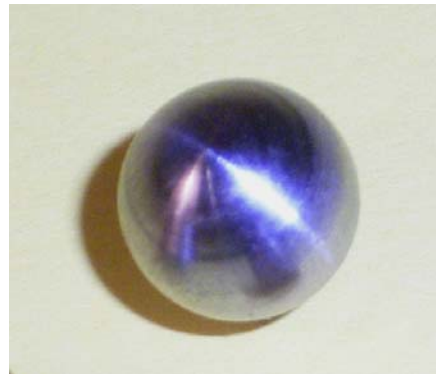
Fig. 6: W ball fabricated by turning Diameter 8 mm
