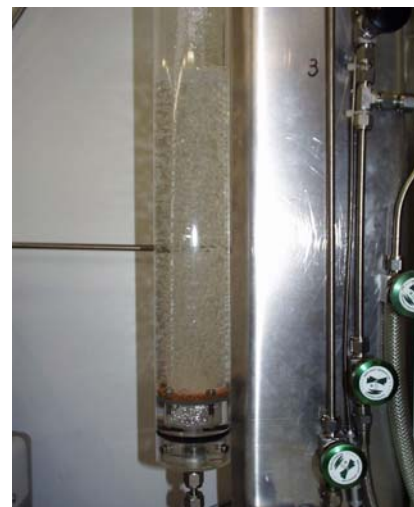
Fig. 1: Bubble column under operation with carrier gas He (at 1000 sccm) in water.
