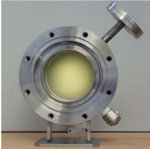
Fig. 9: Torus window demonstrator unit with special illumination to show the green transparency effect of the irradiated CVD-diamond disk (22DB2).
