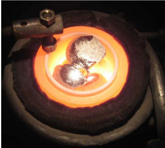
Fig. 4: The arc molten pellets were alloyed in a ceramic crucible by induction heating.
