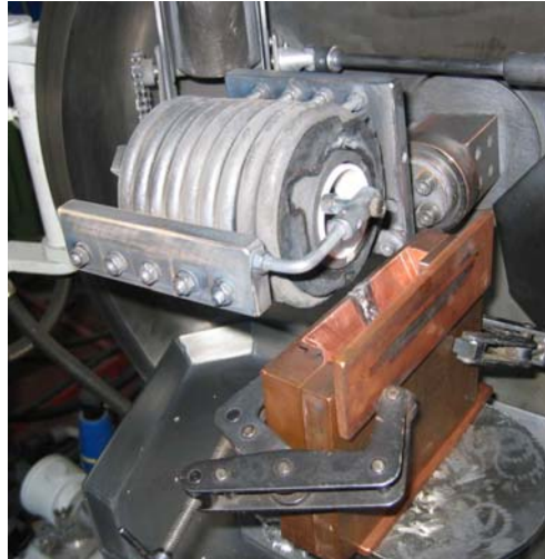
Fig. 5: The heat was finally cast into a copper mould.
