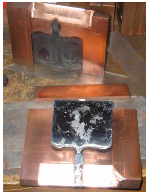
Fig. 6: The opened copper mould with the solidified heat.
