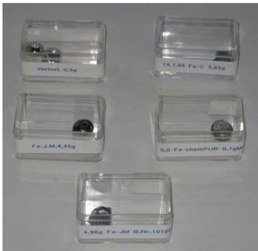
Fig. 3: In a first step the alloy components were arc molten to pellets.
