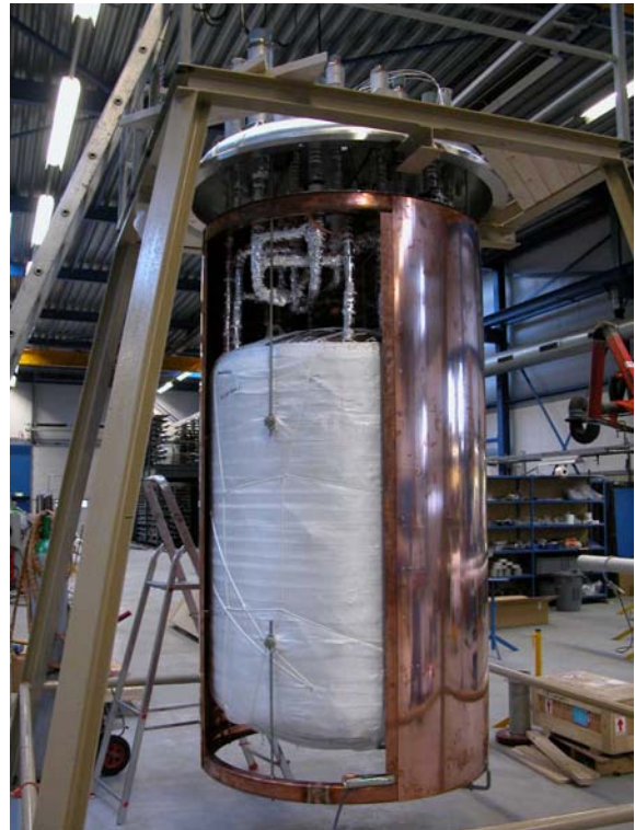
Fig. 2: Cryostat with valve box for the supply of the cryopumps.
