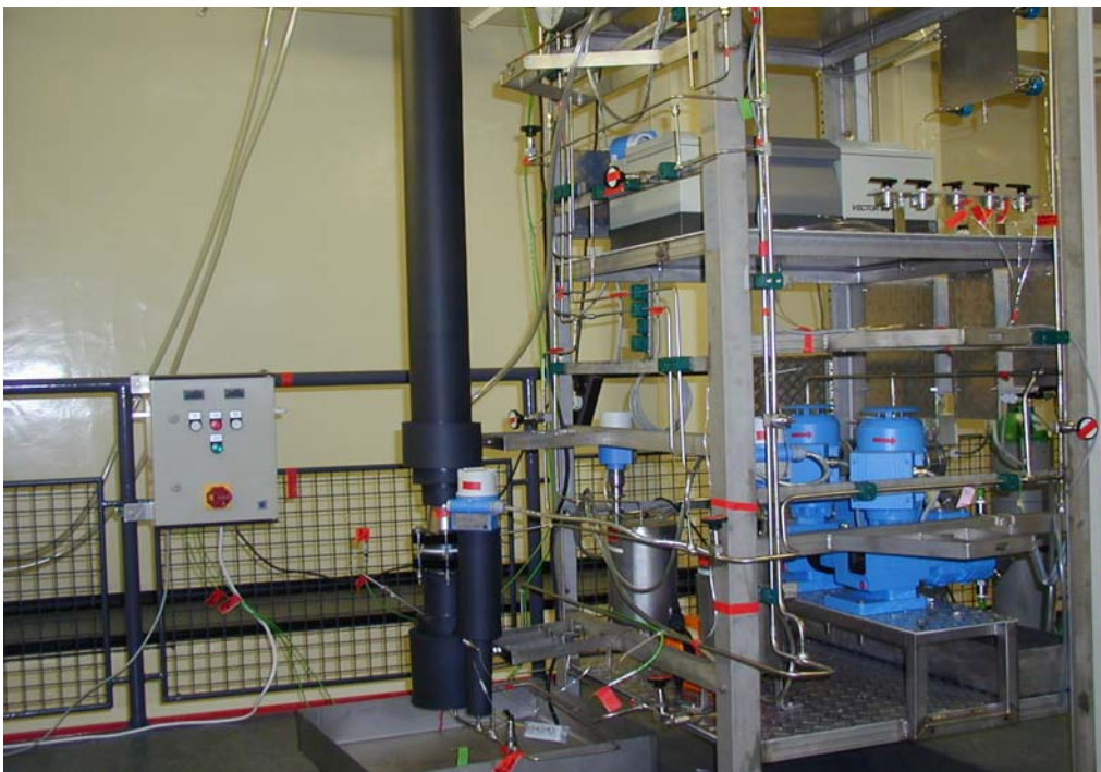
Fig. 2: Experimental rig for catalyst/packing endurance test.
