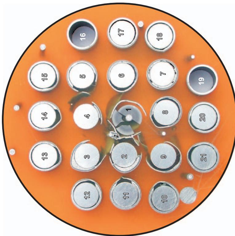
Fig. 76: Cross section at 1320 mm bundle elevation (QUE-08-14); overview from top.
