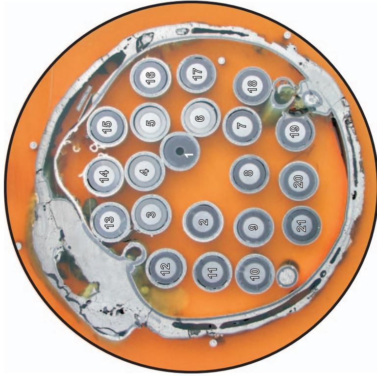
Fig. 64: Cross section at 950 mm bundle elevation (QUE-08-6); overview from top.
