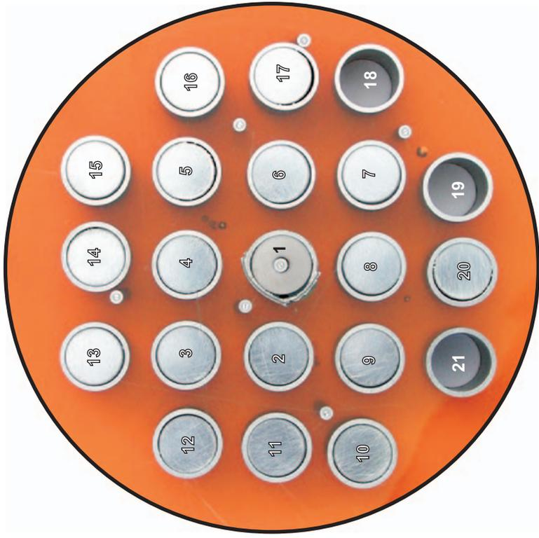
Fig. 80: Cross section at 1480 mm bundle elevation (QUE-08-16); overview from top.
