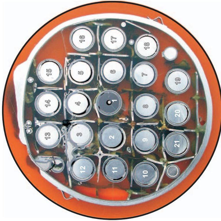
Fig. 70: Cross section at 1065 mm bundle elevation (QUE-08-11); overview from top.
