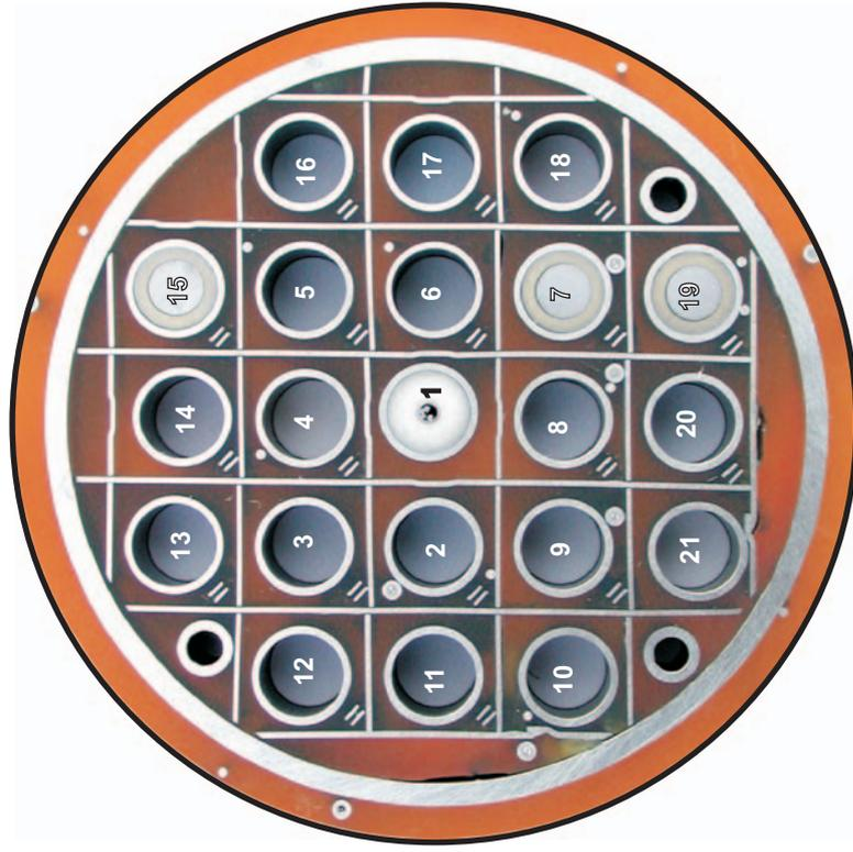
Fig. 51: Cross section at 73 mm bundle elevation (QUE-08-1); overview from top, reference elevation.
