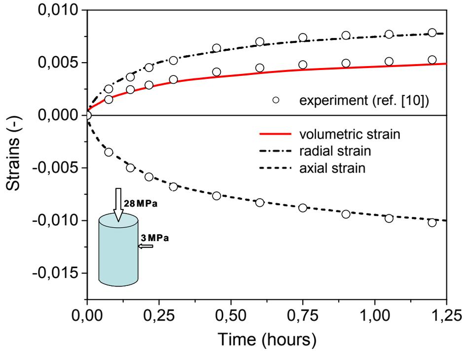
Fig. 1: Comparison between measured creep strains and calculation results
