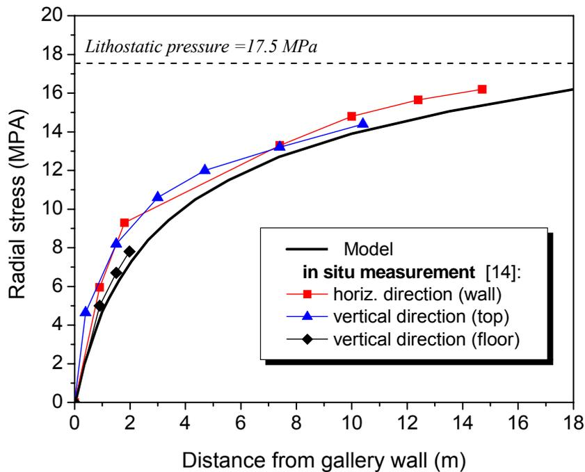
Fig. 12: Comparison of the measured and calculated minimal stresses 37 years after excavation
