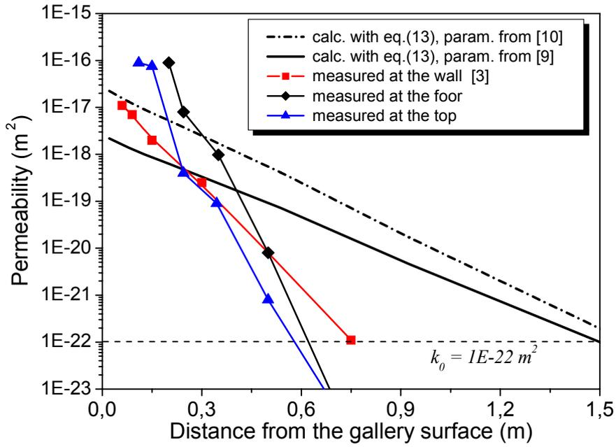
Fig. 11: Comparison of the calculated and measured distribution of rock salt permeability 37 years after excavation
