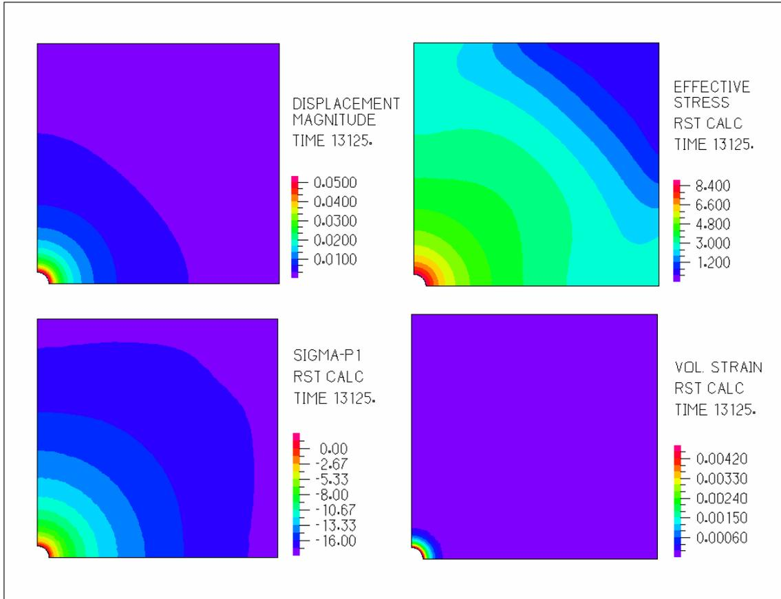
Fig.13: Distribution of displacement, effective stress, minimal stress, and volumetric strain 37 years after excavation
