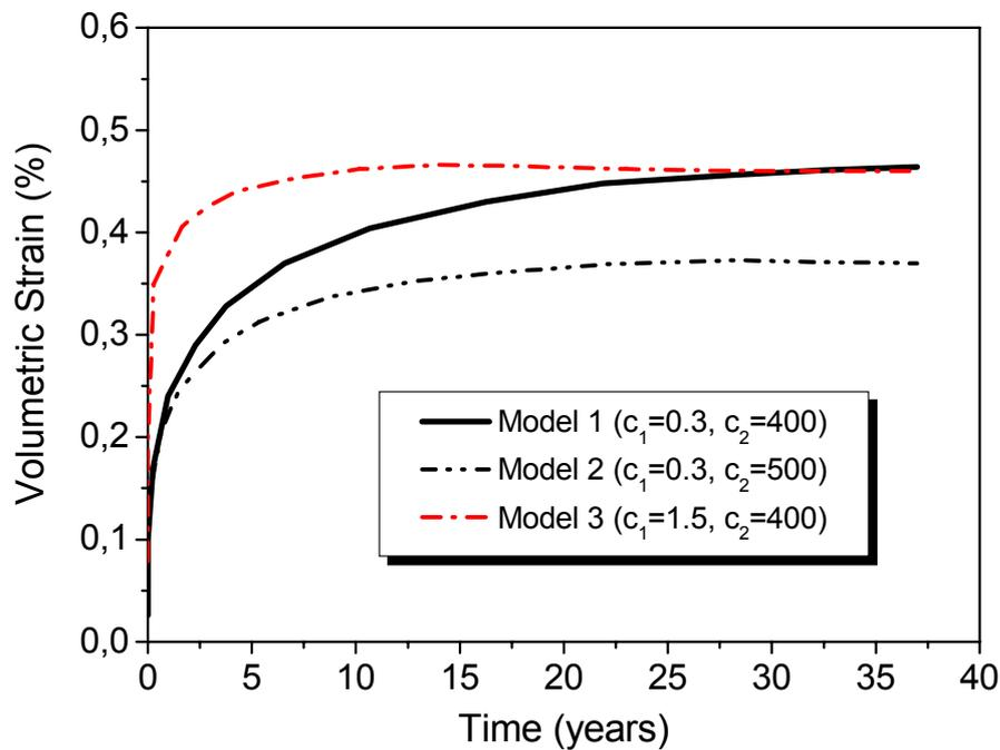
Fig. 10: Model prediction of volumetric strains in rock salt at 5 cm distance from the gallery surface
