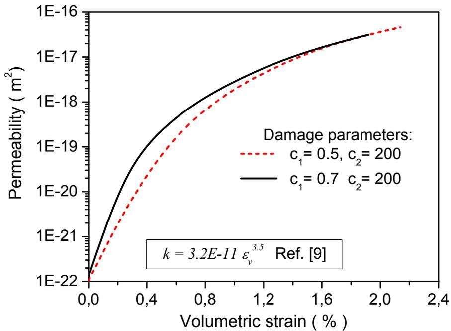
Fig. 5: Permeability as a function of volumetric strain for two sets of parameters
