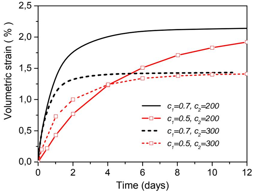
Fig. 4: Development of volumetric strain for various values of model parameters
