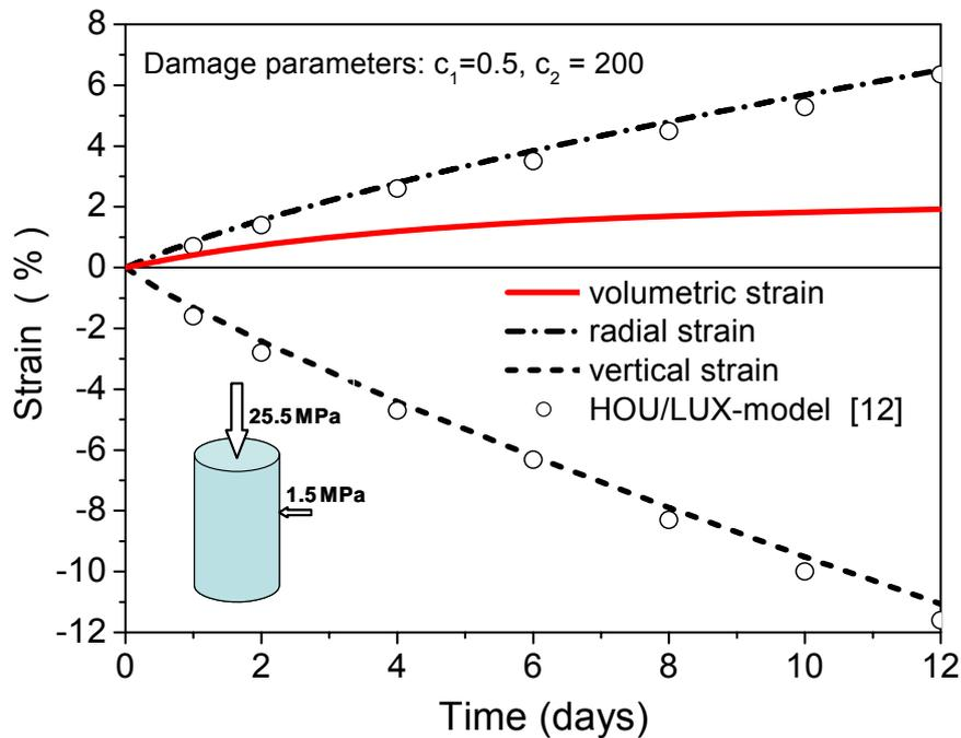
Fig 3: Comparison between results calculated with the proposed damage model and the Hou/Lux model [12]
