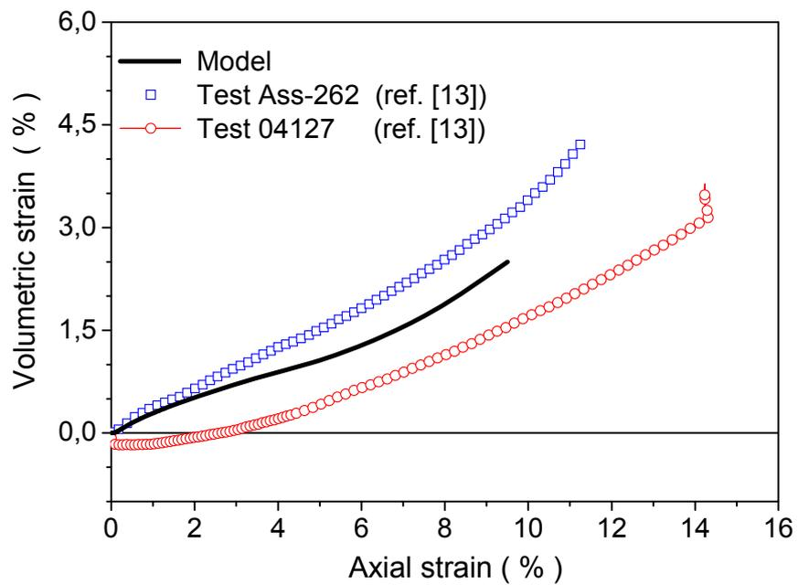
Fig. 7: Development of volumetric strains as a function of axial strain and comparison with calculation results
