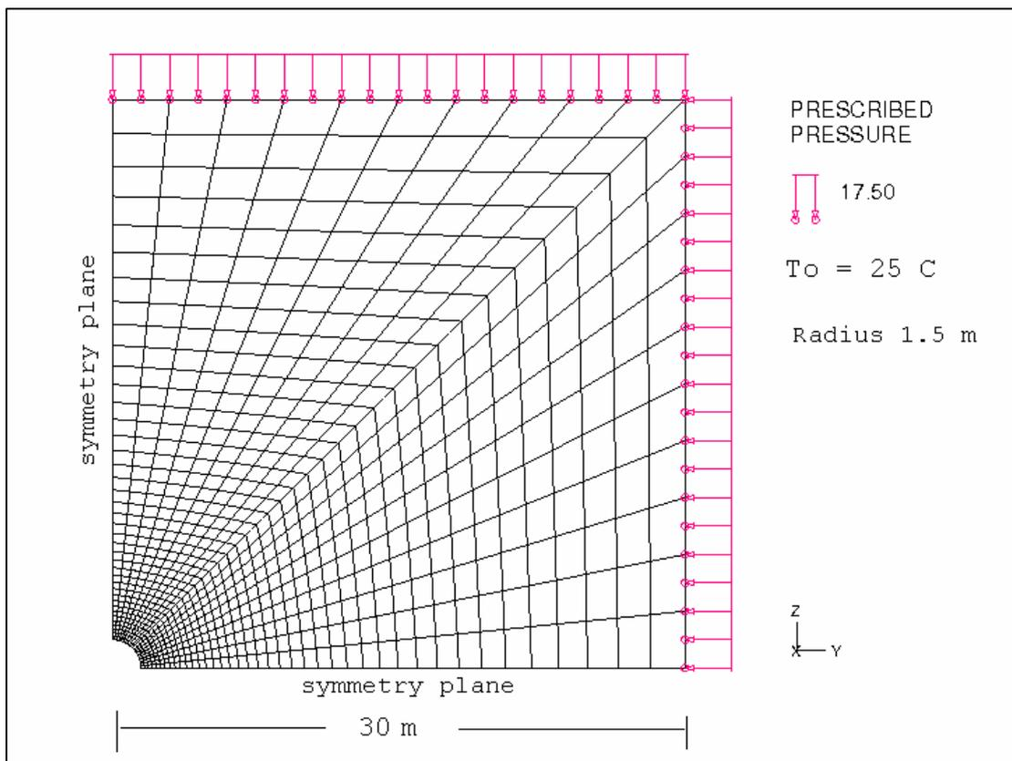
Fig. 8: Finite-element mesh and initial boundary conditions
