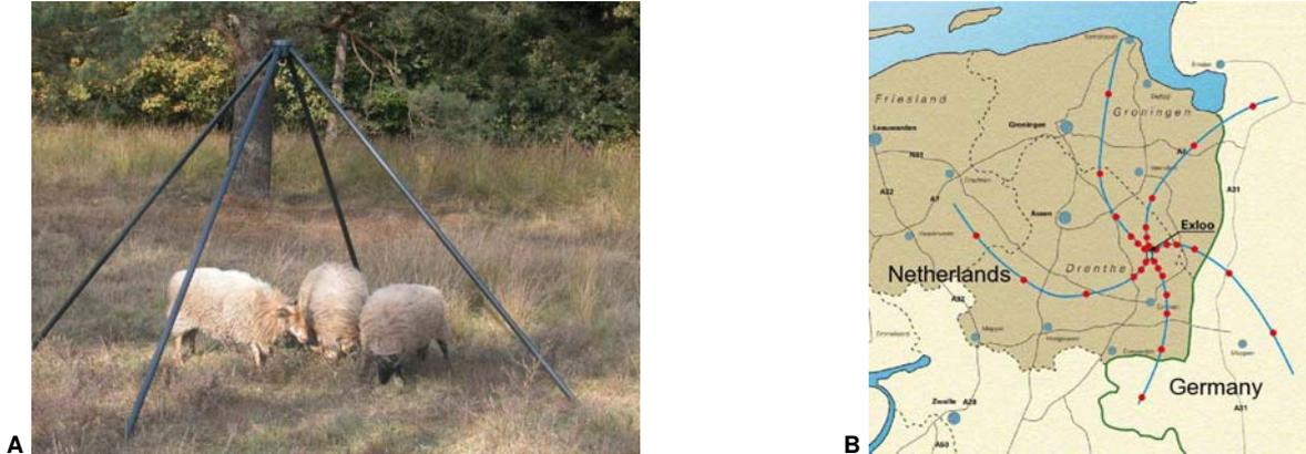
**Figure 1.** **A:** A prototype LOFAR antenna. The dipoles run down the black PVC tubes. **B:** LOFAR layout showing the core and logarithmically spaced remote stations on five spiral arms in the border region of the Netherlands and Germany.
