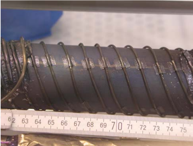
Fig. 2: Detail of heaters with covering foil removed showing gap between heaters and permeator tube.
