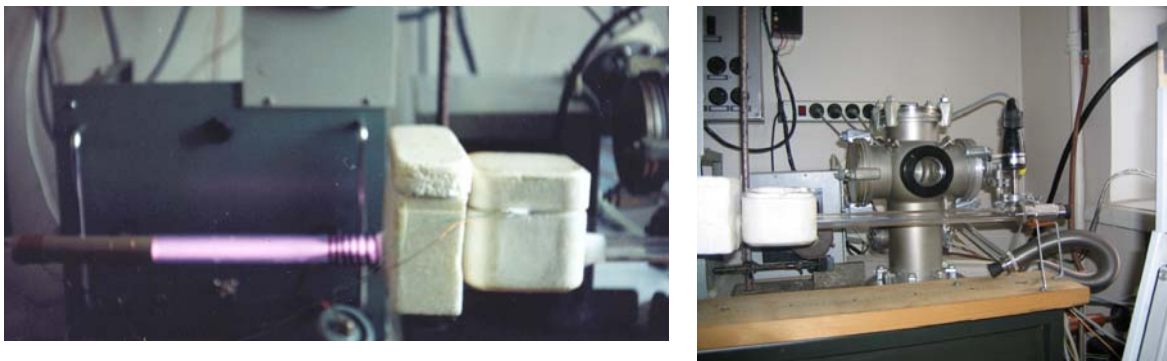
Fig. 1: Top : Scheme of the quartz gas flow reactor for experiments with charcoal in atomic/molecular hydrogen mixture at 77 K. Gas flow controllers were installed at the tube inlet. Bottom : Photos of H 2 RF discharge with cold LN traps (left), and the vacuum and gas analysis part with mass spectrometer and gauges.
