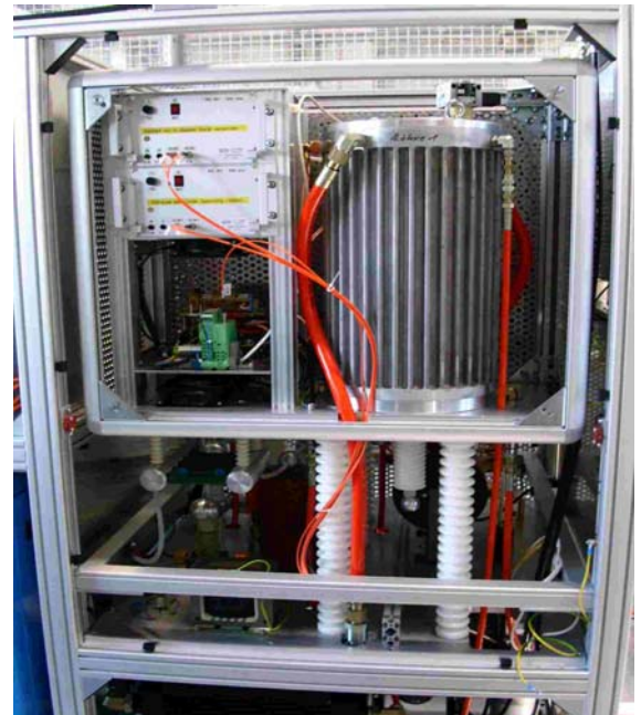
Fig. 9: HV control system for a gyrotron: It consists of a body voltage modulator and of a heater and thyatron protection unit. Left: HV control system for the W7-X gyrotrons (from left: modulator, crowbar and ignition coil. Right: Details of the HV modulator: Tube compartment with cooling hoses on HV isolators.
