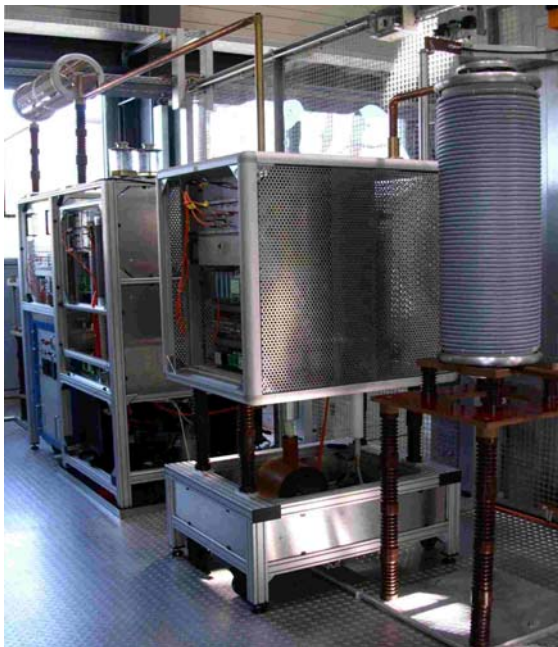
Fig. 9: HV control system for a gyrotron: It consists of a body voltage modulator and of a heater and thyatron protection unit. Left: HV control system for the W7-X gyrotrons (from left: modulator, crowbar and ignition coil. Right: Details of the HV modulator: Tube compartment with cooling hoses on HV isolators.
