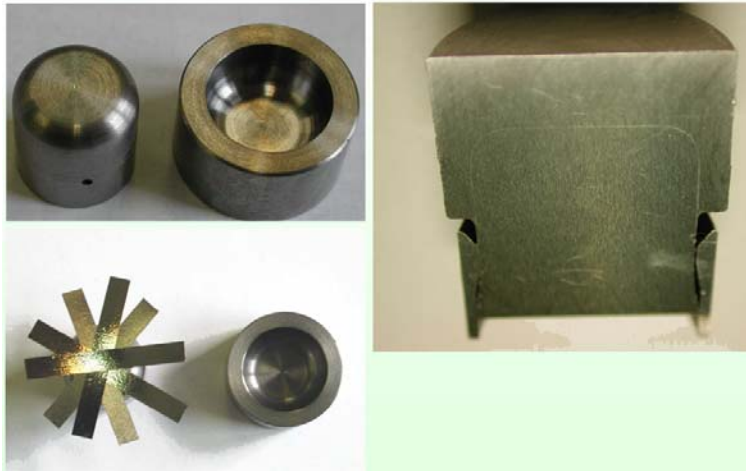
Fig. 7: W-W joint with real curved surface successfully tested with STEMET 1311® filler metal.
