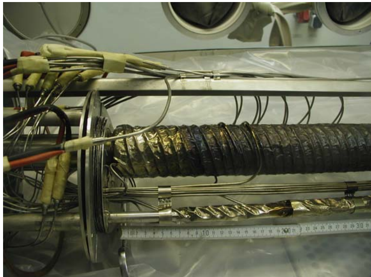
Fig. 1: Permeator element exposed showing the heater arrangement, discoloration of the foil.
