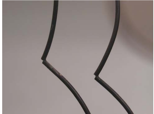
Fig. 3: Heater removed from permeator showing brittle fracture of sheath.
