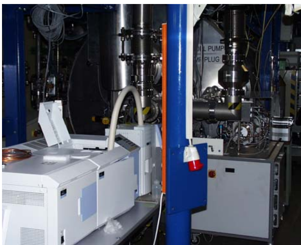
Fig. 1: The two analytical devices used for monitoring the tracer gas release behaviour in TIMO: A GC-MS (in the front) and a stand-alone quadrupole MS (in the back).
