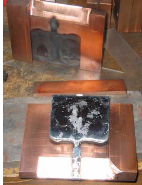
Fig. 2: The opened copper mould with the solidified heat.
