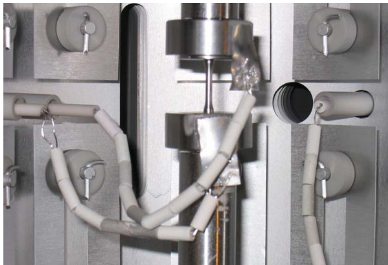
Fig. 1: High temperature pull rods for tensile- and LCF-testing with Pt-PtRh-TC application by intermediate tantalum foils welded on holder rings.
