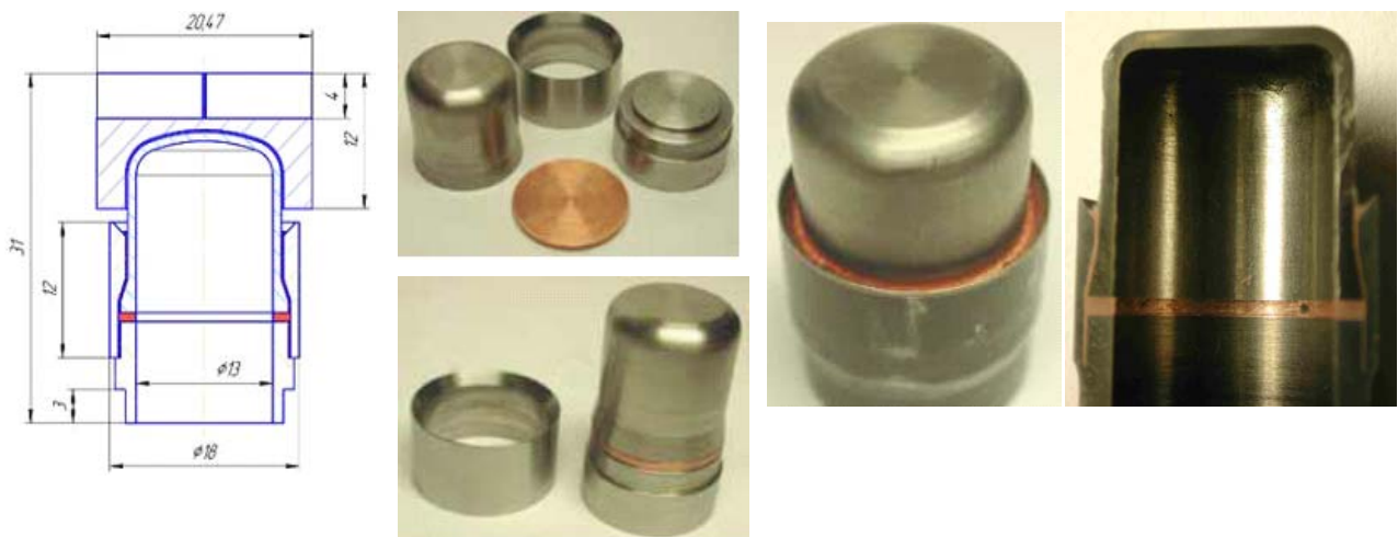
Fig. 8: W-steel joint with conic lock and Cu casting successfully tested under thermocyclic and internal loadings.
