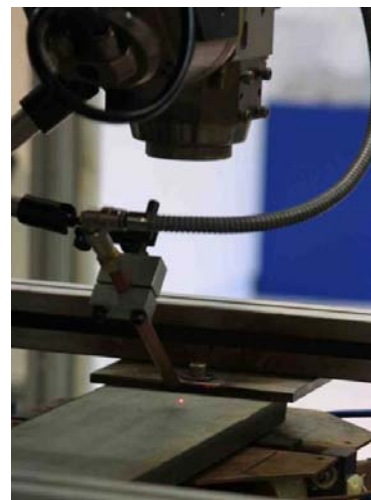
Fig. 4: Schematic view and photo of the CO 2 laser beam welding with EM weld-pool support. Both the magnetic field and the electric current in the welded material are directed parallel to the surface.
