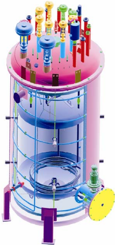
Fig. 2: 3D scheme of the cryostat with valve box for cryosupply.
