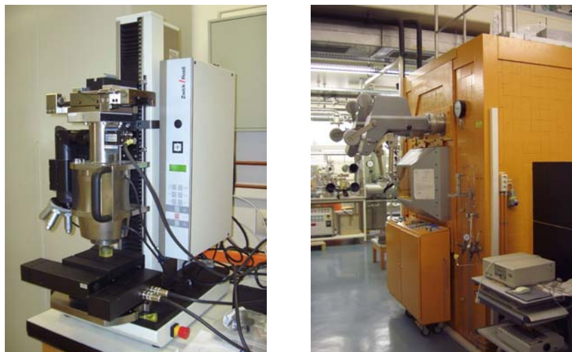
Fig. 1: Zwick system with depth and force reading hardness measurement, xy-stage, and microscope (left) and Box 4 in FML in which the machine will be installed (right).
