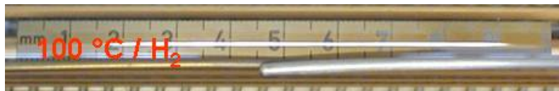
Fig. 3: Deformation of a finger-type Pd / Ag membrane during H_2 permeation at 100 °C.
