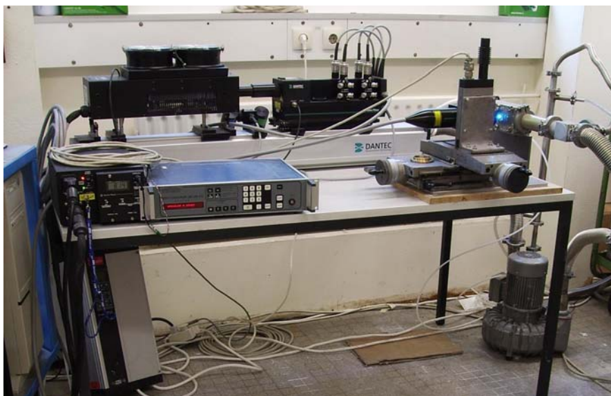
Fig. 6: Setup of LDA system for minichannel measurements.
