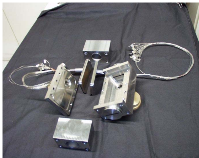
Fig. 2: Parts for the ITHEX rectangular test-section: heater plates, thermocouples, and housing.
