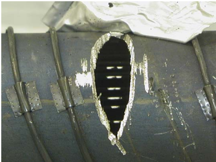
Fig. 4: Cut into permeator element showing Pd/Ag tubes and black powder deposits.
