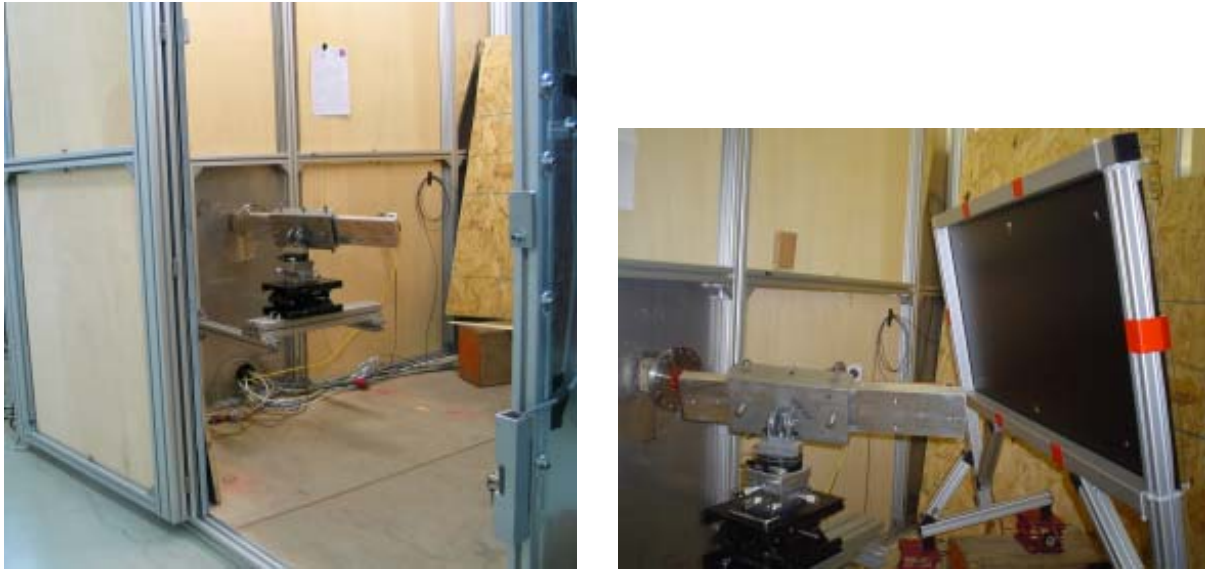
Fig. 8: View into the diagnostics box with the fixed mirror at the launcher front end (left) and the arrangement of the diagnostic screen relative to launcher front end (right).
