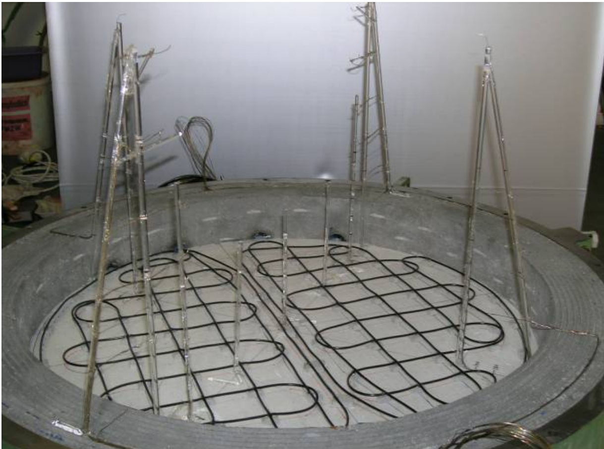
Figure 6: Instrumentation during crucible fabrication: Light guides (black sheathing) and thermocouples fixed to glass rods
