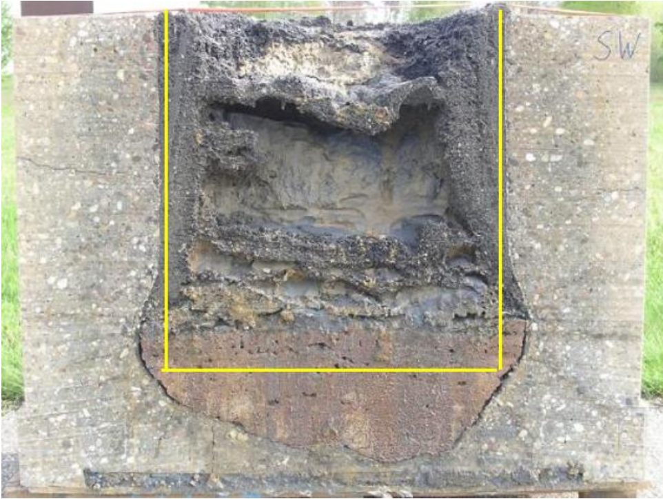
Figure 27: Eroded concrete crucible sectioned in direction NE-SW
