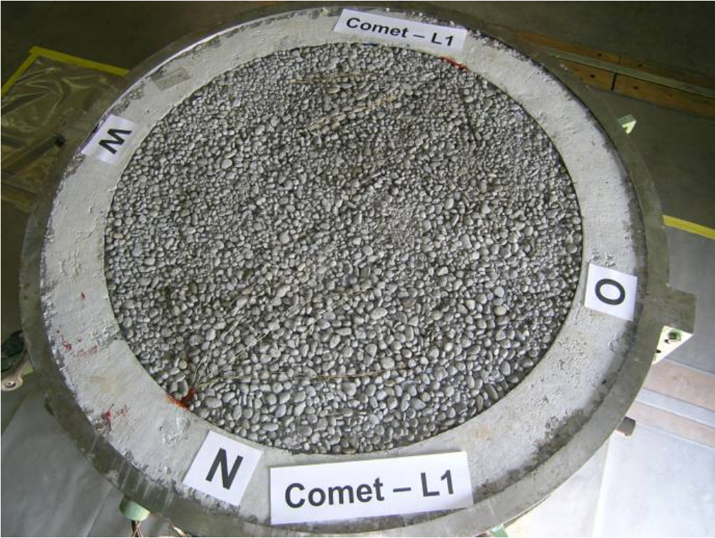
Figure 9: Fabrication of the cylinder wall of the concrete
