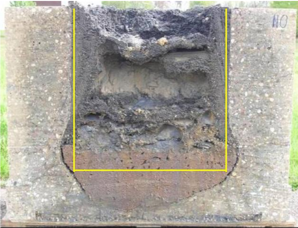
Figure 28: Eroded concrete crucible sectioned in direction SW-NE
