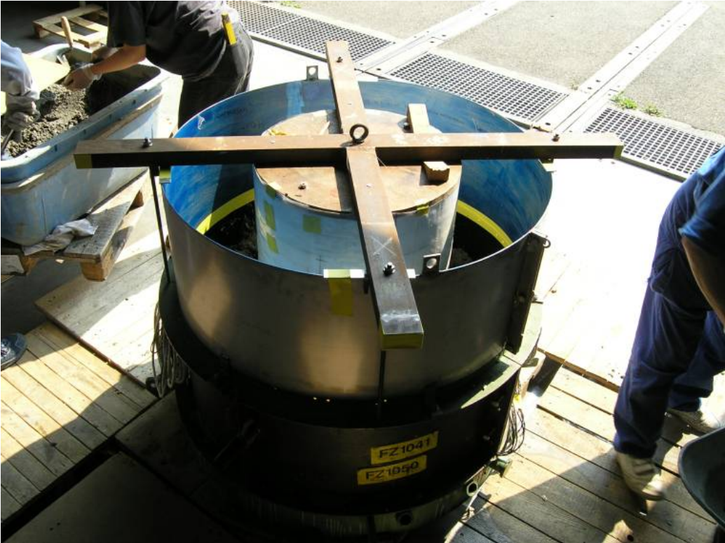
Figure 9: Fabrication of the cylinder wall of the concrete
