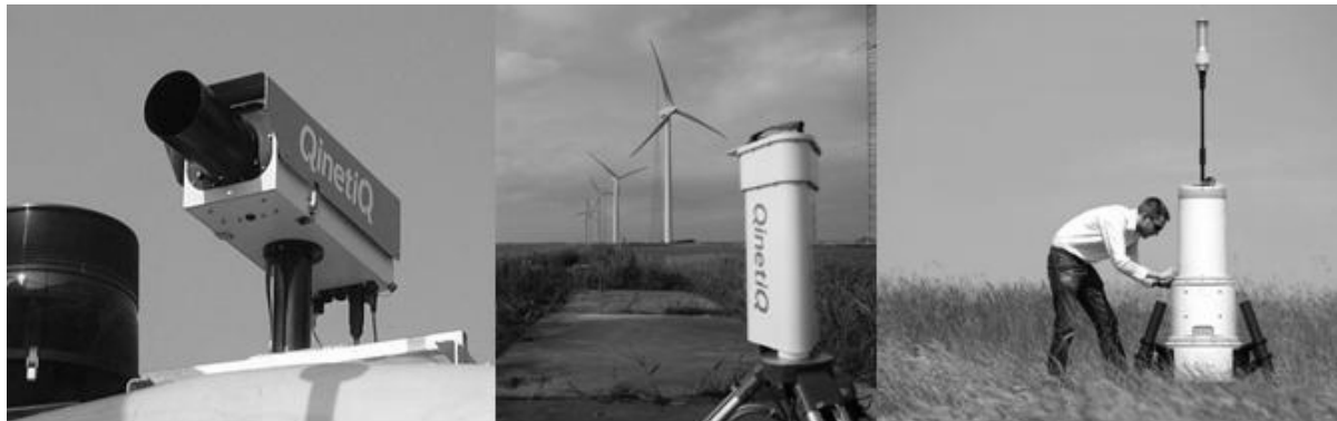
Figure 1-3: Stages of evolution of the ZephIR lidar. Figure 1 shows the lidar head mounted on the nacelle of a Nordex N-90 wind turbine. Figure 2 shows prototype ground-based wind profiler at Risø wind energy test site, Høvsøre, Denmark. Figure 3 shows the ZephIR production model deployed in the field.
