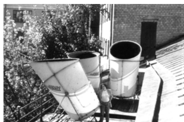
Figure 1. The antenna systems of the sodar Latan-3 at two measuring sites: on the roof of the IAPh building in the center of Moscow (left) and on the roof of Physical Faculty of MSU (right).
