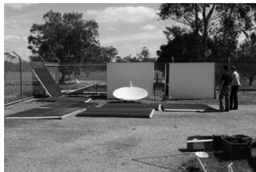
Figure 1. This new RAMP instrument, recently developed in Australia, enables very high spatial and temporal resolution profiles of the boundary layer. The system consists of four receive antennas and one centre transmit antenna shown here being assembled. The centre transmit has since been replaced by four transmit antennas placed outside the receive antennas to overcome issues identified in the first testing.
