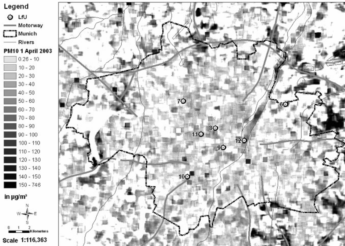
Figure 1: Region of Munich with the spatial distribution of PM10 concentrations in \mu\text{g}/\text{m}^3 on April 1, 2003 calculated with the reference image of April 16, 2000. The measurement sites of the Bavarian State Agency for Environmental Protection, rivers and motorways are indicated.
