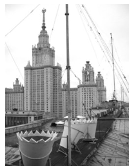
Figure 1. The antenna systems of the sodar Latan-3 at two measuring sites: on the roof of the IAPh building in the center of Moscow (left) and on the roof of Physical Faculty of MSU (right).
