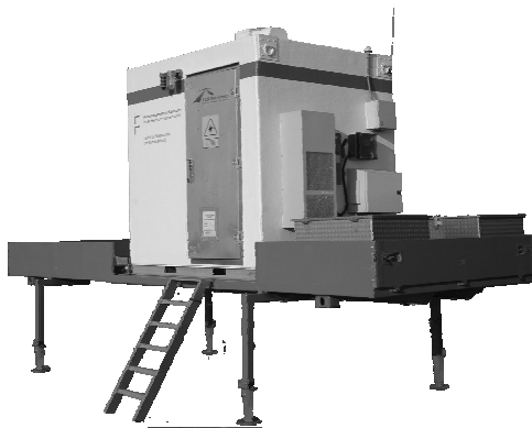
Figure 1: WindTracer 2 \mu\text{m} Doppler Lidar Figure 2: Doppler Lidar measurement principle
