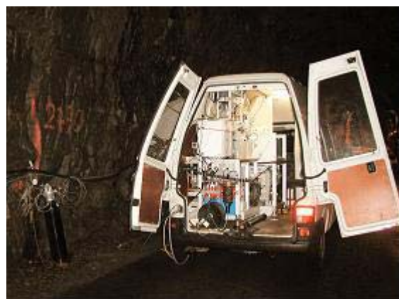
Fig. 1 The mobile LIBD detection system in the Äspö tunnel (not referred to in text)
