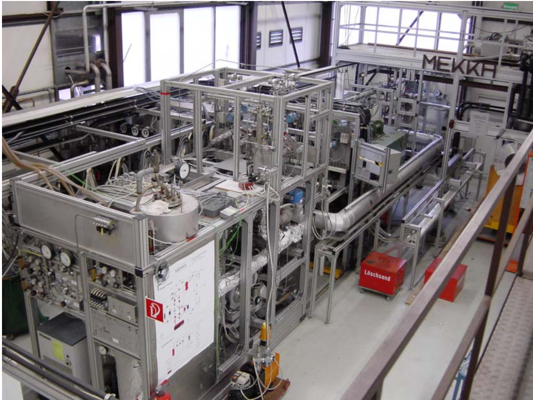
Figure 8: View on the liquid-metal NaK loop of the MEKKA laboratory
