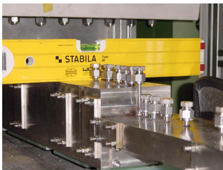
Figure 4: Test section during installation into the liquid-metal loop. All pressure taps are closed.
