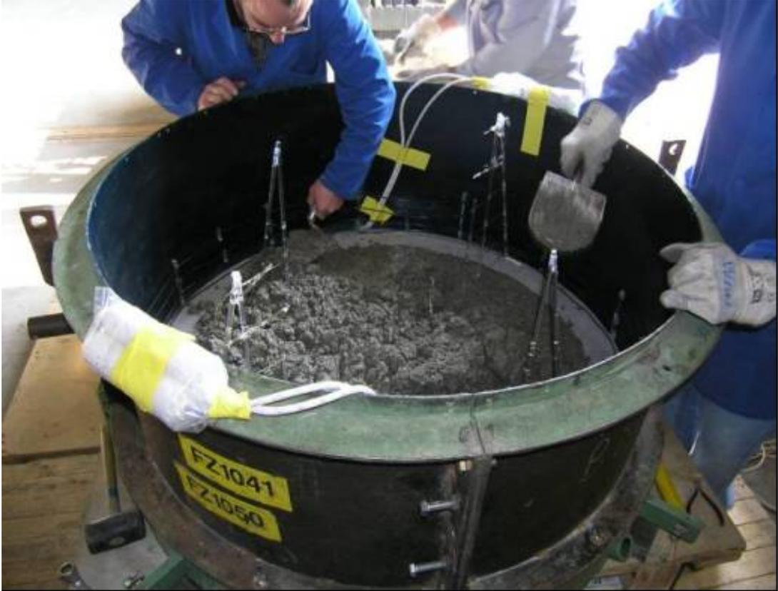
Figure 8: Fabricating the concrete crucible
