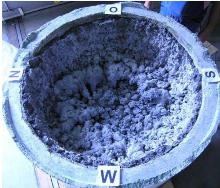
Figure 36: View of the melt surface after the test
