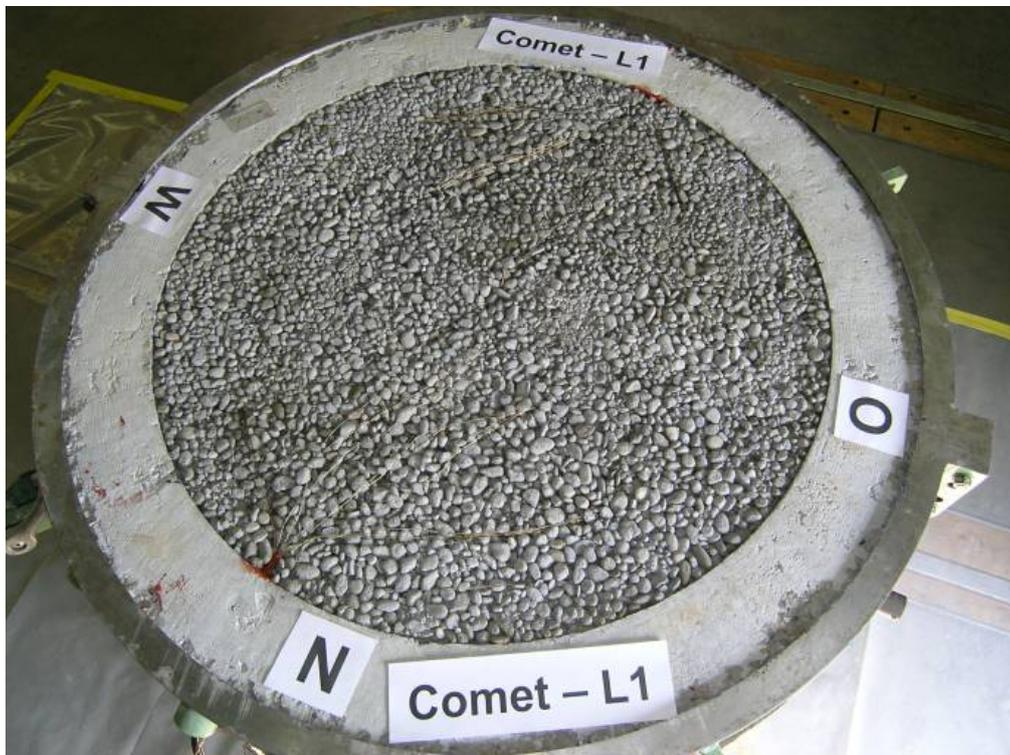
Figure 10: The 4 cm thick porous concrete layer under the crucible (upside down)
