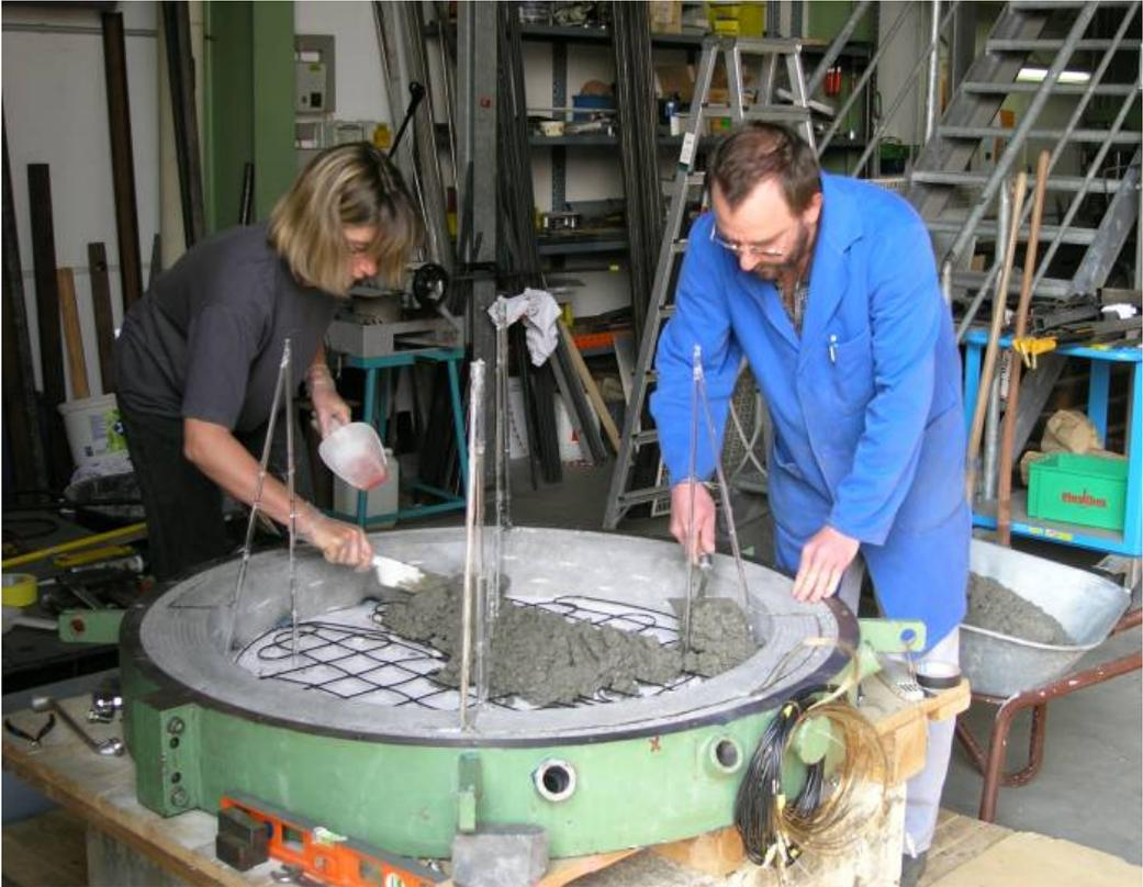
Figure 7: Fabricating the bottom of the concrete crucible
