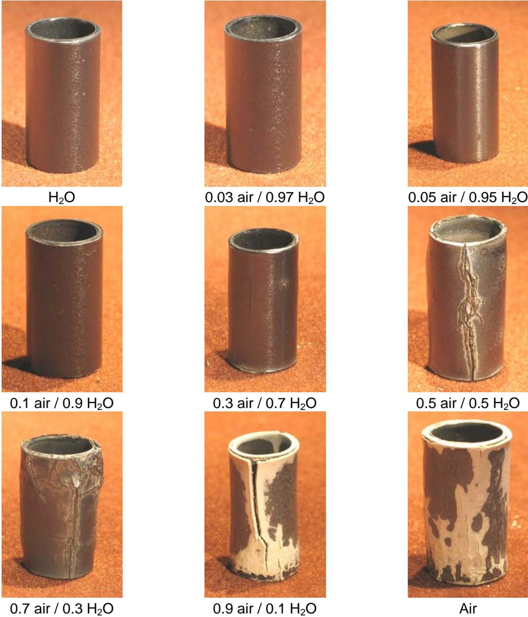
Post-test appearance of specimens oxidised 1 h at 1100 °C
