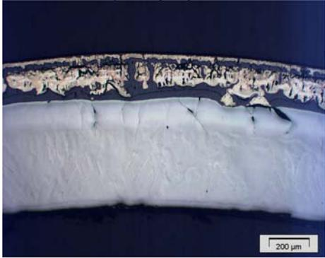
10s\* PO (20µm), 31min N<sub>2</sub>
