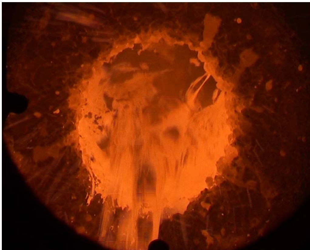
Figure 15: Eruption of melt upon removal of interfacial crust (290 s)
