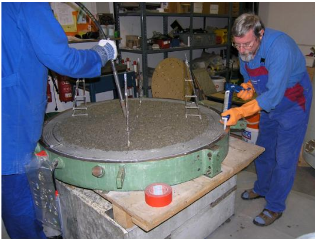
Figure 8: Fabricating the bottom of the concrete crucible
