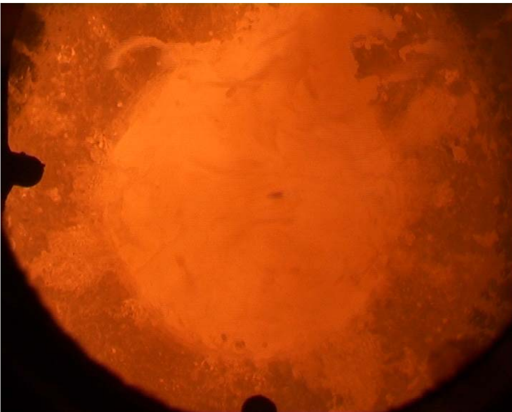
Figure 13: Intense melt concrete interaction with melt splashing at 115 s
