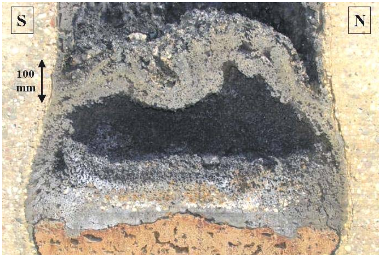
Figure 51: Close-up view of the solidified oxide with large inner cavity and crust
