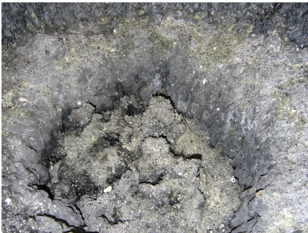
Figure 43: Closer view to the central melt and the rim of the concrete cavity
