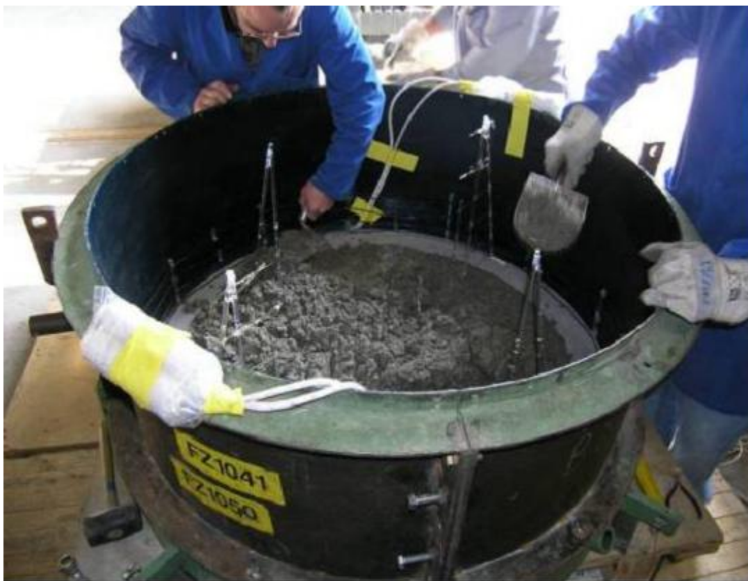
Figure 9: Fabricating the concrete crucible
