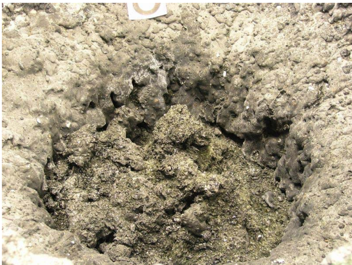
Figure 45: Closer view to the melt surface and the concrete cavity
