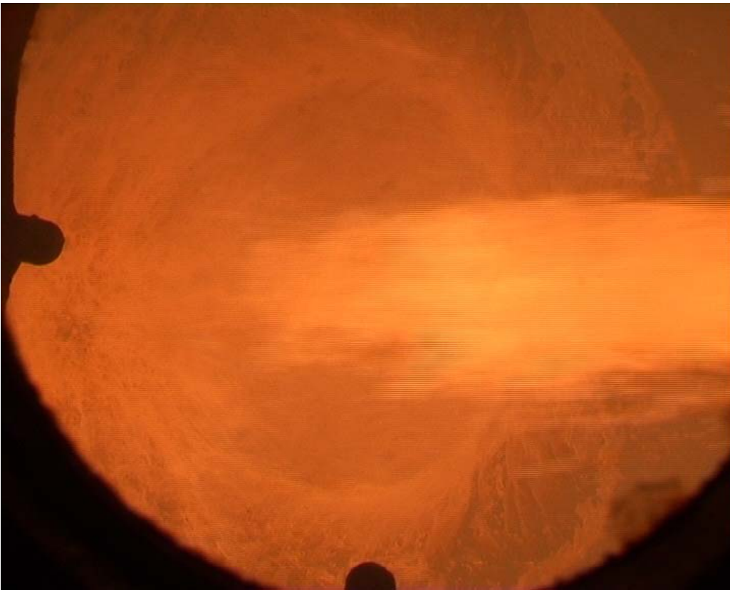
Figure 12: Pour of the oxide melt fraction at 11 s
