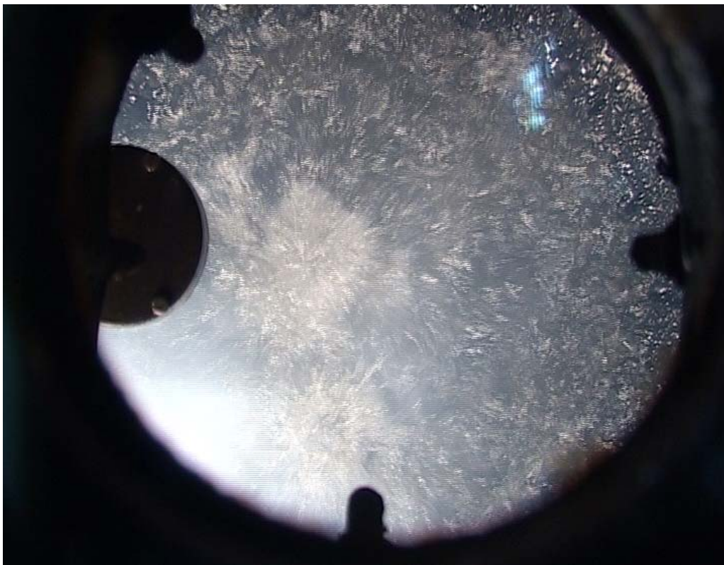
Figure 17: Continuous boiling of the flooded melt surface (1680 s)
