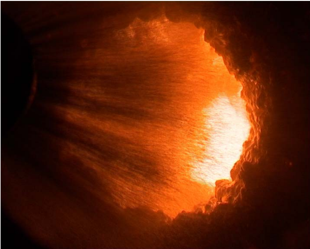
Figure 16: Flooding the melt surface by a showerhead (840 s). The melt forms a darker, viscous surface layer
