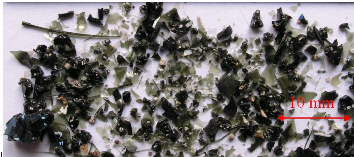
Figure 47: Loose oxidic/glassy debris ejected during volcanic eruption
