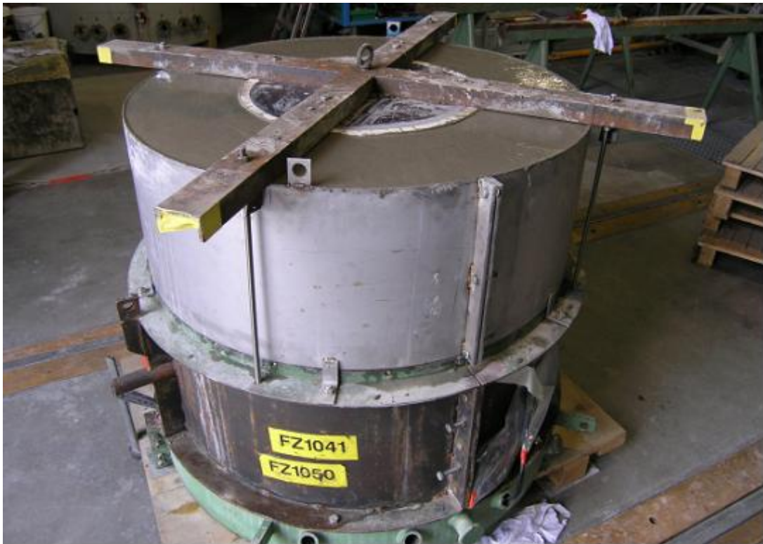
Figure 10: The mould for the cavity filled with concrete
