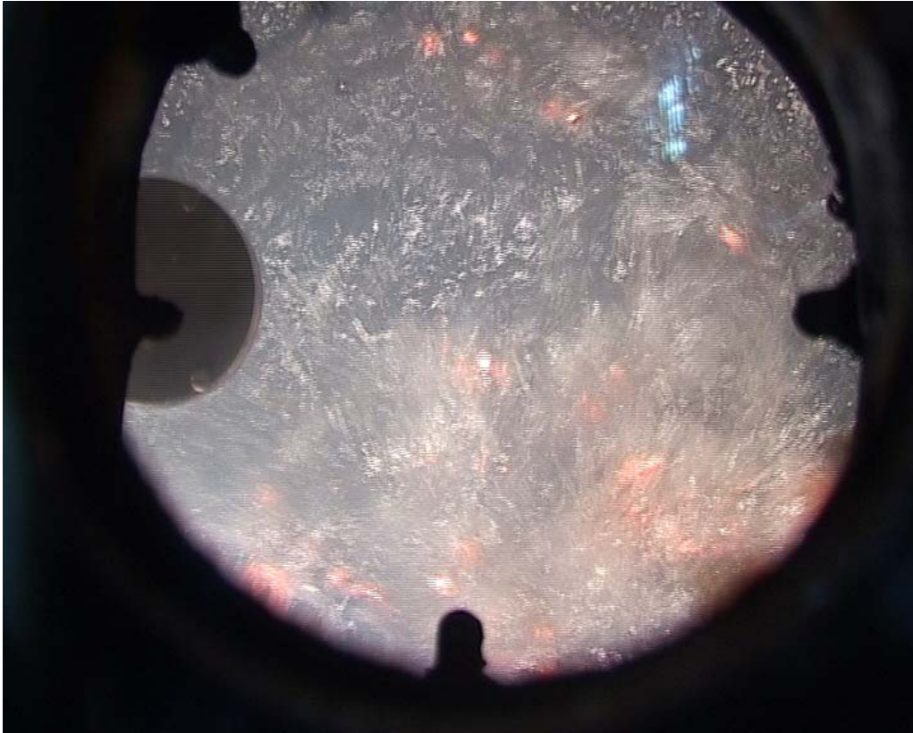
Figure 18: Volcanic melt eruption through the flooded surface at 1760 s. Hot oxide particles are injected into the boiling water layer.
