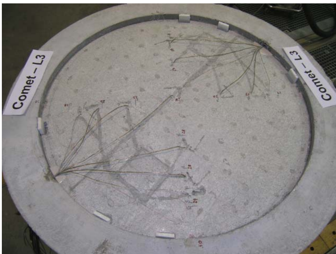
Figure 11: The lower side of the concrete crucible with the 30 mm deep cavity
