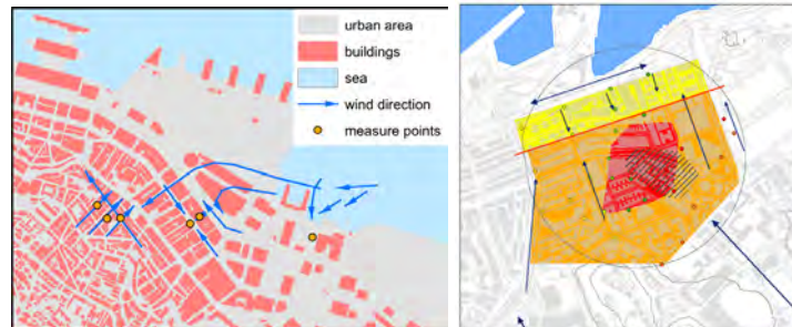
Fig. 3: Case study wind distribution (left), climate mapping with UHI and wind reduction zonings (right), PET values and neutral thermal conditions (right) from a one day experiment with easterly wind flow. Measurements were taken at 26 th November 2005. Each point again had three different spots to get the average characteristic of the place.
