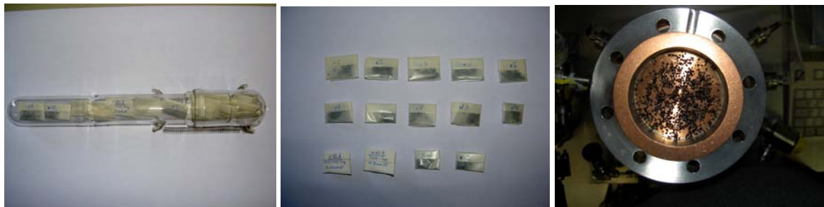
Fig. 1: The radical exposed charcoal sample from IPC-RAS. Left : In the glass ampoule, as received; middle : The individual samples; right : The total sample inside the COOLSORP test cell.
