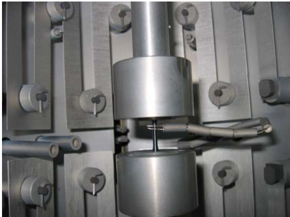
Fig. 1: Temperature calibration arrangement of the tungsten LCF specimen.
