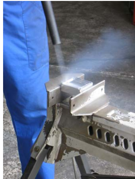
Fig. 5: Cleaning procedure with CO 2 pellets applied to a CMU. CO 2 pellets are accelerated to about twice of sonic speed. They ice pollutions and shave the pollutions by mechanical impact.
