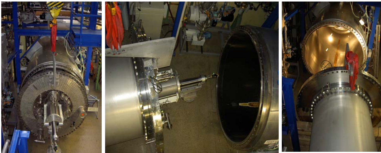
Fig. 2: Steps of the ITER model pump dismantling from the test vessel.
