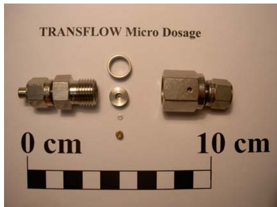
Fig. 4: The orifice flow device for establishing very small flows, and the test set-up for its calibration.
