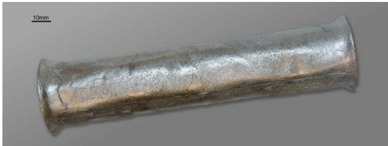
Fig. 1: Be-Ti rod consisting of Be 12 Ti phase fabricated by method of Hot Isostatic Pressing.
