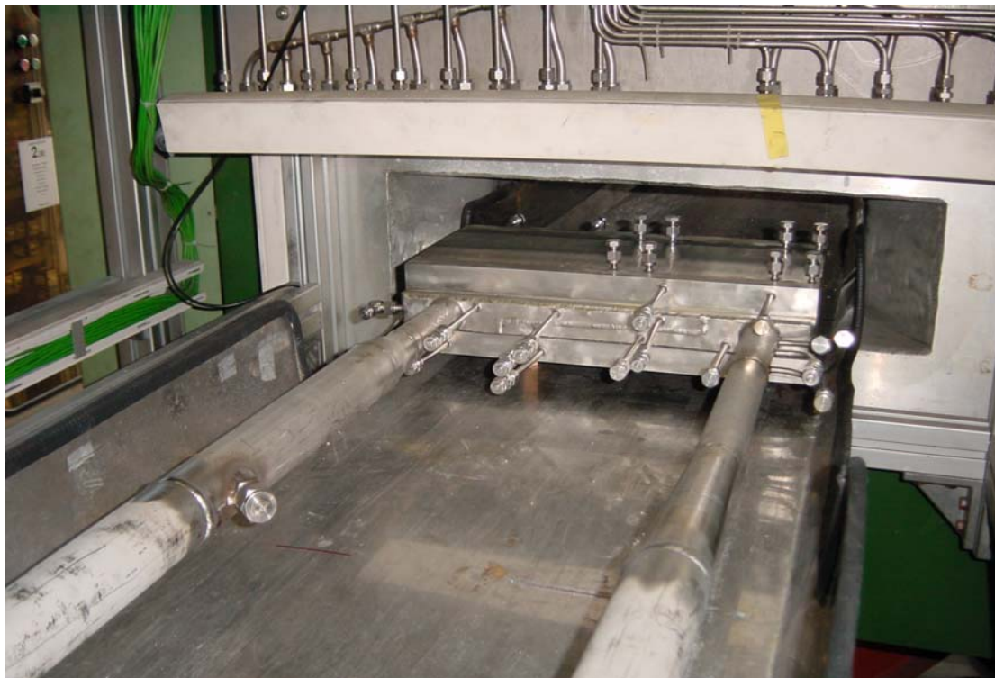
Fig. 1: MHD mock up connected to the liquid metal loop, here positioned in front of the magnet.
