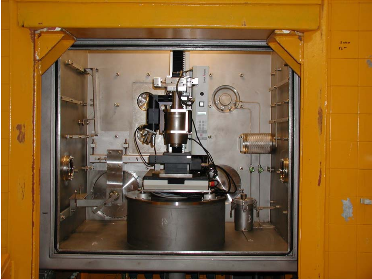
Remotely controlled indenter during mounting into FML box no. 4
