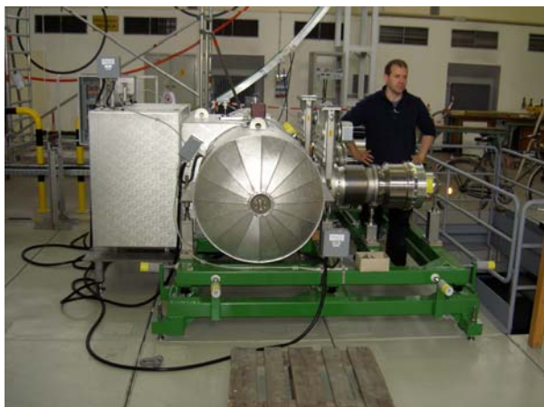
Fig. 4: The orifice flow device for establishing very small flows, and the test set-up for its calibration.
