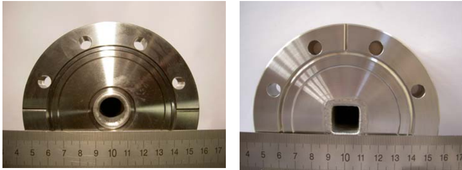
Fig. 6: Cross-sections of the first test channels: A long circular duct (diameter 16 mm), and a long square duct (hydraulic diameter 16 mm), with a length/diameter ratio of 80.
