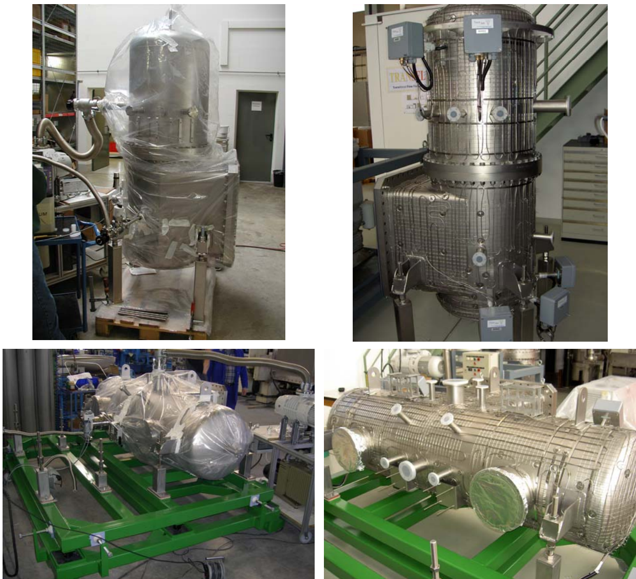
Fig. 2: Top: Photos of the dosing dome during the integral leak test at the manufacturer ( left ) and after the resistance heating system has been attached ( right ). Bottom: Correspondingly for the pump dome.
