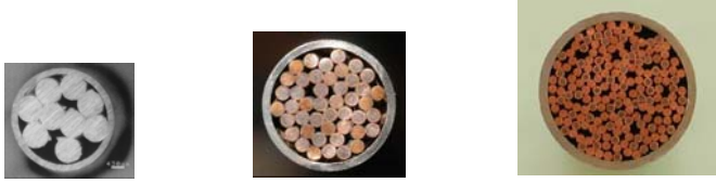
Fig. 2: Cross section view of the different sub-stages with the smallest cable layout of 3x3 (OD 3.3 mm), the larger 3x3x5 (OD 7.6 mm) and the largest cable in conduit sample with 3x3x5x4 layout (OD 15 mm).
