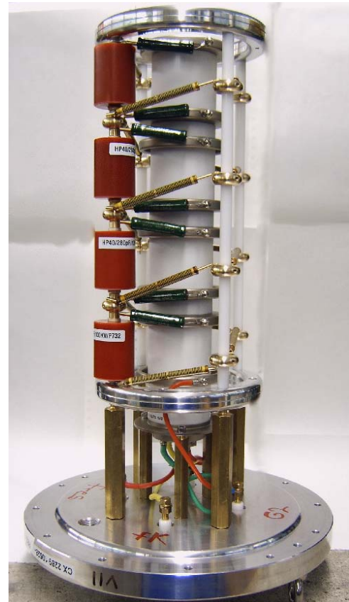
Fig. 8: HV control system for the W7-X gyrotrons: Modulator, crowbar and ignition coil (left) and thyatron tube with new external circuitry for protection of the gyrotron (right).
