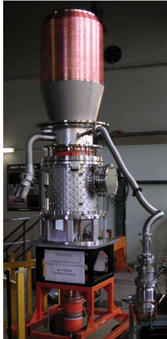
Fig. 1: Photography of the first industrial prototype of the 2 MW, CW, 170 GHz coaxial cavity gyrotron (fabricated by TED).
