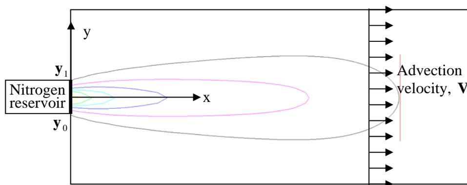
**Figure 7-1-2-1 Two-dimensional advective diffusion of nitrogen into air flow**
