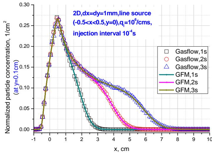
**Figure 7-2-3-3 Advection diffusion from continuous particle line source distributed in advection (x) direction in two-dimensional domain**
