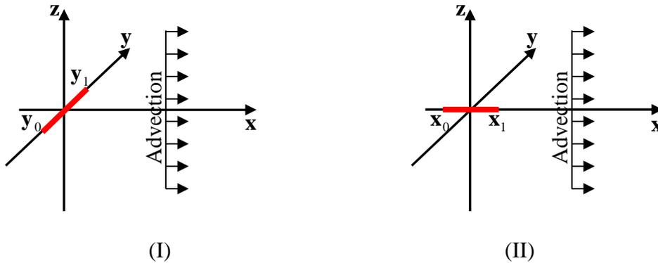
**Figure 7-2-4-1 Two cases of line sources in infinite three-dimensional domain**
