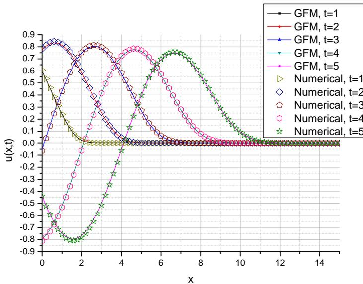
**Figure 4-4-3 Verification of Green's function solution in semi-infinite domain with Robin boundary**
