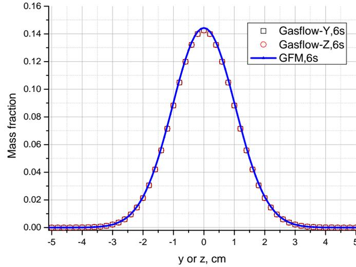
**Figure 7-1-3-3 Mass fraction distributions in transverse directions ( $x = 10$  cm) at  $t = 6$  s (three-dimensional problem)**
