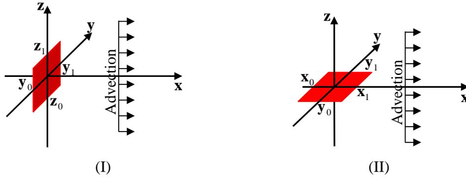
**Figure 7-2-6-1 Area source in infinite three-dimensional domain**
