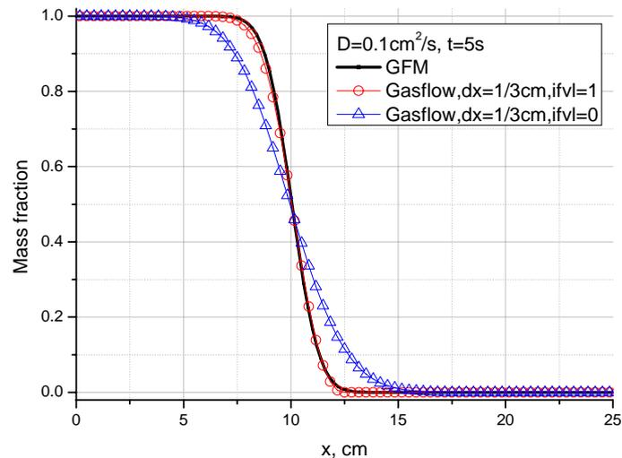
**Figure 7-1-1-2 One-dimensional advective diffusion with  $D = 0.1 \text{ cm}^2/\text{s}$  and different ifvl options**
