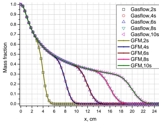
**Figure 7-1-2-3 Mass fraction distributions in advection direction ( $y = 0$  cm) at different times (two-dimensional problem)**
