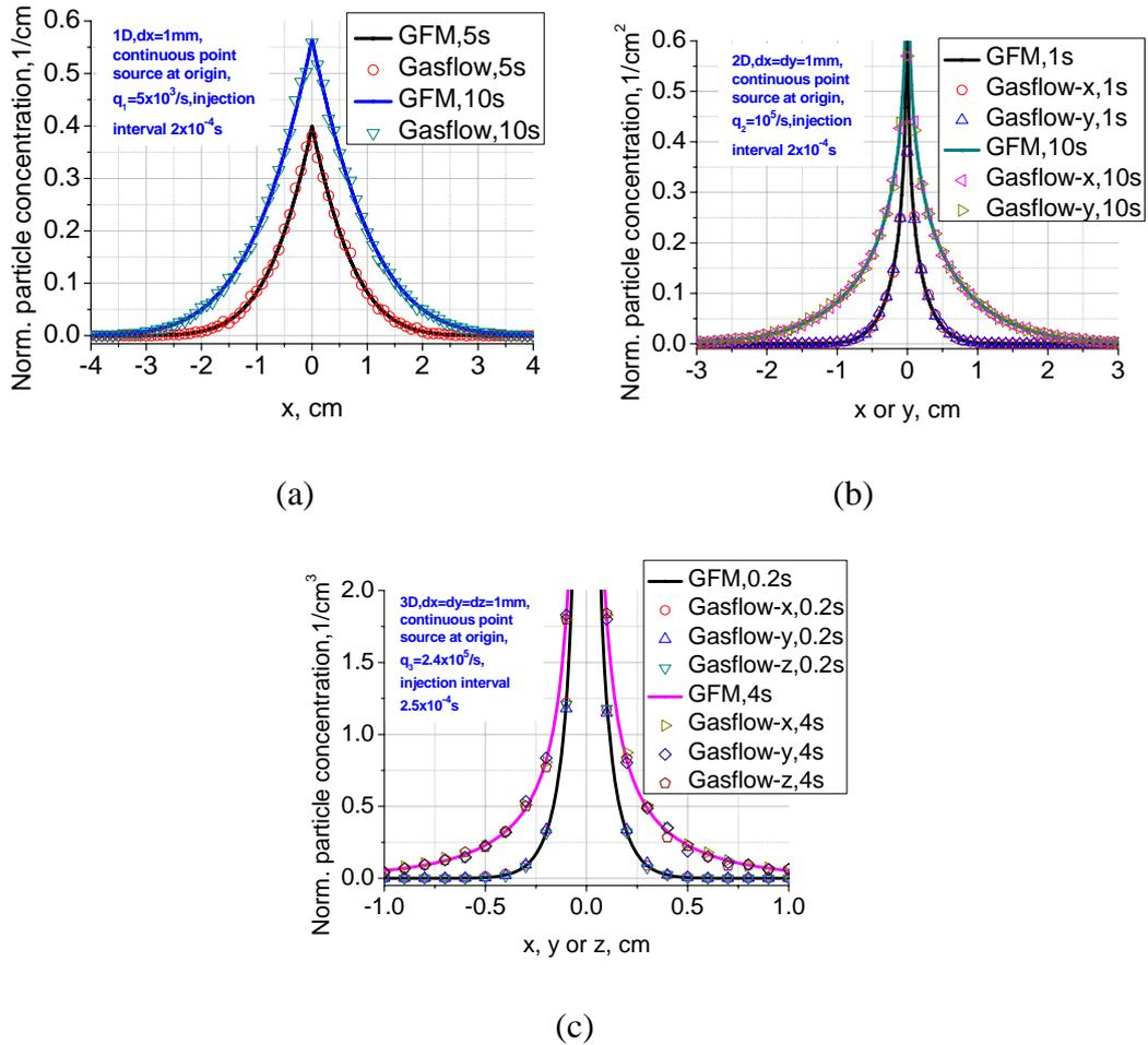
**Figure 7-2-1-2 Particle diffusion from continuous point source in quiescent flows in one-, two- and three-dimension**
