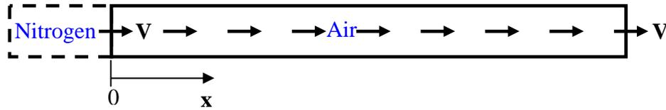
**Figure 7-1-1-1 One-dimensional advective diffusion of nitrogen into air flow**
