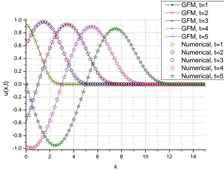
**Figure 4-3-2 Verification of Green's function in semi-infinite domain with Dirichlet boundary condition**
