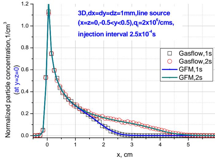
**Figure 7-2-4-2 Advection diffusion from continuous particle line source distributed in transverse (y) direction in three-dimensional domain**
