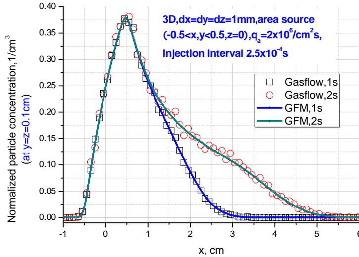
**Figure 7-2-6-3 Advection diffusion from continuous particle area source distributed in  $x - y$  plane in three-dimensional domain**
