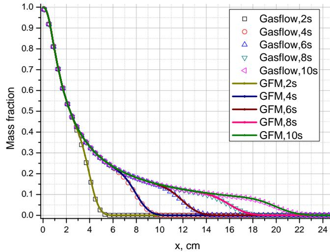
**Figure 7-1-3-2 Mass fraction distributions in advection direction ( $\mathbf{y} = \mathbf{z} = 0 \text{ cm}$ ) at different times (three-dimensional problem)**
