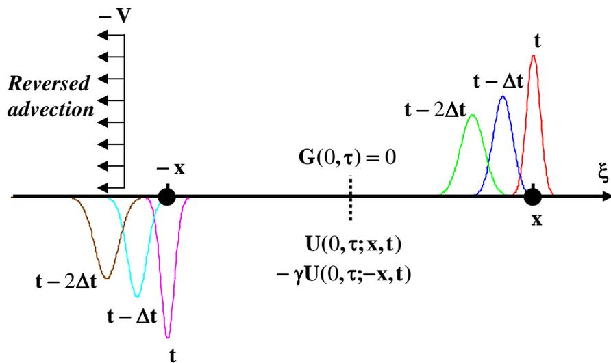
Figure 4-3-1 Schematic image system for advection diffusion problem with Dirichlet boundary condition
