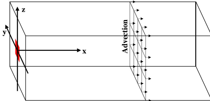
**Figure 7-1-3-1 Three-dimensional advective diffusion of nitrogen into air flow**
