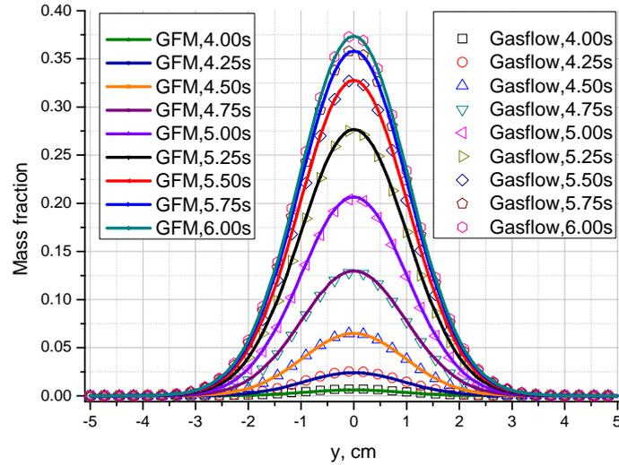
**Figure 7-1-2-4 Mass fraction distributions in transverse direction ( $x = 10$  cm) at different times (two-dimensional problem)**
