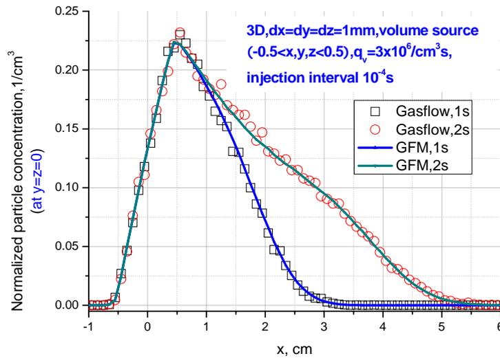
**Figure 7-2-7-2 Advection diffusion from continuous particle volume source in three-dimensional domain**
