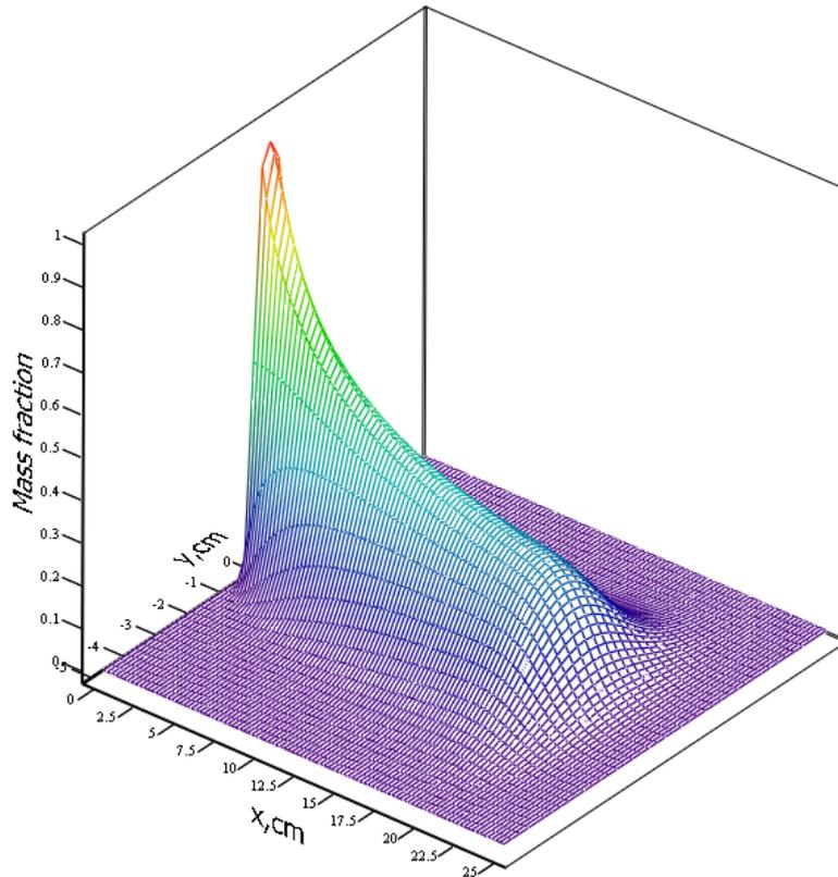
**Figure 7-1-2-2 Three-dimensional view of advection diffusion plume of nitrogen at  $t = 10$  s**
