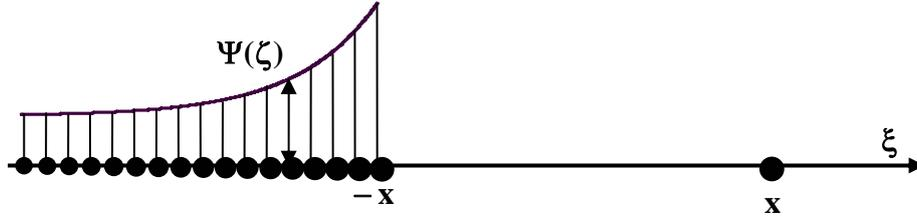
**Figure 4-4-1 Schematic image system for advection diffusion problem with Robin boundary condition**
