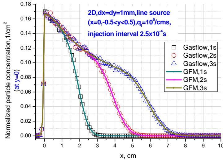
**Figure 7-2-3-2 Advection diffusion from continuous particle line source distributed in transverse ( y ) direction in two-dimensional domain**
