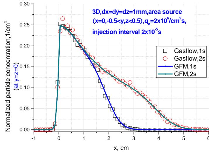
**Figure 7-2-6-2 Advection diffusion from continuous particle area source distributed in transverse ( $y - z$ ) plane in three-dimensional domain**
