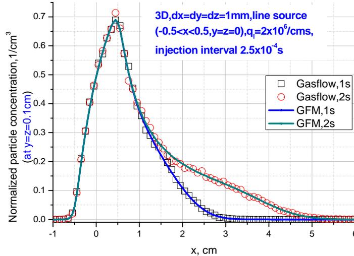
**Figure 7-2-4-3 Advection diffusion from continuous particle line source distributed in advection ( $x$ ) direction in three-dimensional domain**
