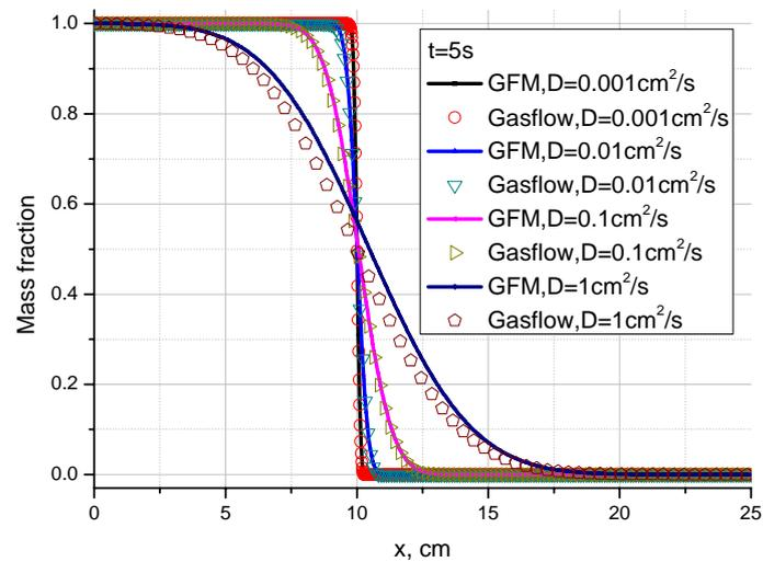
**Figure 7-1-1-4 One-dimensional advective diffusion with different diffusion coefficients**
