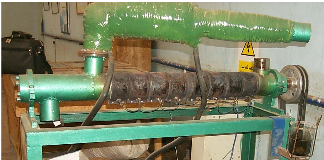
Figure 36: General view of the bench scale facility at the Helwan university, Cairo; screw reactor, electrically heated.
