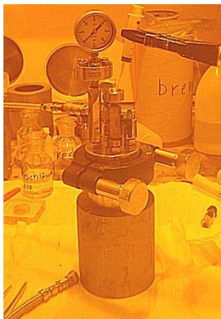
Fig. 1 Corrosion experiment using high pressure autoclave with spent nuclear fuel pellets in NaCl brine containing hydrogen and bromide.
