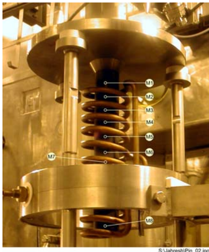
Fig. 3 Temperature monitoring points M1 to M8 along a dummy of the glass pouring pipe for measurements by the thermovision camera. The tests have shown that the MF-power for the VEK-melter must be limited to 25 kW at the MF-Generator in order to not exceed a pouring pipe temperature of 1150°C.
