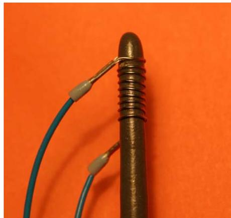
Fig. 6. Thermite igniters and electrical starter
