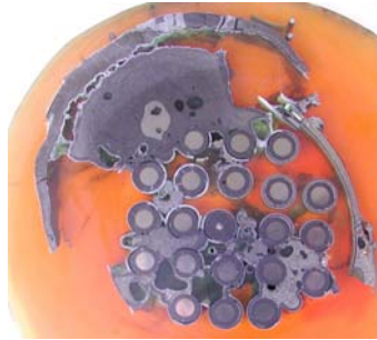
Figure 6.5: Color macro photos of cross sections at 750-850 mm for quantification of material distribution by image analysis.
