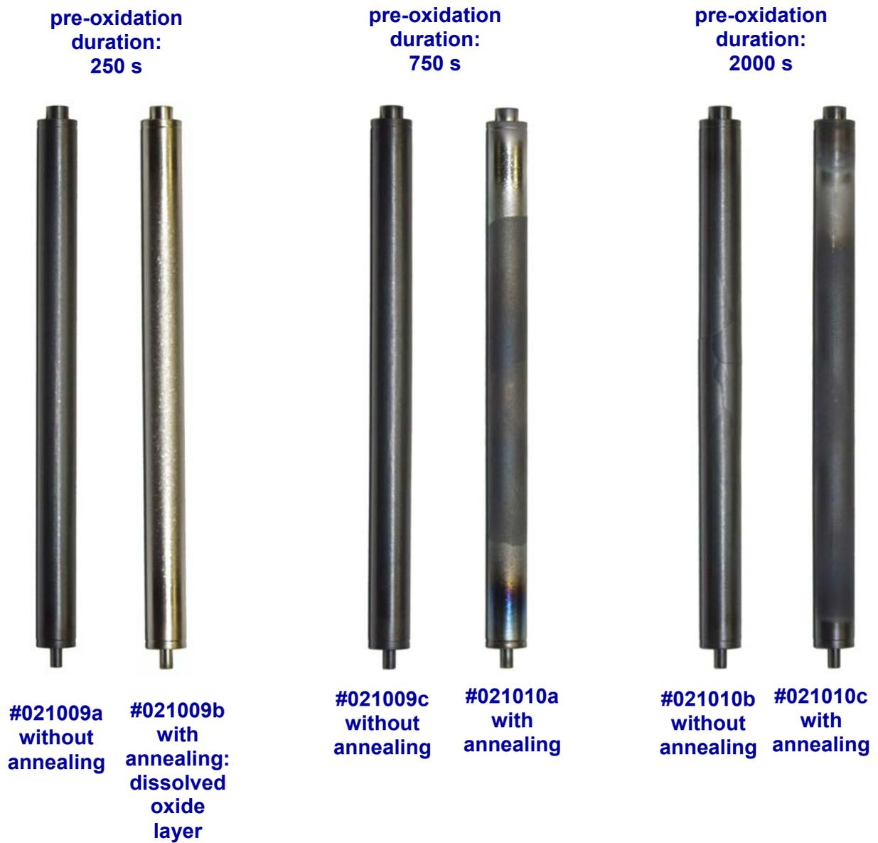
Fig. 5. 2002 experiments in the Quench test rig with different pre-oxidation durations and an annealing time of ~3 h: external view of the Zry-4 claddings pre-oxidised in steam and then annealed in argon at a temperature of ~1475 °C measured with a pyrometer on the cladding surface.
