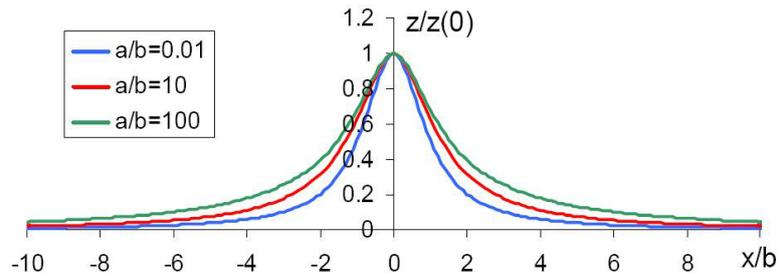
Figure 10: Model of a single bump. The upper curve corresponds to  $a/b = 100$ .
