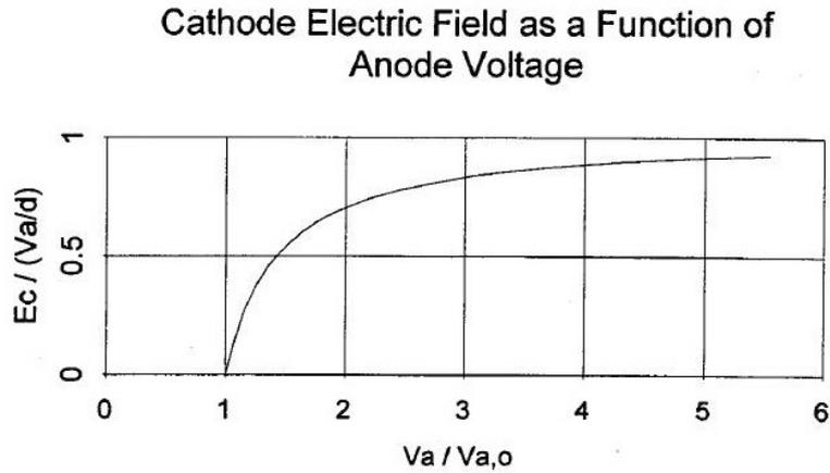
Figure 1: Electric field  $E_c$  normalized to the space-charge free electric field,  $V_a/d$ , as a function of the voltage  $V_a$  on the anode normalized to the voltage  $V_{a,o}$  [from (Amboss 1993)].
