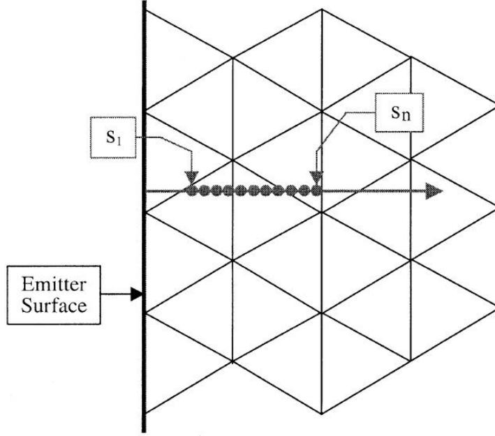
Figure 16: Integration path for the Child–Langmuir law along a surface normal direction on an arbitrary mesh cross section [from (Petillo *et al.* 2002)].
