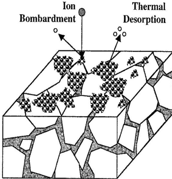
Figure 6: Schematic of cathode surface. The large blocks are tungsten grains of average size  $4.5 \mu\text{m}$ . The separation between pores averages  $6 \mu\text{m}$ , and the pore diameter averages  $2\text{--}3 \mu\text{m}$ . In the “Thermal Desorption” regions barium evaporates from the surface. In the “Ion Bombardment” regions barium is sputtered off [from (Jensen, Lau, and Levush 2000)].
