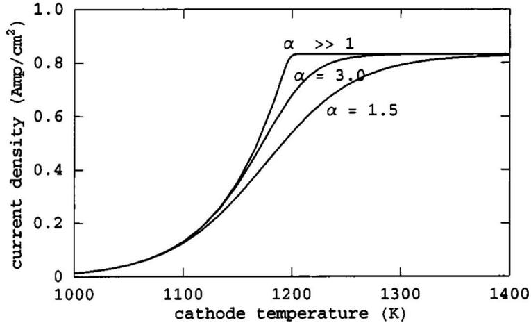
Figure 4: Sensitivity of the emission curve, Eq. (21), to the shape factor  $\alpha$ . The work function and current loading (i.e., the space charge current) are the same for each curve [from (Longo 2003)].
