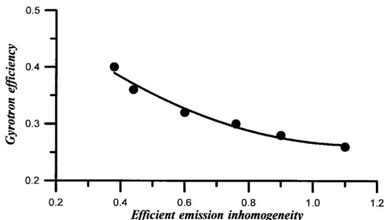
Figure 12: Dependence of the efficiency on the emission nonuniformity measured by the parameter  $\sigma$  which is equal to the standard deviation of the normal distribution  $F(J) = (1/\sqrt{2\pi}\sigma) \exp[-(1-x)^2/2\sigma^2]$  that approximates the measured one [from (Glyavin, Goldenberg, Kufin, Lygin, Postnikova, and Zapevalov 1999)].
