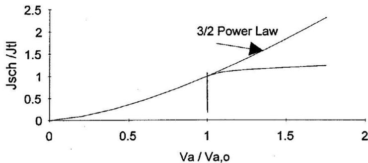
Figure 2: Schottky emission current density  $J_{SCH}$  normalized to the temperature limited emission current density,  $J_{TL}$ , as a function of the normalized anode voltage [from (Amboss 1993)].
