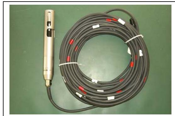
**Figure 5: conductivity/temperature sensor**
