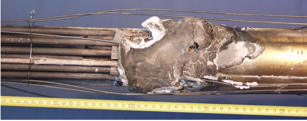
Fig. 31: QUENCH-12; Posttest appearance of the hot zone of shroud and test bundle (~750-1150 mm) at orientations 0, 90, 180, and 270 degrees (from left).
