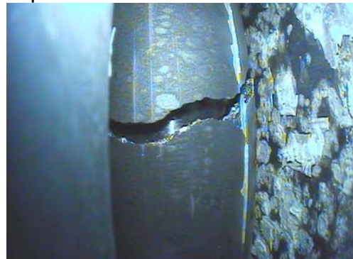
rod16 break at 900 mm
