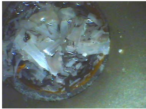
debris inside corner rod guide tube
