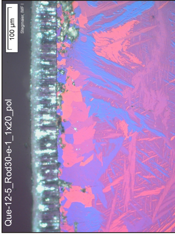
Fig. 73: QUE-12-5, level 750 mm; cladding oxidation of rods 24 and 30 (outer ring, heated).
