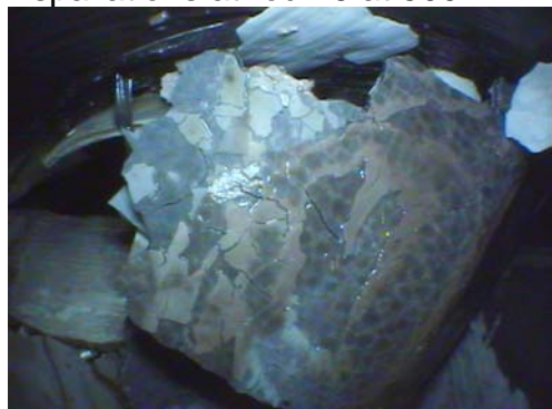
cladding piece on top of 4 th spacer
