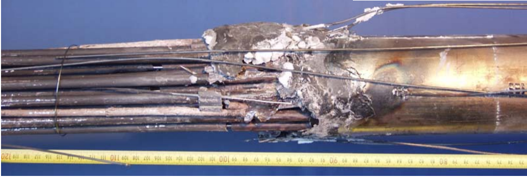
Fig. 31: QUENCH-12; Posttest appearance of the hot zone of shroud and test bundle (~750-1150 mm) at orientations 0, 90, 180, and 270 degrees (from left).
