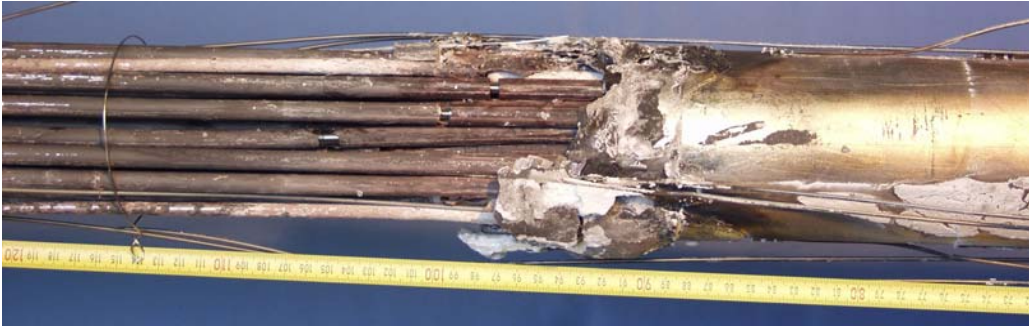
Fig. 31: QUENCH-12; Posttest appearance of the hot zone of shroud and test bundle (~750-1150 mm) at orientations 0, 90, 180, and 270 degrees (from left).
