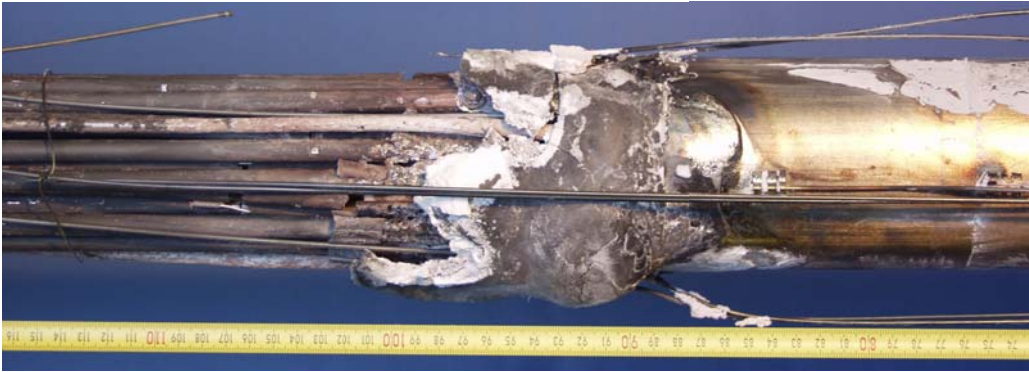
Fig. 31: QUENCH-12; Posttest appearance of the hot zone of shroud and test bundle (~750-1150 mm) at orientations 0, 90, 180, and 270 degrees (from left).
