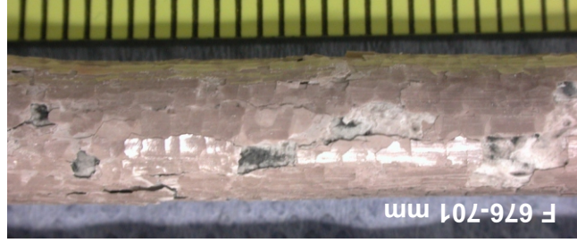
Fig. 119: QUE-12, level 700 mm; oxidation of withdrawn corner rod F, representing the state just before quenching.
