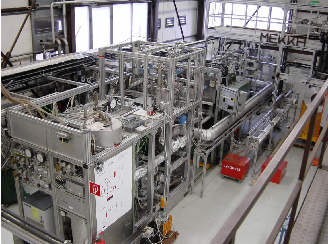
Figure 14: View on the liquid-metal NaK loop in the MEKKA laboratory.
