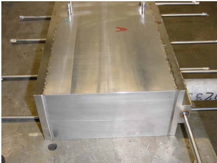
Figure 9: Module during welding. The vertical wall in the foreground of the picture is already welded, the upper walls are fixed.
