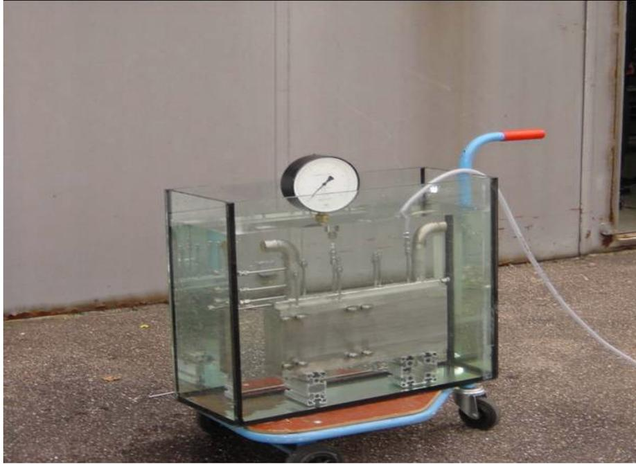
Figure 10: MHD mock-up submersed in water for leak and pressure tests.
