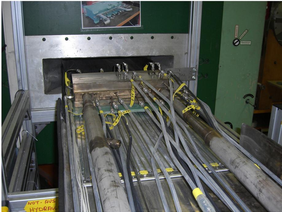
Figure 20: Connection of pressure taps with pressure transducers through rigid pipes of stainless steel. The pipes are externally insulated by flexible silicon tubes to avoid that a contact with metallic structures creates a short circuit already close to the test section.
