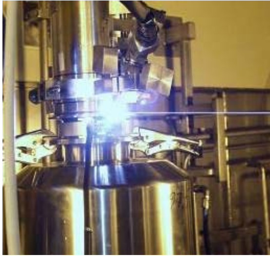
Fig. 5: Lid-welding of glass canister
