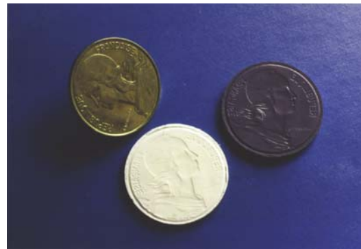
Fig.7: ZircoDur®-replicas of a coin (upper left) by embossing showing the green body (upper right) and the sintered part (bottom).
