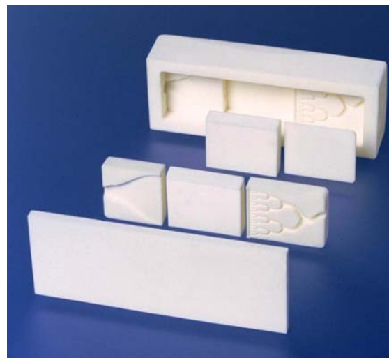
Fig. 17: Modular Al 2 O 3 micro reactor system with exchangeable components made by RPPC [59]
