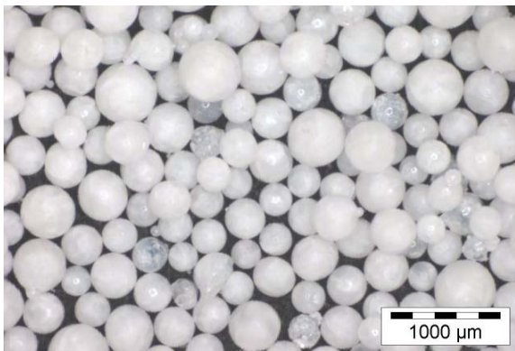
Fig. 4: Lithium orthosilicate pebbles with sizes of 250-630 \mu\text{m} fabricated by melt-spraying.
