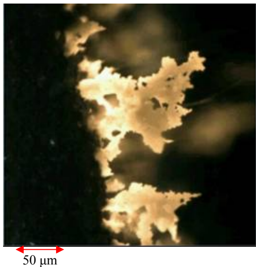
Fig. 9: nAl based propellant aggregate (SPLab, Maggi)
