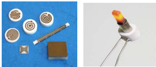
Fig. 5: Types of ceramic microheaters: screen printed patterns on ceramic substrates (left), heating plug in operation at about 1200°C (right)
