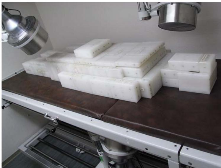
Abb. 6-38: P5 phantom in modified configuration with only the NaI(Tl) detectors
