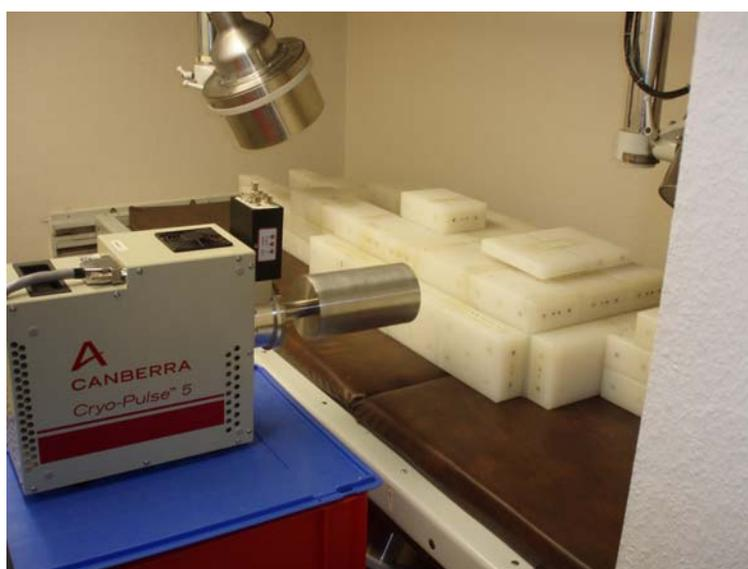
Abb. 6-39: Placement of the second germanium detector
