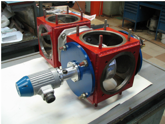
Fig. 1: Target system with step-wise electromotor for rotation of degrader wheel.
