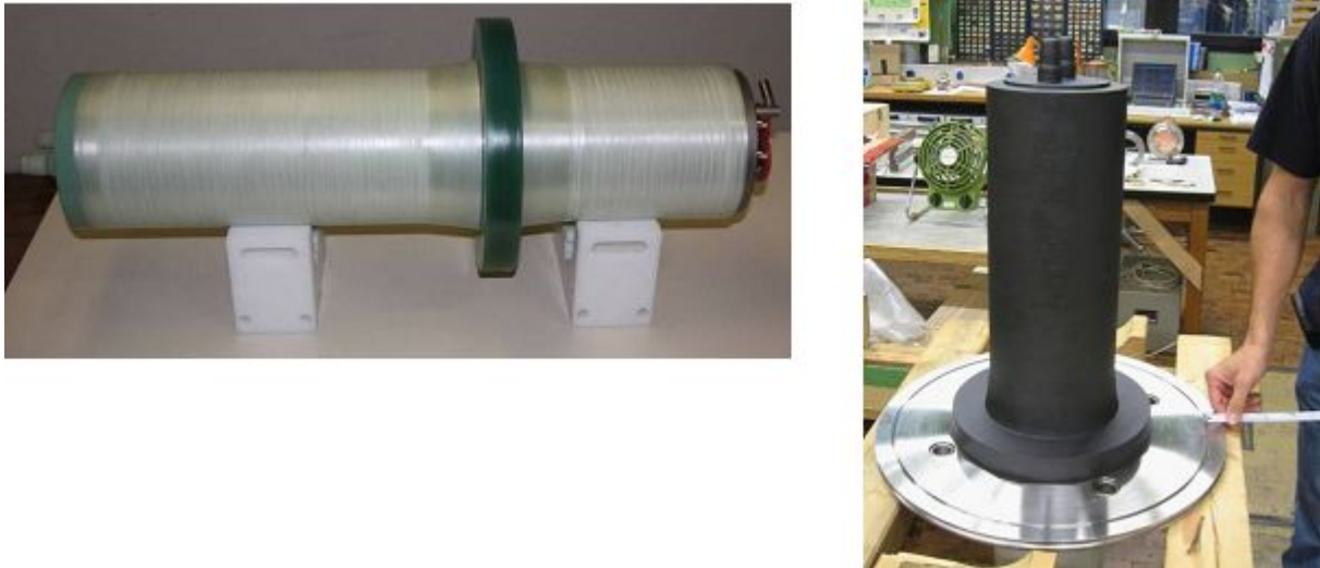
Fig. 2: HV-insulation mock-up - left: glas/G10 insulation, right: mock-up covered with conductive paint.
