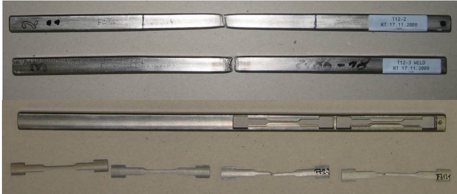
Fig. 3: Conductor samples and machined flat specimens after test.
