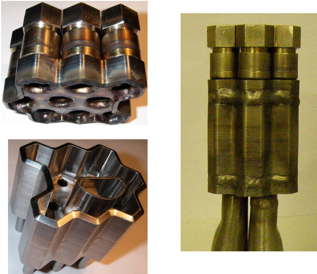
Fig. 6: Final assembly and TIG welding of the 9-finger module parts.
