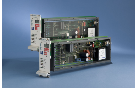
Fig. 1: Quench Detector UNIQD IPE 3410 (sealed / unsealed).
