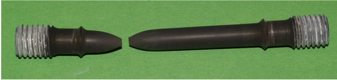
Fig. 2: EUROFER 97 creep specimen after 35,688 hours (4 years) at 600 °C. For the ageing study only the screw heads are used, since they are un-strained.
