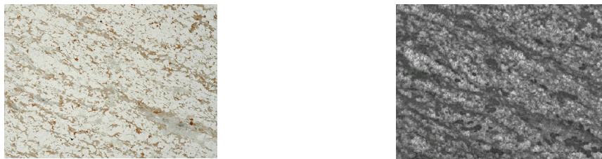
Figure 1: The photograph (left) and Am-241 autoradiography (right) images of the thin rock sections (mica gneiss) B6.
