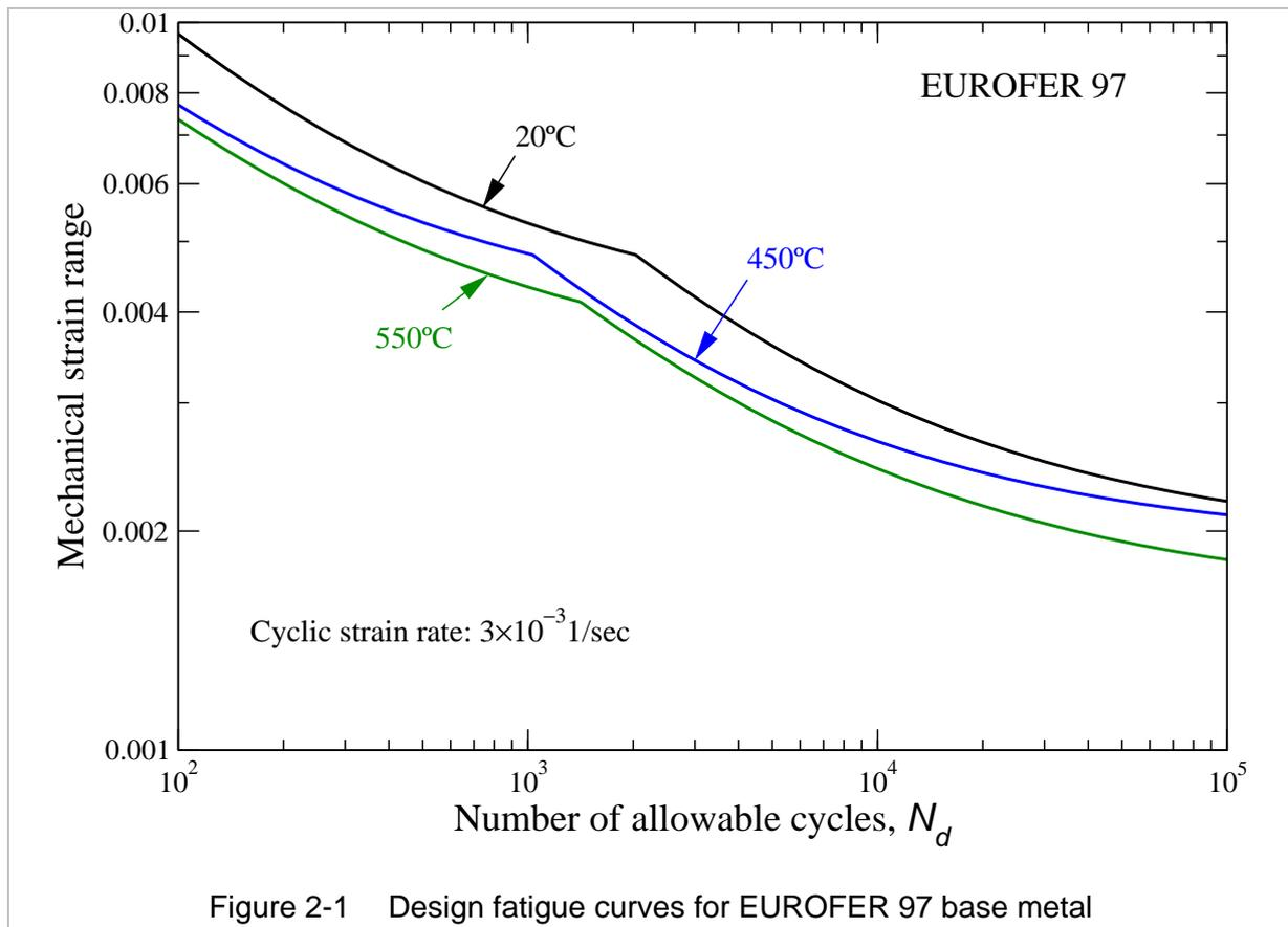
Figure 2-1 Design fatigue curves for EUROFER 97 base metal
