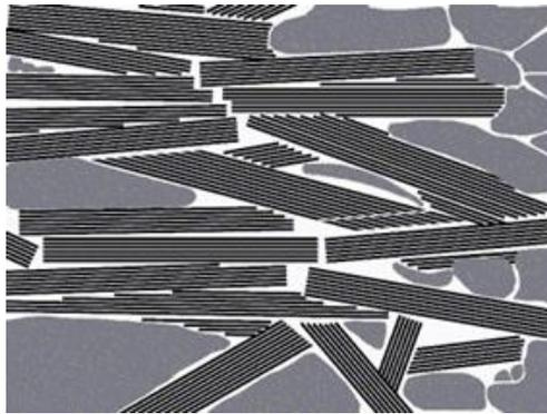
*Fig. 3. An example of clay (elongated particles) and quartz grains (gray area) distribution in the full scale simulations. The solution accessible pore space is shown as white area.*
