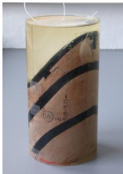
*Fig. 1. Sandstone drilling core consisting of heterogeneous material, pervaded by several material boundaries and fissures and prepared for column experiments.*
