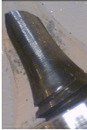
Fig. 9-16 Photographs (Macro) of the tensile tested ADS 4 specimens: A4 01 ( T_{\text{rest}} = 250^{\circ}\text{C} ), A4 02 ( 300^{\circ}\text{C} ), A4 03 ( 350^{\circ}\text{C} )
