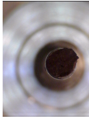
Fig. 9-12 Photographs (Macro) of the tensile tested F82H mod. specimens: F 10 ( T_{\text{test}} = 300^{\circ}\text{C} ), F 11 ( 300^{\circ}\text{C} ), F 12 ( 350^{\circ}\text{C} )
