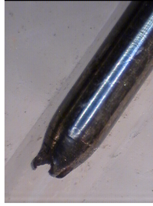
Fig. 9-13 Photographs (Macro) of the tensile tested OPTIFER IVc specimens: OT 06 ( T_{\text{test}} = 250^{\circ}\text{C} ), OT 07 ( 300^{\circ}\text{C} ), OT 08 ( 350^{\circ}\text{C} )
