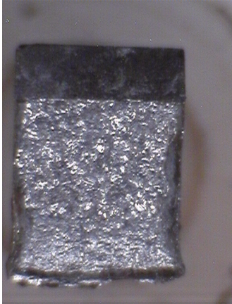
Fig. 8-27 Tested impact specimens F 01, F 02, F 03 after testing (Macro) and after complete breaking (Macro)
