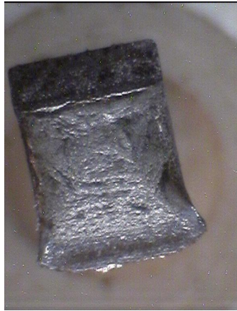
Fig. 8-33 Tested impact specimens A3 08, A3 09, A3 10 after testing (Macro) and after complete breaking (Macro)
