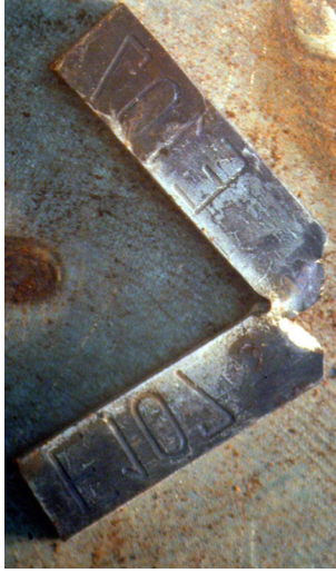
Fig. 8-23 Tested impact specimen E1 07 after testing (Macro) and after complete breaking (SEM)
