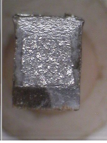
Fig. 8-28 Tested impact specimens F 04, F 05, F 06 after testing (Macro) and after complete breaking (Macro)
