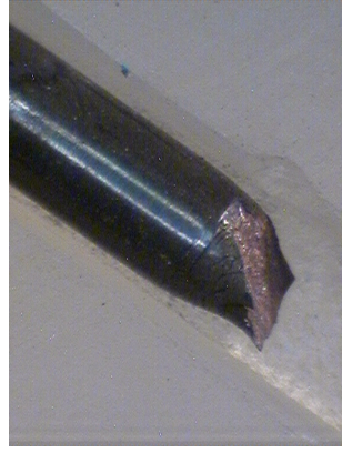
Fig. 9-15 Photographs (Macro) of the tensile tested ADS 3 specimens: A3 09 ( T_{\text{rest}} = 250^{\circ}\text{C} ), A3 10 ( 300^{\circ}\text{C} ), A3 11 ( 350^{\circ}\text{C} )
