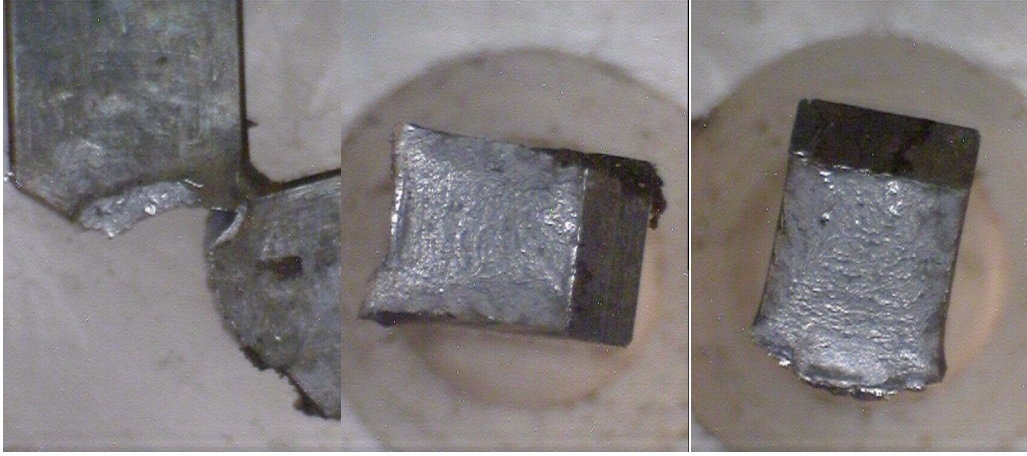
Fig. 8-42 Tested impact specimens C 165, C 166, C 167 after testing (Macro) and after complete breaking (Macro)
