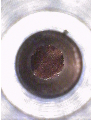
Fig. 9-16 Photographs (Macro) of the tensile tested ADS 4 specimens: A4 01 ( T_{\text{rest}} = 250^{\circ}\text{C} ), A4 02 ( 300^{\circ}\text{C} ), A4 03 ( 350^{\circ}\text{C} )
