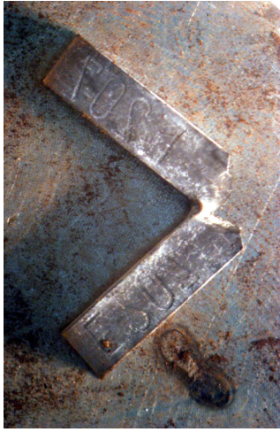
Fig. 8-26 Tested impact specimen E2 07 after testing (Macro) and after complete breaking (SEM)
