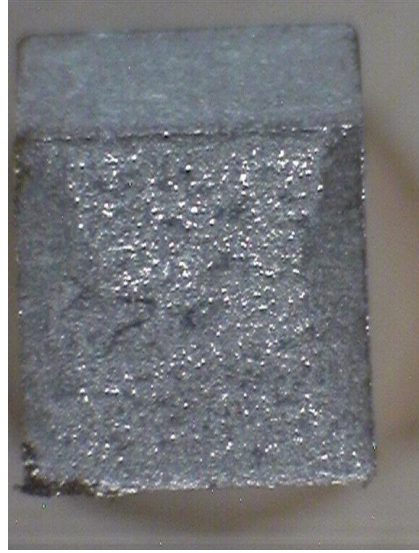
Fig. 8-35 Tested impact specimens A4 01, A4 02, A4 03 after complete breaking (Macro)
