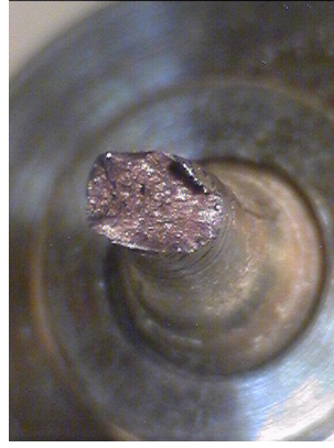
Fig. 9-12 Photographs (Macro) of the tensile tested F82H mod. specimens: F 10 ( T_{\text{test}} = 300^{\circ}\text{C} ), F 11 ( 300^{\circ}\text{C} ), F 12 ( 350^{\circ}\text{C} )
