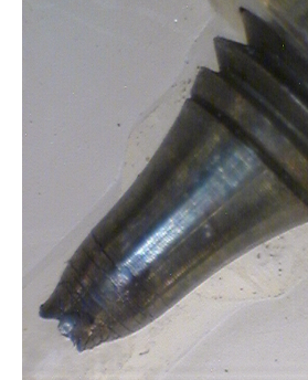
Fig. 9-10 Photographs (Macro) of the tensile tested EUROFER 97 ANL specimens: E1 15 ( T_{rest} = 250^{\circ}\text{C} ), E1 16 ( 300^{\circ}\text{C} ), E1 17 ( 350^{\circ}\text{C} )
