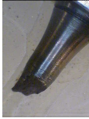
Fig. 9-14 Photographs (Macro) of the tensile tested ADS 2 specimens: A2 09 ( T_{\text{test}} = 250^{\circ}\text{C} ), A2 10 ( 300^{\circ}\text{C} ), A2 11 ( 350^{\circ}\text{C} )
