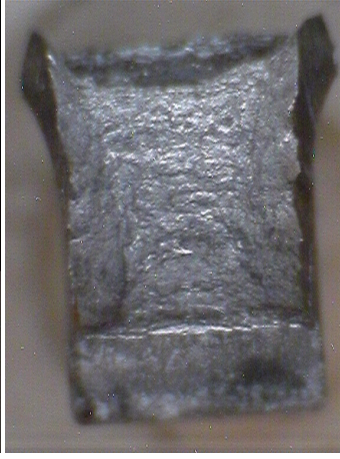
Fig. 8-32 Tested impact specimens A2 11, A2 12 after testing (Macro) and after complete breaking (Macro)
