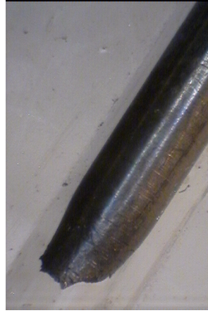
Fig. 9-12 Photographs (Macro) of the tensile tested F82H mod. specimens: F 10 ( T_{\text{test}} = 300^{\circ}\text{C} ), F 11 ( 300^{\circ}\text{C} ), F 12 ( 350^{\circ}\text{C} )
