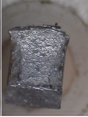
Fig. 8-28 Tested impact specimens F 04, F 05, F 06 after testing (Macro) and after complete breaking (Macro)
