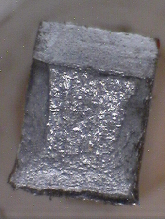
Fig. 8-32 Tested impact specimens A2 11, A2 12 after testing (Macro) and after complete breaking (Macro)
