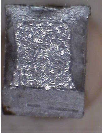
Fig. 8-31 Tested impact specimens A2 08, A2 09, A2 10 after testing (Macro) and after complete breaking (Macro)
