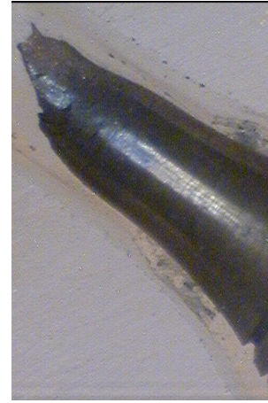
Fig. 9-15 Photographs (Macro) of the tensile tested ADS 3 specimens: A3 09 ( T_{\text{rest}} = 250^{\circ}\text{C} ), A3 10 ( 300^{\circ}\text{C} ), A3 11 ( 350^{\circ}\text{C} )
