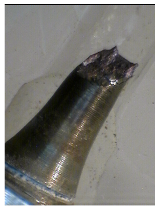
Fig. 9-12 Photographs (Macro) of the tensile tested F82H mod. specimens: F 10 ( T_{\text{test}} = 300^{\circ}\text{C} ), F 11 ( 300^{\circ}\text{C} ), F 12 ( 350^{\circ}\text{C} )
