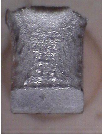
Fig. 8-31 Tested impact specimens A2 08, A2 09, A2 10 after testing (Macro) and after complete breaking (Macro)
