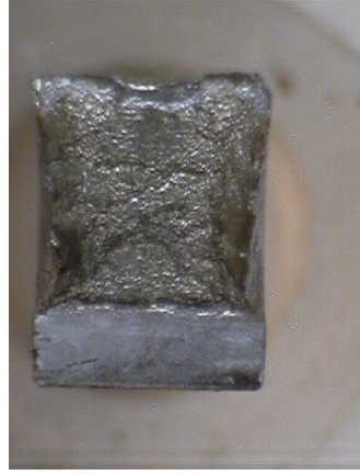
Fig. 8-27 Tested impact specimens F 01, F 02, F 03 after testing (Macro) and after complete breaking (Macro)
