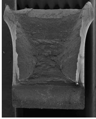
Fig. 8-21 Tested impact specimens E1 01, E1 02, E1 03 after testing (Macro) and after complete breaking (SEM)
