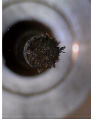
Fig. 9-17 Photographs (Macro) of the tensile tested EURODSHIP specimens: EO 10 ( T_{\text{test}} = 250^{\circ}\text{C} ), EO 12 ( 300^{\circ}\text{C} ), EO 15 ( 350^{\circ}\text{C} )
