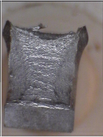
Fig. 8-29 Tested impact specimens OT 01, OT 02, OT 03 after testing (Macro) and after complete breaking (Macro)
