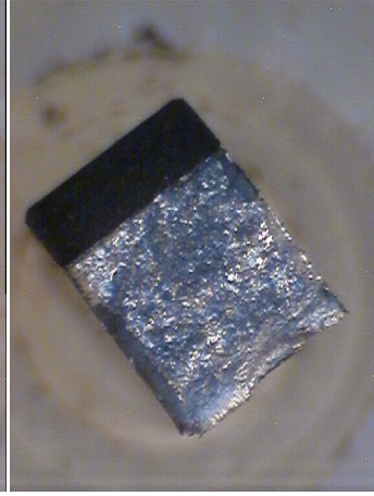
Fig. 8-45 Tested impact specimens C 177, C 170, C 175(6) after testing (Macro) and after complete breaking (Macro)
