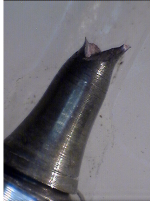
Fig. 9-11 Photographs (Macro) of the tensile tested EUROFER 97 WB specimens: E2 15 ( T_{\text{test}} = 250^{\circ}\text{C} ), E2 16 ( 300^{\circ}\text{C} ), E2 17 ( 350^{\circ}\text{C} )
