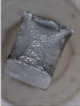
Fig. 8-33 Tested impact specimens A3 08, A3 09, A3 10 after testing (Macro) and after complete breaking (Macro)
