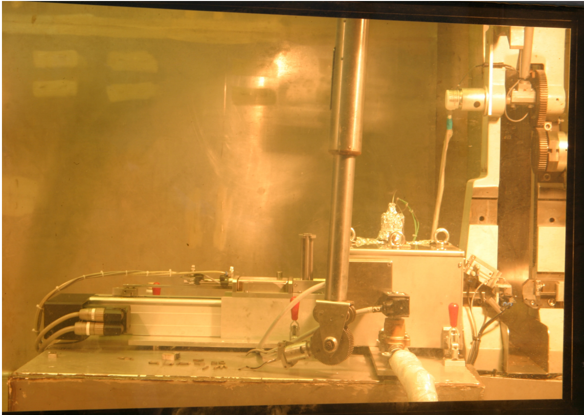
Fig. 3-2 Instrumented impact testing facility with transporting system, cooling facility/furnace and specimen positioning system implemented in the hot cells of RIAR
