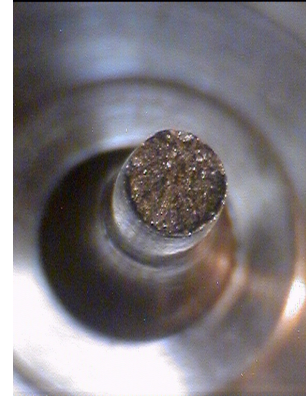
Fig. 9-17 Photographs (Macro) of the tensile tested EURODSHIP specimens: EO 10 ( T_{\text{test}} = 250^{\circ}\text{C} ), EO 12 ( 300^{\circ}\text{C} ), EO 15 ( 350^{\circ}\text{C} )
