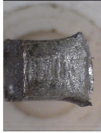
Fig. 8-31 Tested impact specimens A2 08, A2 09, A2 10 after testing (Macro) and after complete breaking (Macro)
