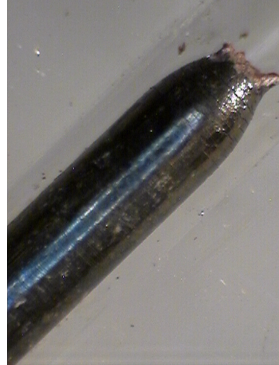
Fig. 9-10 Photographs (Macro) of the tensile tested EUROFER 97 ANL specimens: E1 15 ( T_{rest} = 250^{\circ}\text{C} ), E1 16 ( 300^{\circ}\text{C} ), E1 17 ( 350^{\circ}\text{C} )
