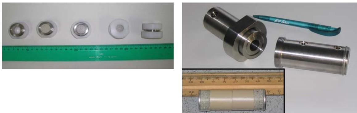
**Figure 2-19:** (left) Reactor of the CIEMAT setup in different assembly stages. The bentonite pellet is squeezed into a stainless-steel cylinder by two filter plates. (right) Stainless steel reactor version of the KIT-INE experimental setup. Two bentonite pellets with the PEEK spacer and the filter plates are inserted.
