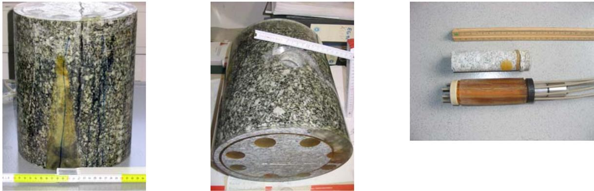
**Figure 2-30:** Preparation of the core from the Grimsel test site, Switzerland, for the transport experiments. At the surface of the core epoxy resin is used as sealing material (a). Afterwards both ends were cut and a borehole was drilled in the middle of the core with a 90° angle to the fracture zone (b). The packer system and drilled core from the location where the packer system is placed into the Grimsel core (c).
