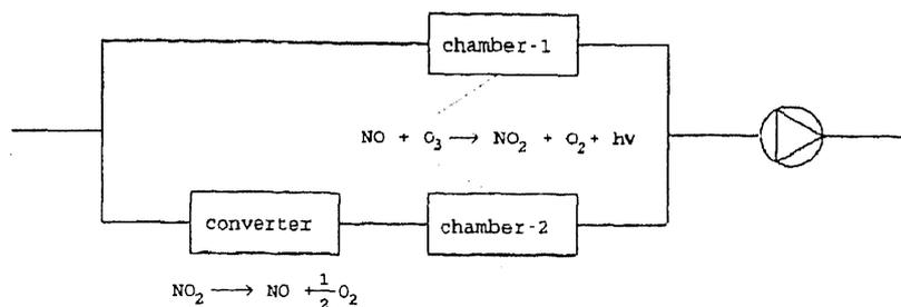
Fig. 2: Measuring Scheme of NO- and NO<sub>2</sub>-Concentrations in the NO<sub>x</sub>-instrument
