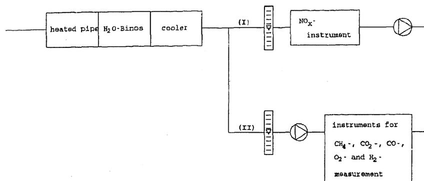
Fig.1: Sampling system for gas concentration measurement
