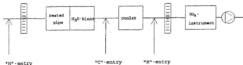
Fig. 12: Flowsheet for gas entry at different position of the sampling system
