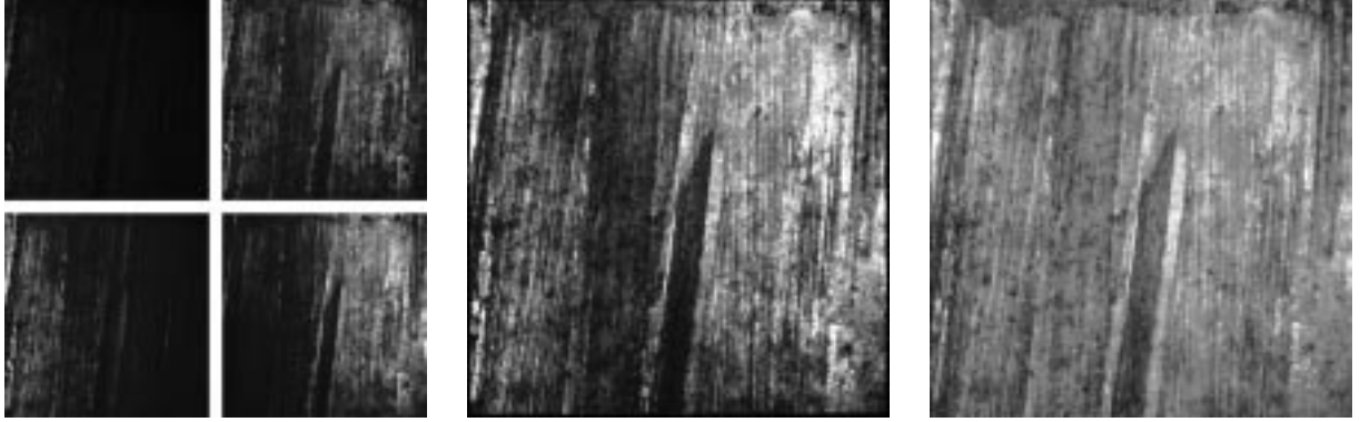
Figure 4. Bullet: a) illumination series (images 10, 15, 20, and 25); b) fusion result (criterion C : variance in a 3 \times 3 -mask; smoothing of \tilde{\theta}(\bar{x}) with a binomial filter of size 49 \times 49 ); c) diffuse lighting.
