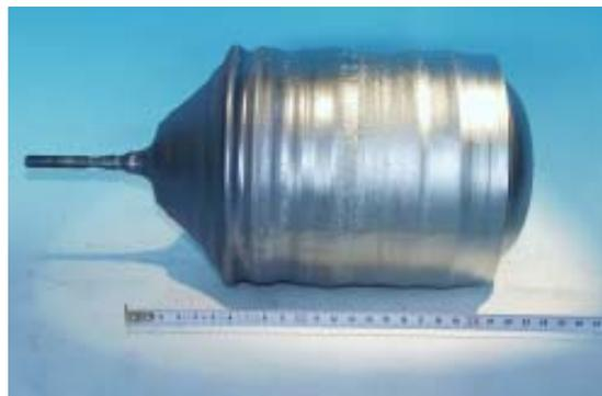
**Figure #14:** Freiberger GaAs crystal (source: <http://www.fcm-germany.com/>).
