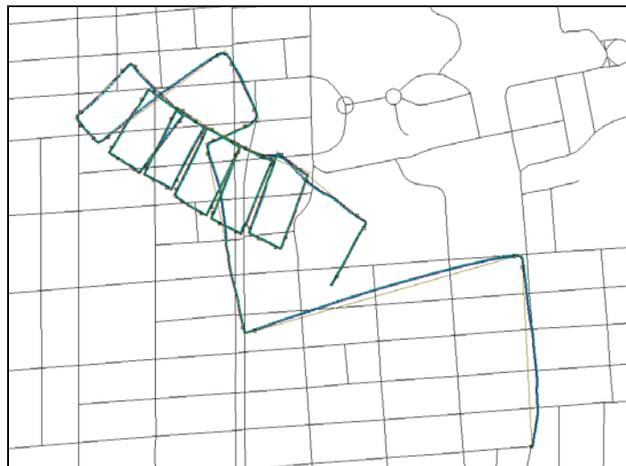
Figure 5-1: Path obtained by adding relative steps overlaid on top of a digital road map. During the first few hundred meters, the path follows the road map; the longer the driving, the more the path separates from the map, and it is finally completely off the real road.
