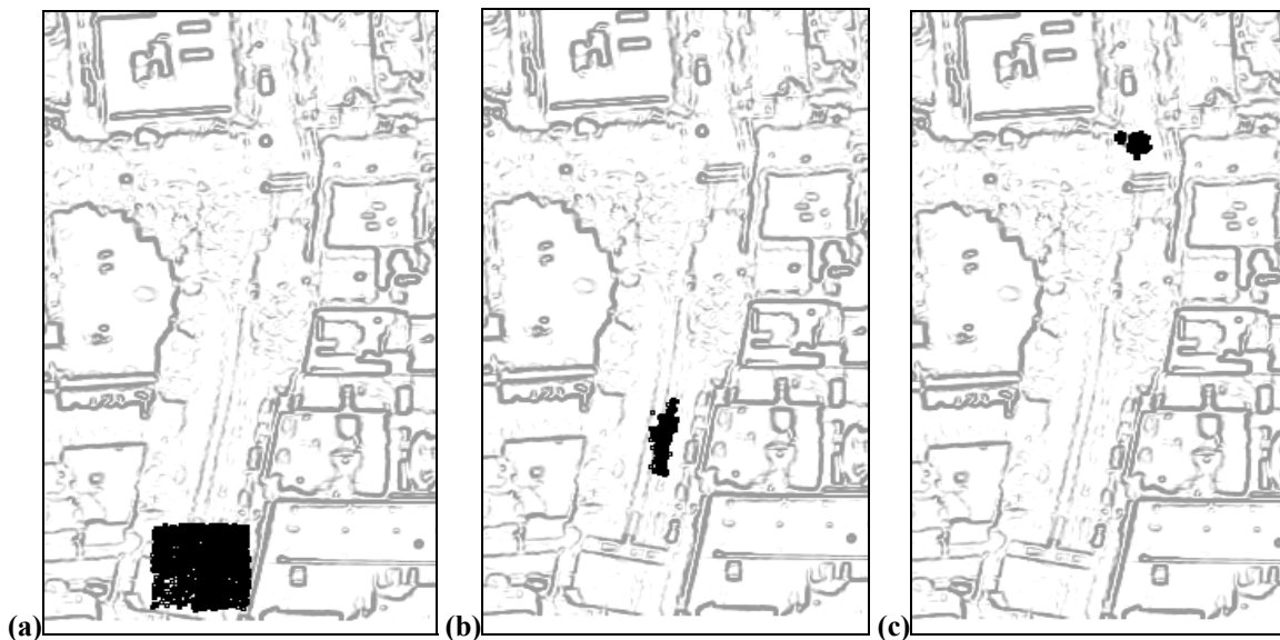
Figure 8-7: Sets of particles (black) overlaid over aerial edge map (gray) (a) Initial uniform distribution S_0 ; (b) set S_{30} after 30 iterations of motion and perception; (c) set S_{100} after 100 iterations of motion and perception.
