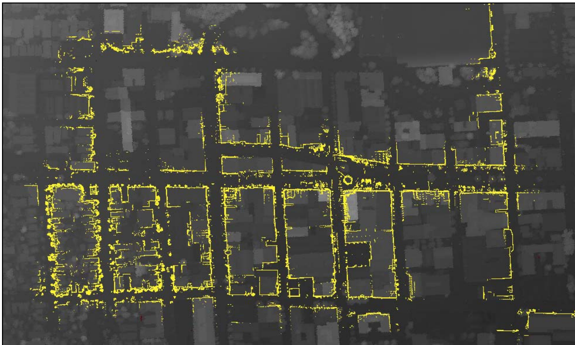
Figure 8-15: Horizontal scan points for corrected path superimposed on top of the DSM.
