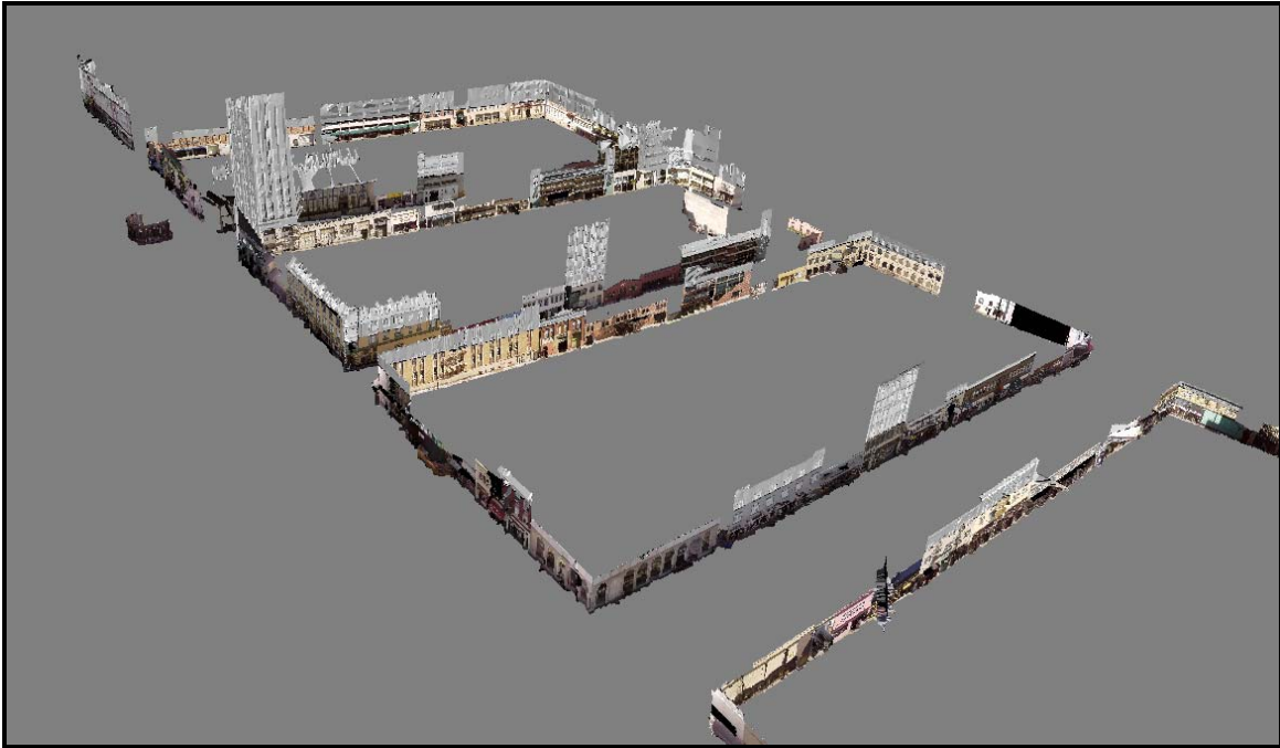
Figure 8-22: Bird's eye view on the texture mapped facade models for the downtown blocks
