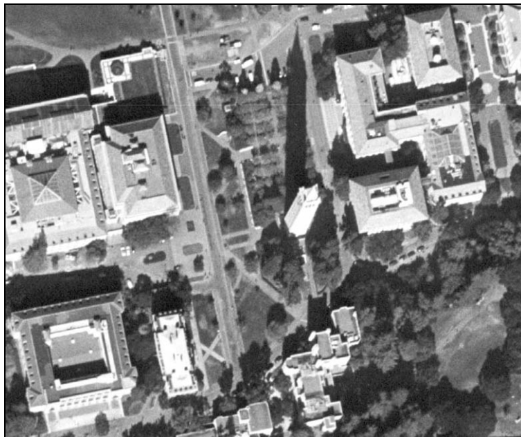
Figure 5-2: Perspective shift for the 92-meter Berkeley campanile (Sather Tower) and surrounding lower buildings
