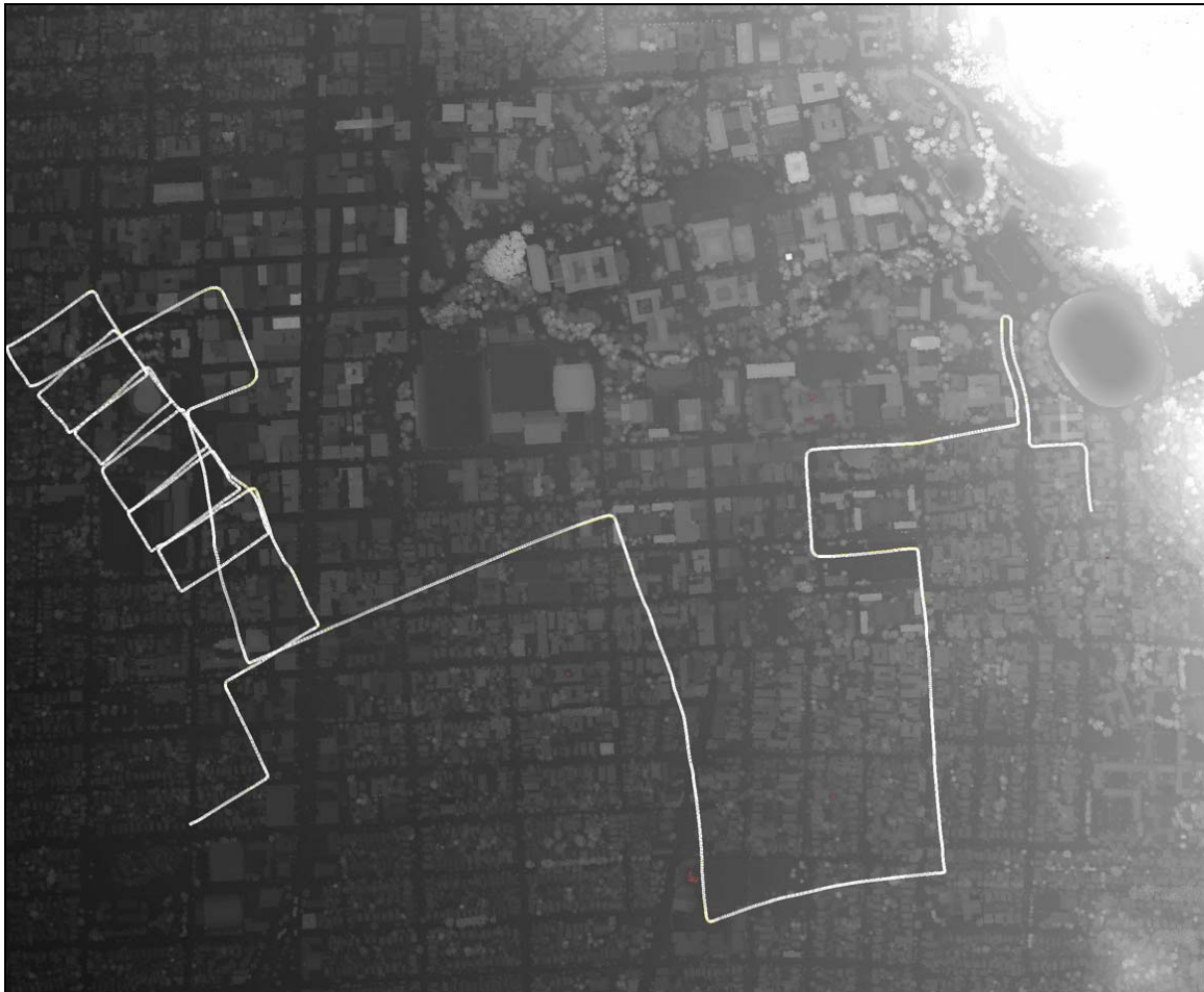
Figure 8-3: Path computed by concatenating relative pose estimates obtained in the scan-to-scan matching process, superimposed on top of the DSM
