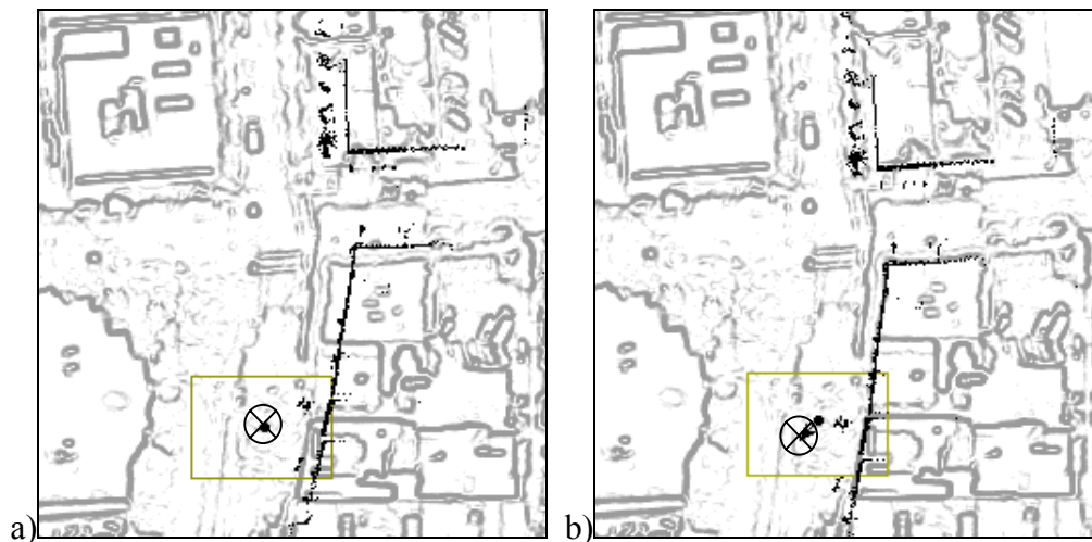
Figure 5-7: Edge image with (a) scan superimposed from pose (x_a, y_a, \theta_a) , with c(x_a, y_a, \theta_a) = 0.377 ; (b) at pose (x_b, y_b, \theta_b) , with c(x_b, y_b, \theta_b) = 0.527 , optimally matching the airborne edge map
