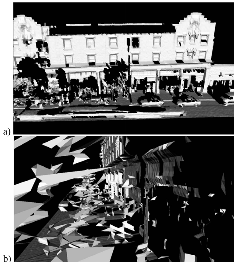
Figure 6-2: Triangulated raw points; (a) front view; (b) side view.
