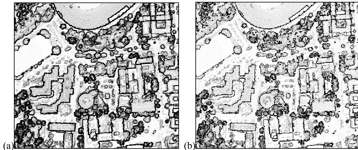
Figure 5-5: Edge map obtained from DSM with (a) Sobel filter, (b) proposed alternative discontinuity filter
