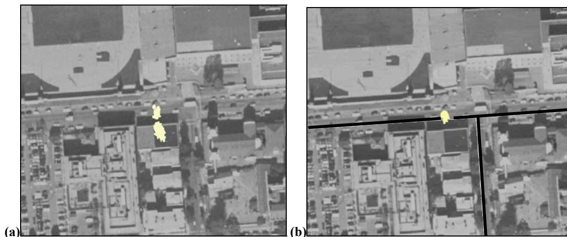
Figure 8-8: Restricting particles to locations near roads; belief computed with (a) N=200,000 particles without restrictions, (b) N=10,000 particles restricted within a 25 meter wide strip around the roadmap (black)
