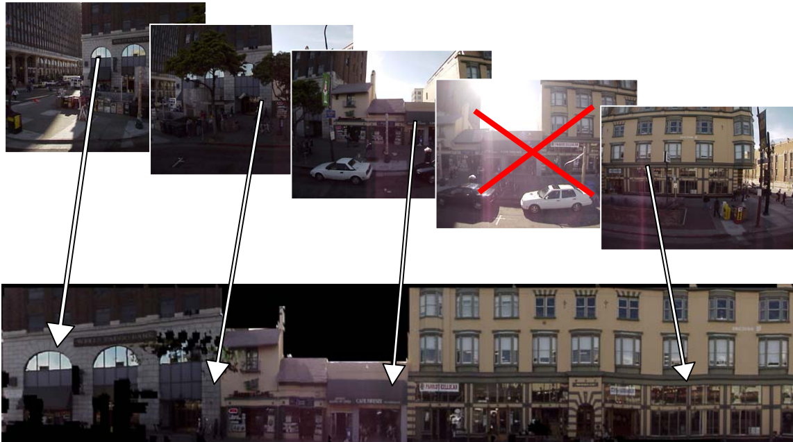
Figure 6-18: Automatic texture atlas generation. Texture triangles from various pictures are assembled to one single artificial image. One image has been prohibited for texture mapping due to over-saturation of the camera; for the others, the arrows illustrate the process of copying triangles.
