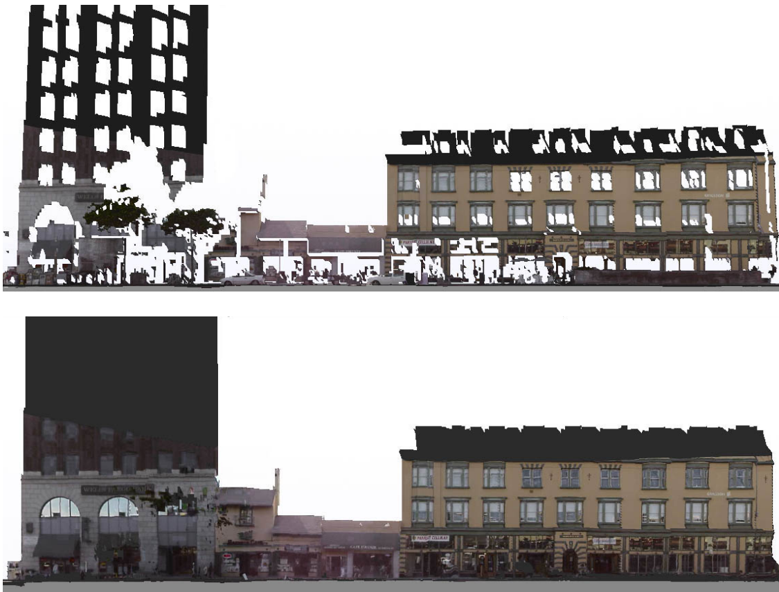
Figure 8-19: Textured facade mesh without (top) and with (bottom) processing.
