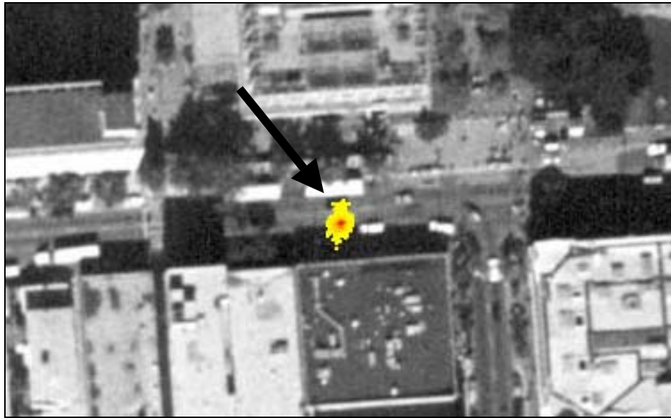
Figure 5-12: Set of particle representing the pose belief, superimposed on the aerial image. In this visualization, the probability density is expressed by different colors.
