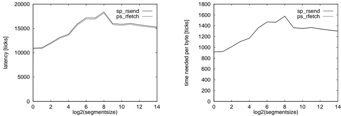
These pictures show how long it takes on the MP-1 to send or fetch a 1-byte packet (latency time, left picture) and 1 additional byte in a large packet (right picture), depending on the size size of the machine segments, when each processor sends/fetches one packet to/from a random target processor in the same nice-rectangular machine segment.
