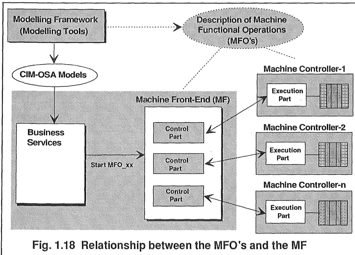
Fig. 1.18 Relationship between the MFO's and the MF
