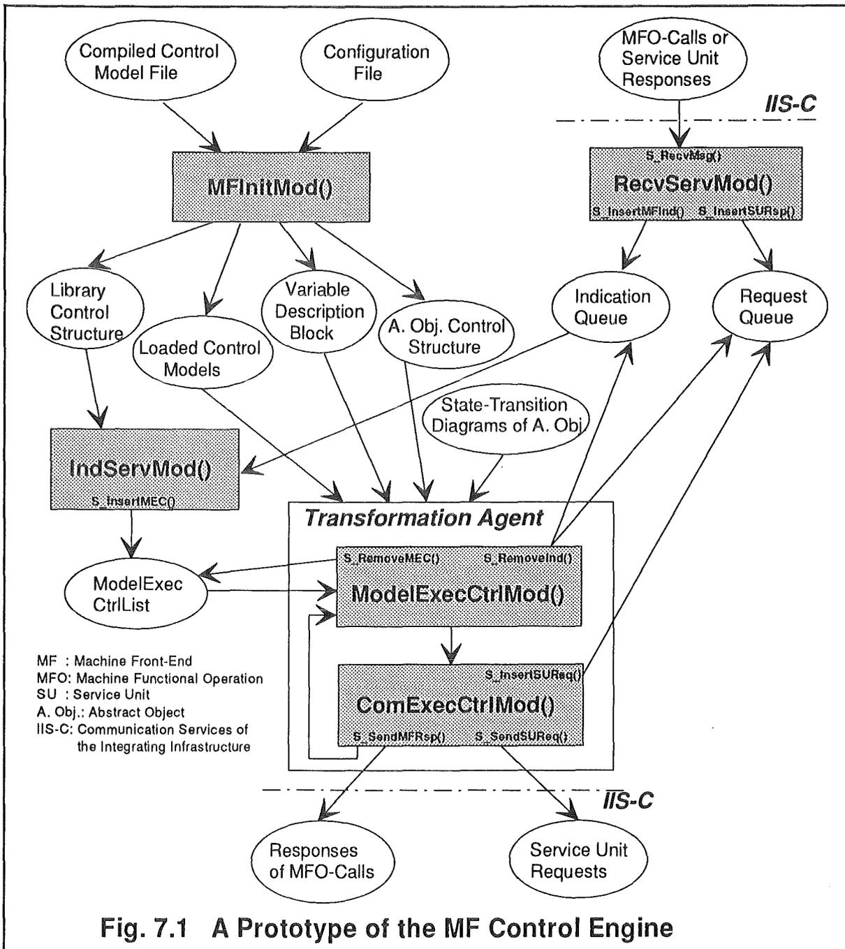
The 'ModelExecCtrlList' contains a list of control records. Each control record holds information for the processing of a Control Model for a specified MFO execution. These control records are initiated by the *Indication Service Module, IndServMod()*, and used by the *Transformation Agent*. Within the processing of a Control Model the Transformation Agent may send requests to the underlying *Service Unit Provider* for controlling the MFO execution at the MF-Server. As soon as a Control Model is
