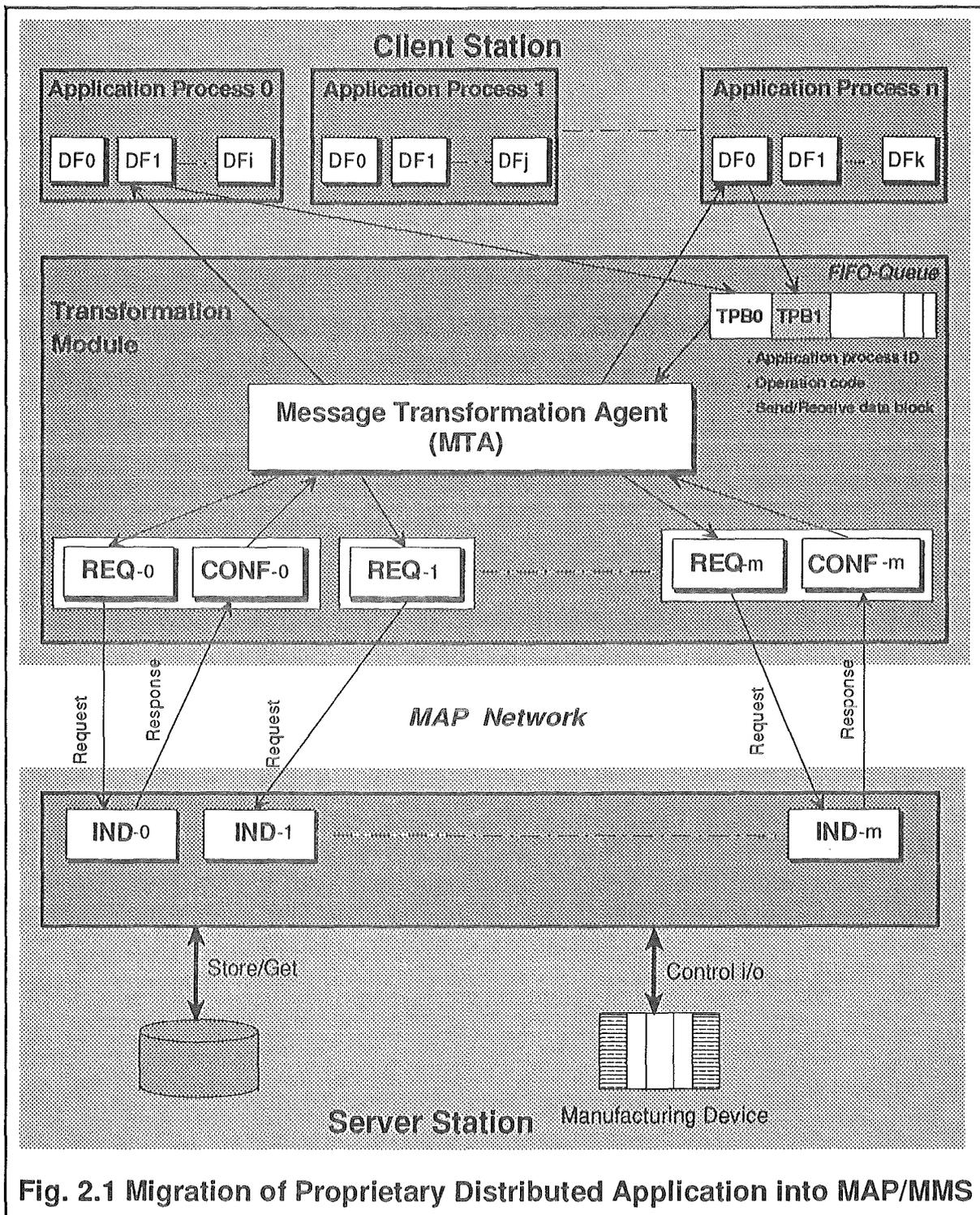
Fig. 2.1 Migration of Proprietary Distributed Application into MAP/MMS
