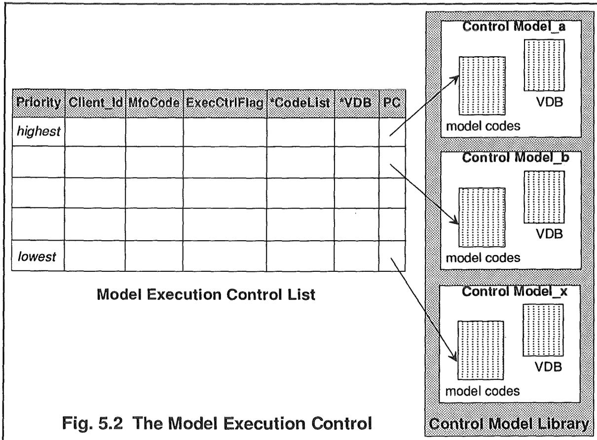
By use of the *Model Execution Control List*, the Transformation Agent can process a number of Control Models concurrently. It is able to deal with several CIM-OSA models in a quasi parallel way. The Transformation Agent interprets each instruction of a Control Model and takes the corresponding actions. As soon as the Transformation Agent has completed a service request, it will change the state of the associated *Abstract Object Instance* (cf. Section 6.3).
