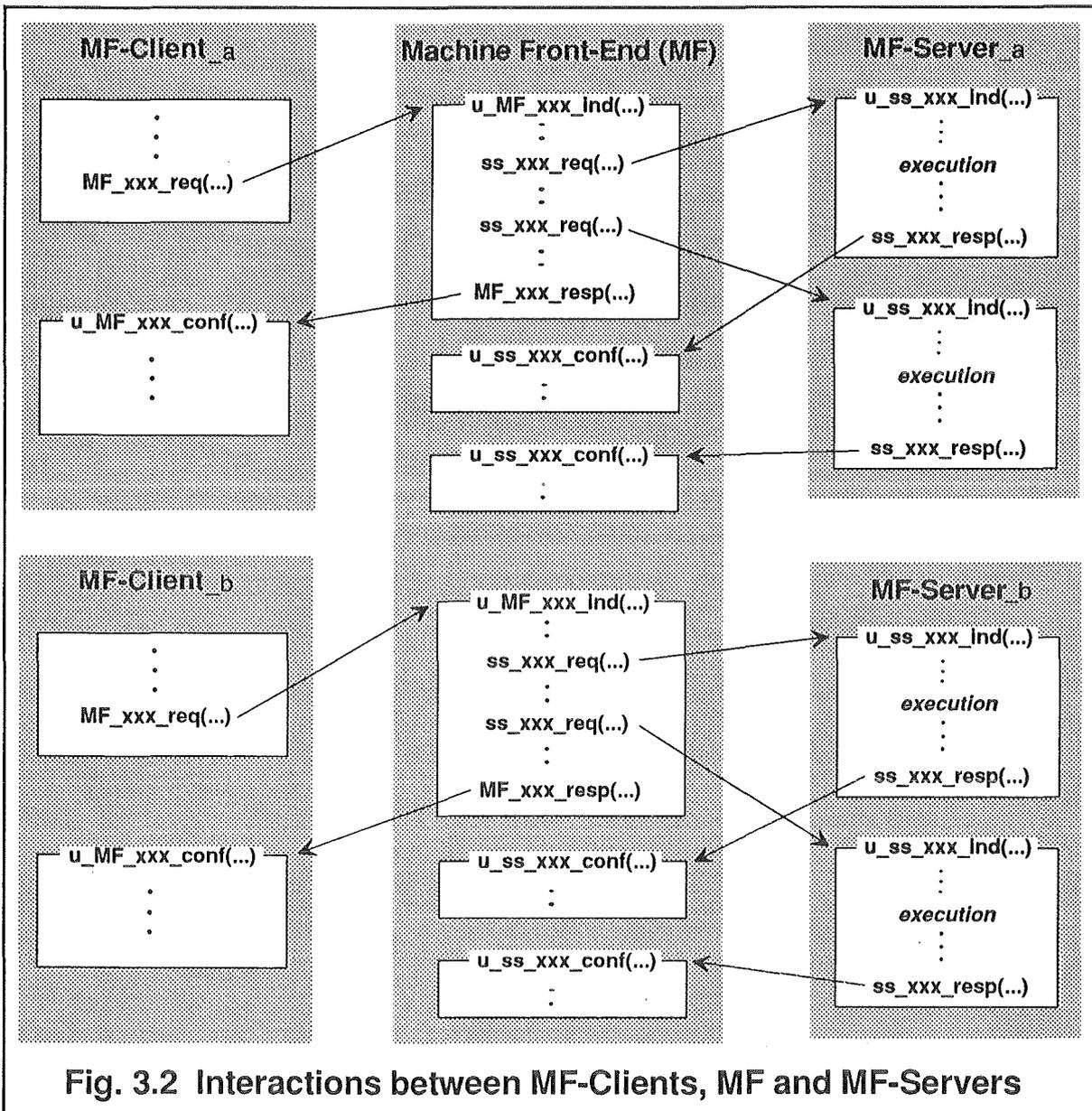
Fig. 3.2 Interactions between MF-Clients, MF and MF-Servers
