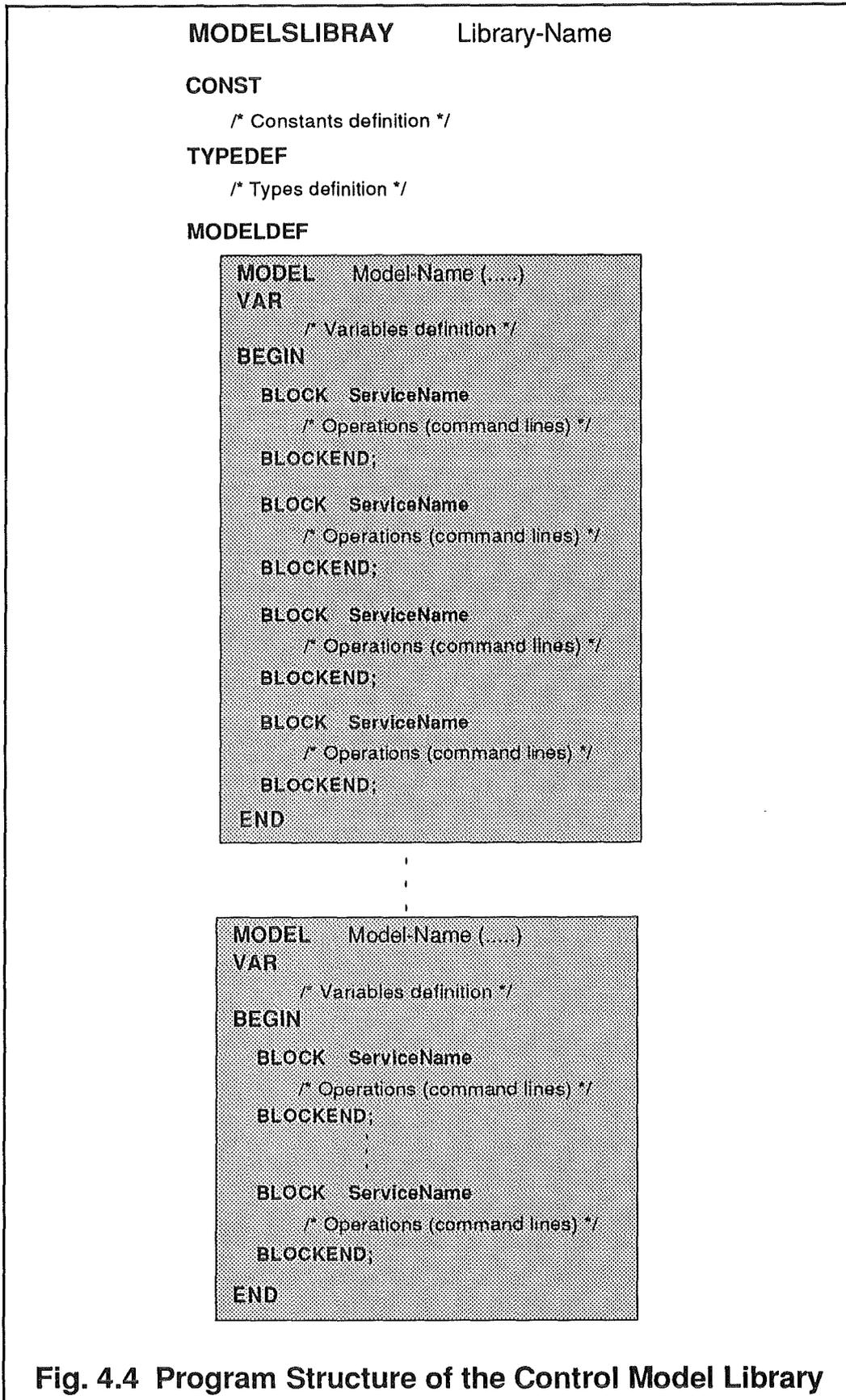
Fig. 4.4 Program Structure of the Control Model Library
