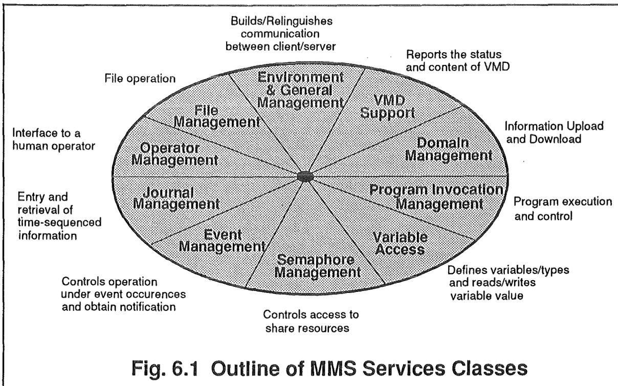
In MMS, services which are used to manipulate a MMS object are defined on the basis of the *Object State Transition Diagram*. Each service is described in a tabular form with their arguments and results.
