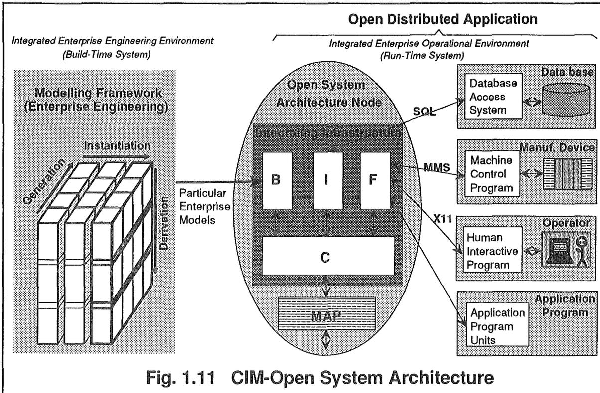
Fig. 1.11 CIM-Open System Architecture
