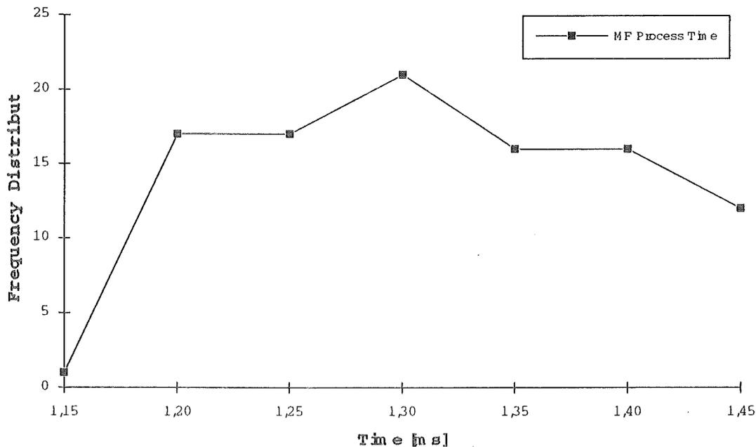
**Fig. 7.7 Frequency Distribution of the MF Process Time**
