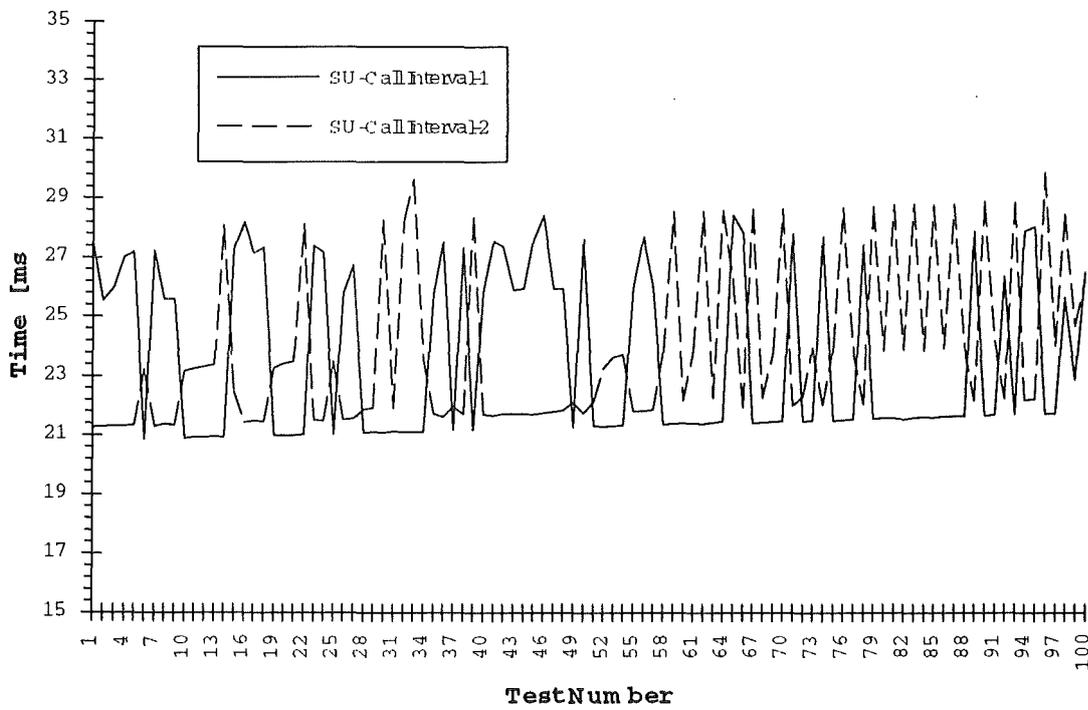
Fig. 7.9 Interval of the Service Unit Calls (with 3 MFO's)
