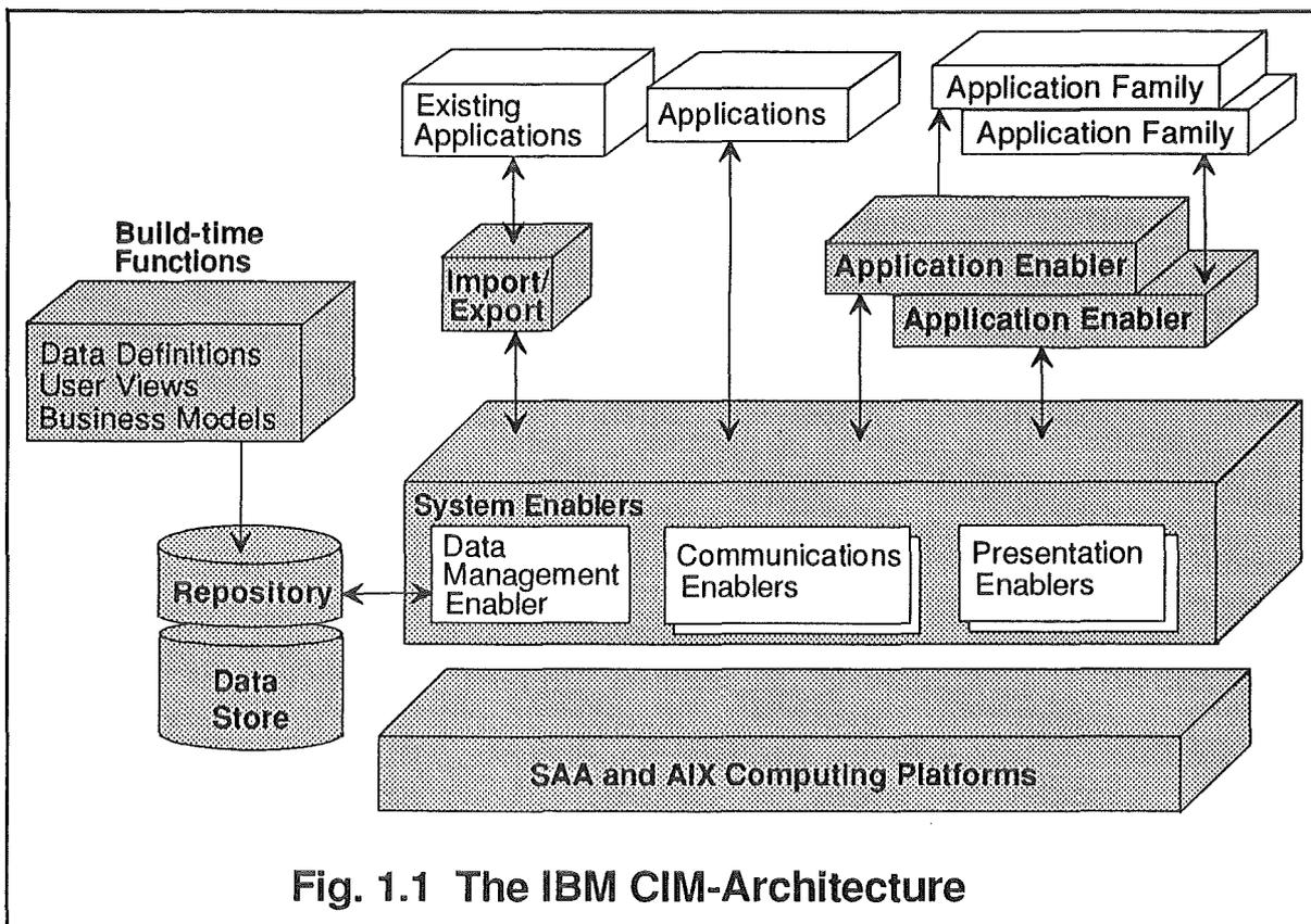
The IBM CIM-Architecture functions will be implemented on the operating environments of *IBM's Systems Application Architecture (SAA)* and *IBM's Advanced Interactive Executive (AIX)*. SAA is for consistency and compatibility among software products and AIX is for the UNIX environment.
