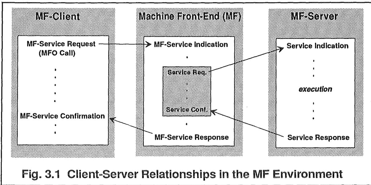
The Machine Front-End acts as an agent between the service requestor (MF-Client) and the service executor (MF-Server). After receiving a MFO call, it generates corresponding service request(s) and sends them to the appropriate MF-Server.
