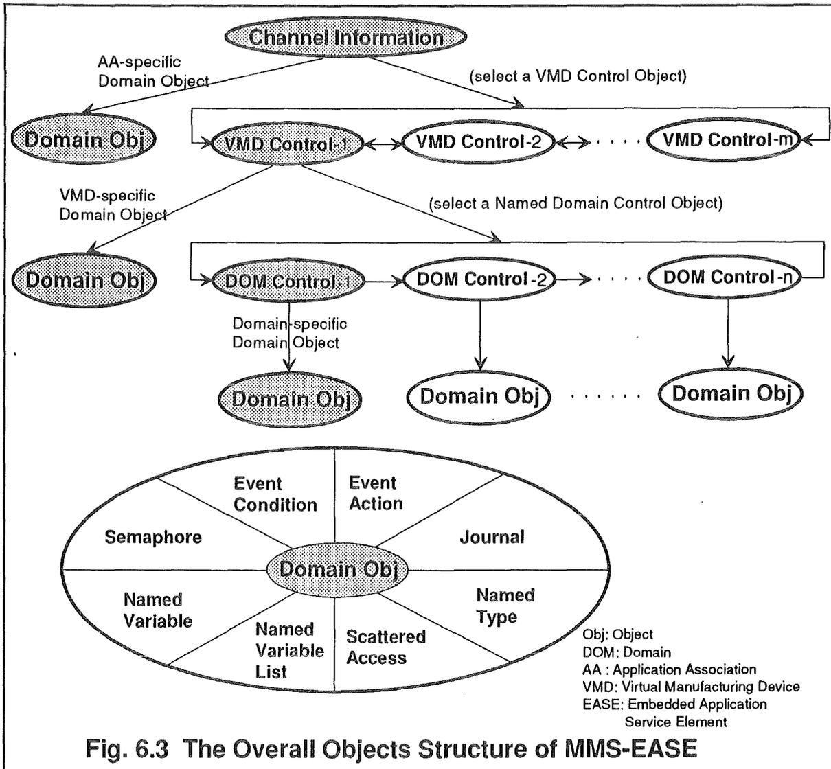
In MMS-EASE, a *VMD Control Object* (VMD Control) is used to represent a VMD. It is linked with its preceding and succeeding *VMD Control Objects*. This means that several VMD's can be established for a server application. This object contains the VMD-specific information: a VMD-specific Domain Object, pointers to the Domain, Program Invocation, Operator Station and Named Domain Control object, etc.
