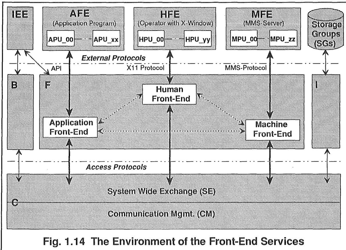
**Fig. 1.14 The Environment of the Front-End Services**
