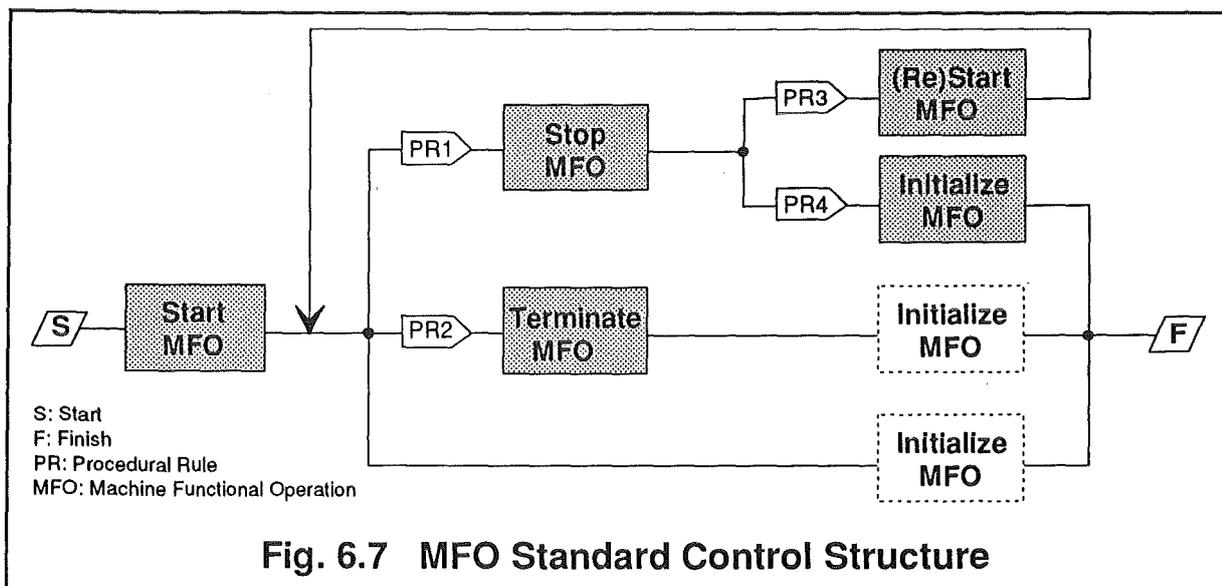
The action in the dotted blank box indicates that the service is not issued by the Activity Control. Internally, it is automatically triggered by the Machine Front-End. For example, after a *Start MFO Service Request* issued by the Activity Control has been successfully executed, the Machine Front-End should itself execute the *Initialize* service block of the Control Model, not because of an *Initialize MFO Service Request* issued by the Activity Control.
