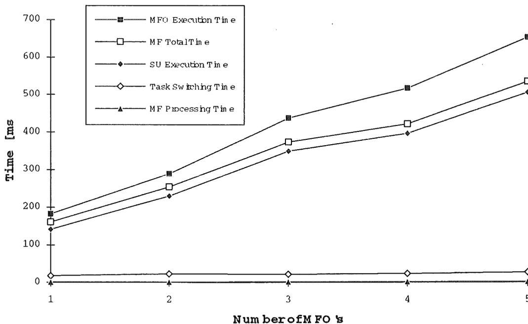
Fig. 7.10 Execution Times with Multiple MFO's
