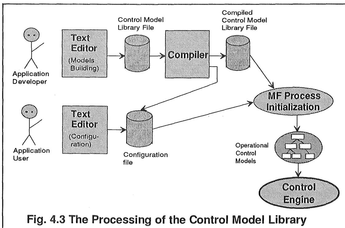
Fig. 4.3 The Processing of the Control Model Library
