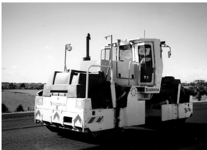
Fig. 4-14. The compactor used for the CIRCUM and MultiCIRCUM full-scale trials.
