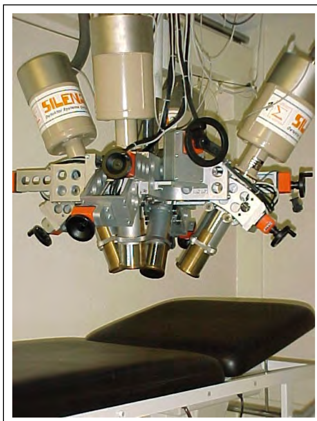
Figure 2.3.6 The HPGe detecting system for direct measurements of body activity available at the Forschungszentrum Karlsruhe.
