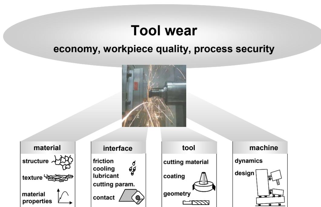
Fig. 1.7 Influencing elements of tool wear [Söhn-01b]
