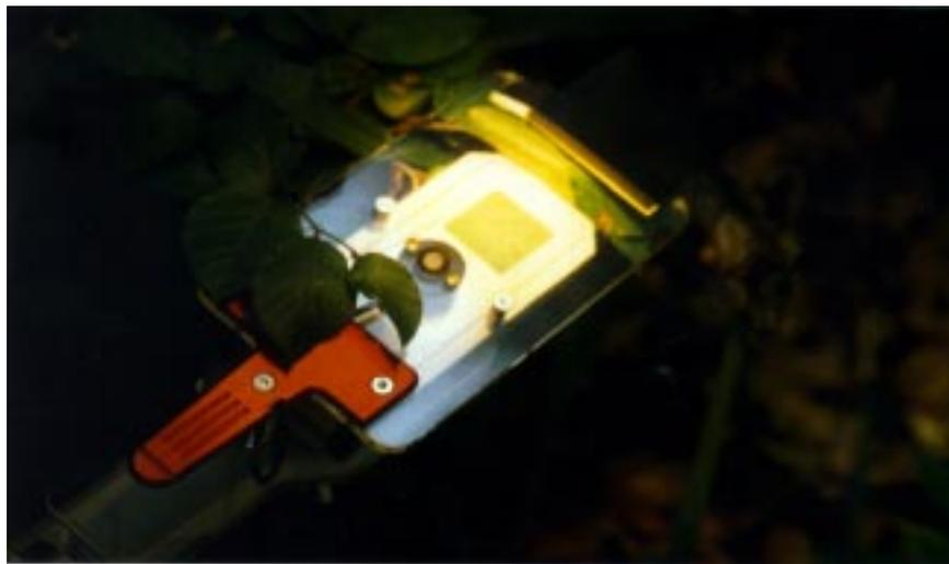
**Abb. 2.18:** Meßkopf des LCA-4-Porometers.
